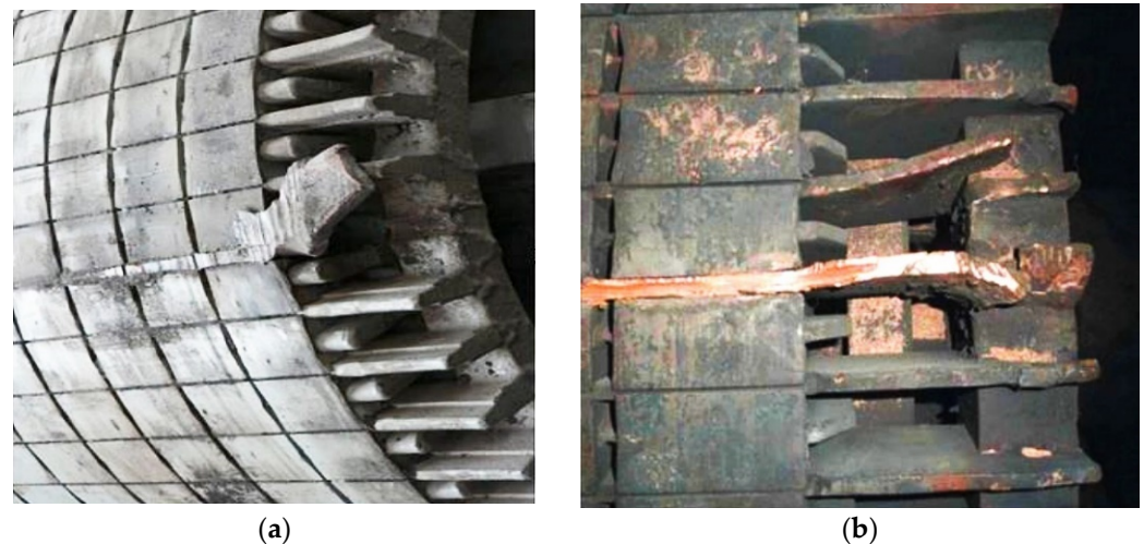
Figure 2. Damage to the rotor winding: (a) cast winding; (b) welded winding.
