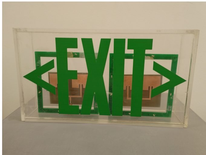
(a) Two harvesting circuits inserted inside the emergency sign box.
