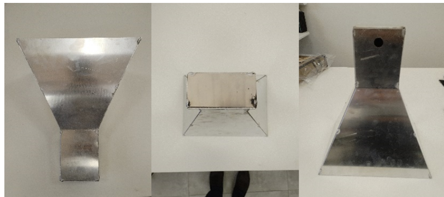
(b) Horn antenna made by welding aluminum sheets of 2 mm in thickness.
