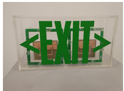
(b) Prepared circuit placed in the emergency exit sign.
