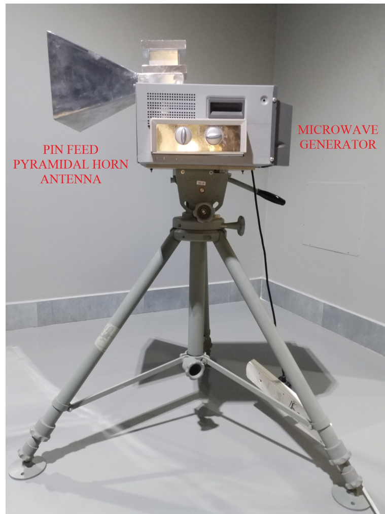
Figure 5. The microwave transmitter (0.5 kW).
