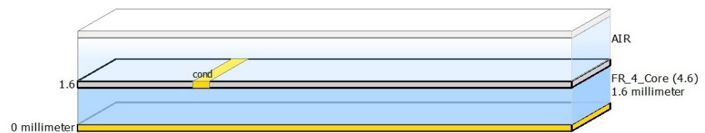
(a) Dimensions of the twin-patch antenna.
