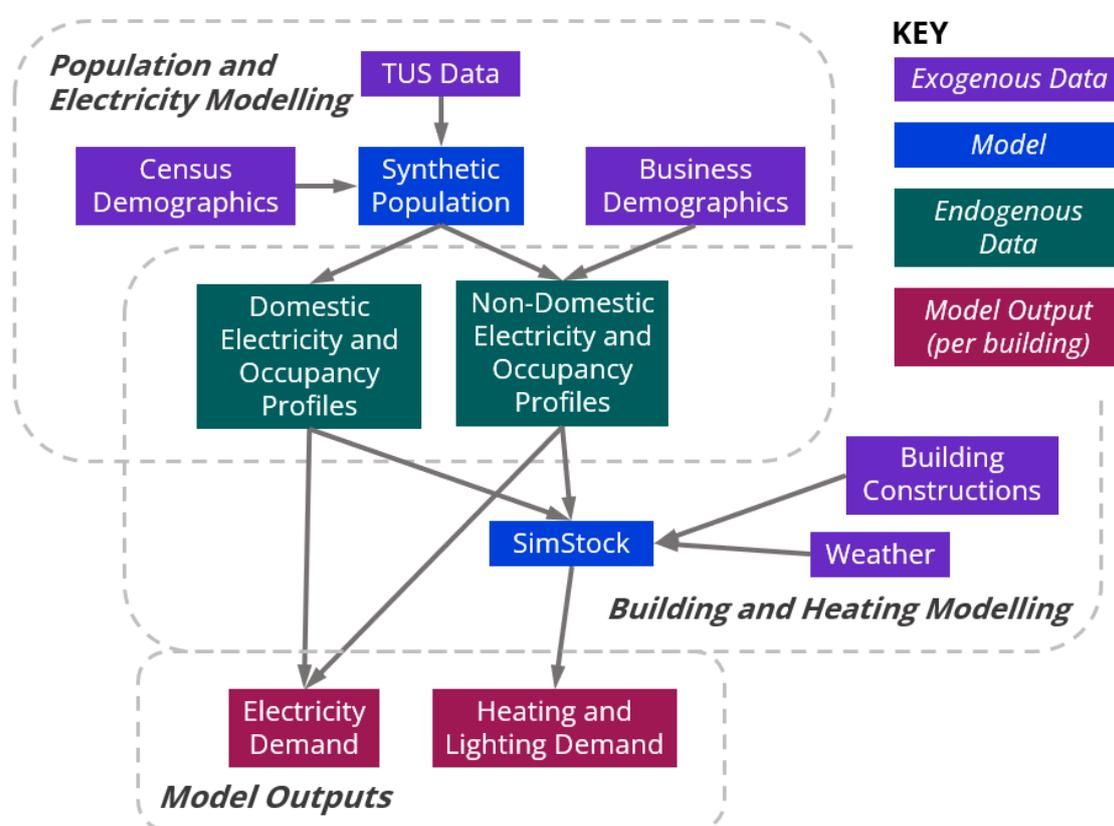
Figure 1. High-level flow chart of the modelling process.
