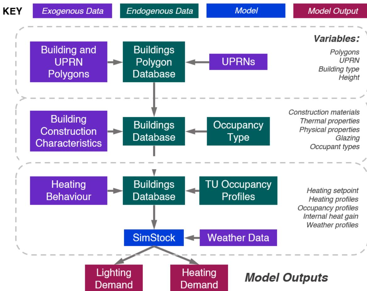
**Figure 6.** Workflow of the heating and lighting model using SimStock.
