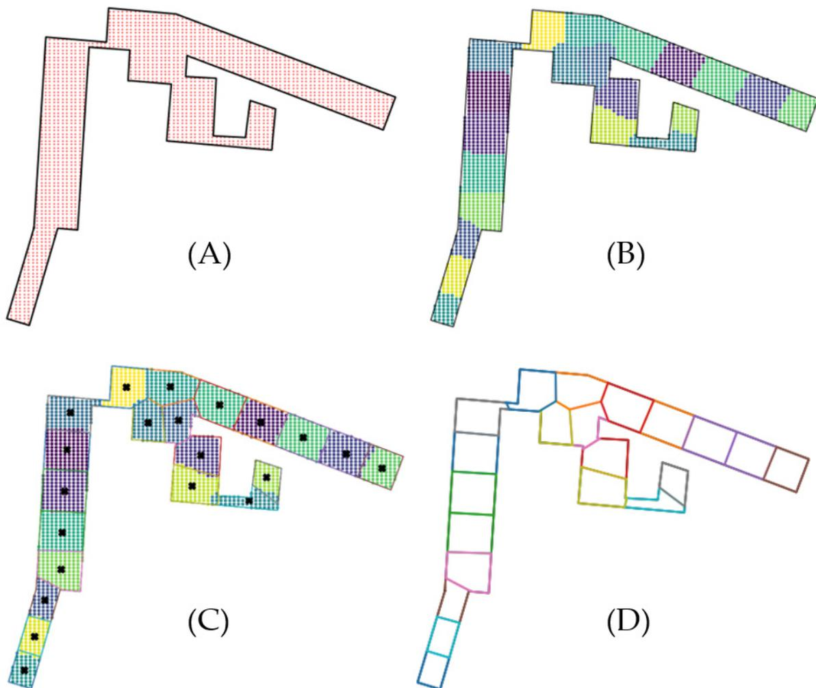
**Figure 7.** The polygon splitting process: (A) points assigned to a grid over the polygon; (B) spectral clustering groups for the number of building UPRNs; (C) centroids used to generate Voronoi diagrams; (D) intersection of Voronoi vertices generates new polygons for each UPRN.
