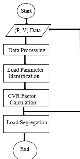
Figure 3. Flow chart of CVR calculation.
