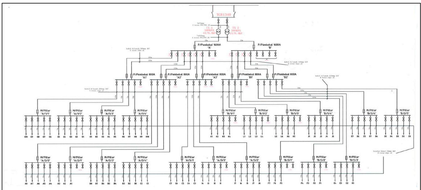
Figure 2. Single line diagram for a residential substation.
