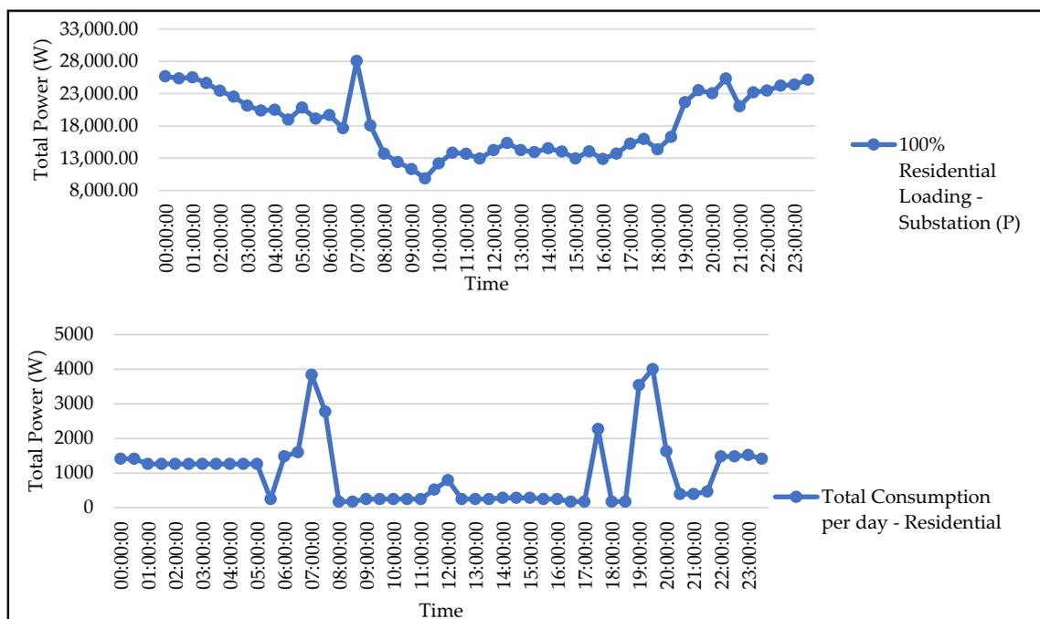
**Figure 10.** Substation and residence power consumption pattern.
