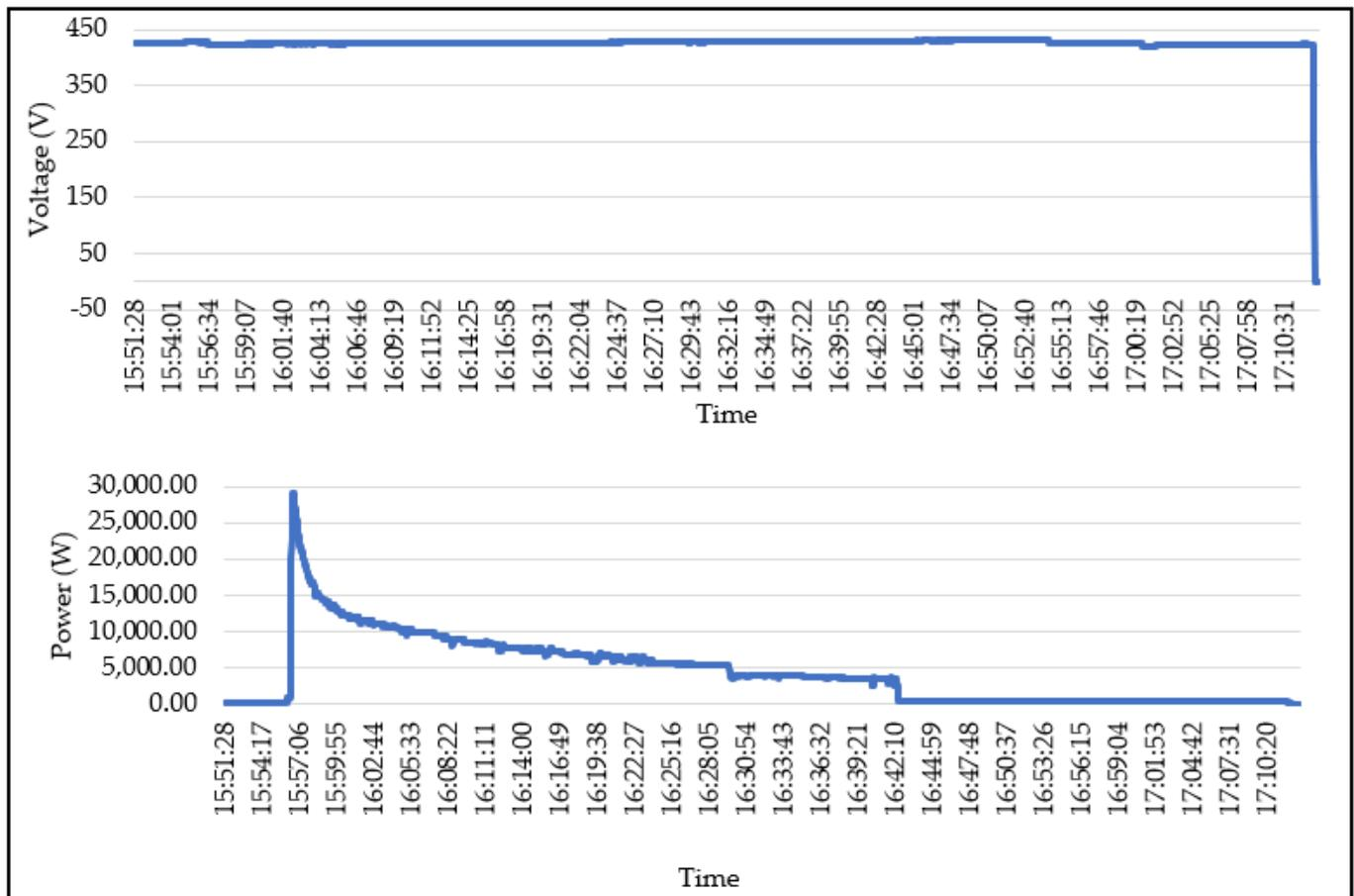
Figure 12. Voltage and Power Graph for EV Fast Charging (Chademo).
