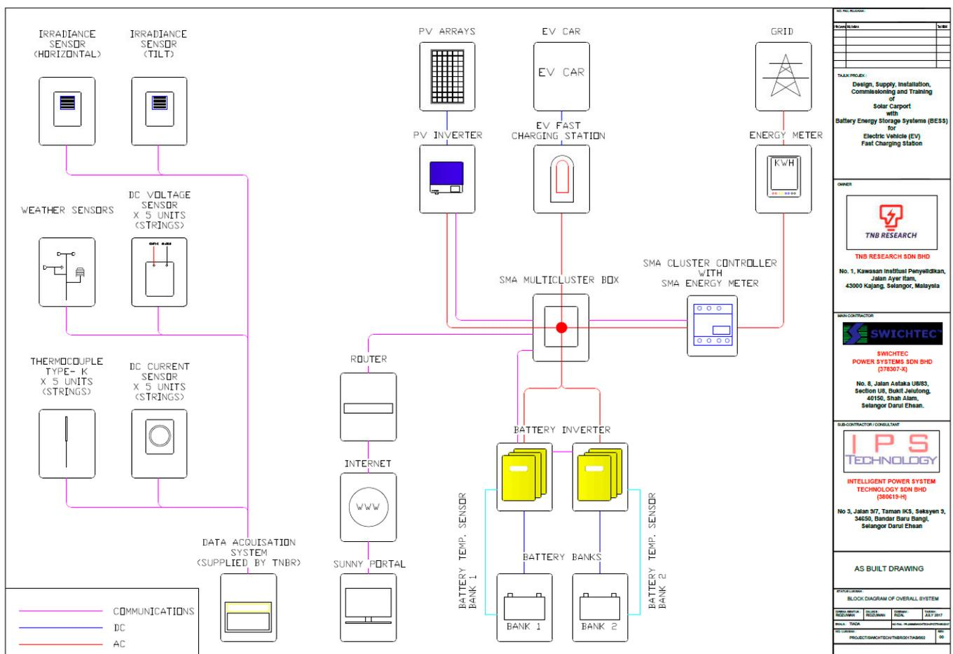
Figure 11. Schematic block diagram of the EV (Courtesy of the TNBR Environment Group).
