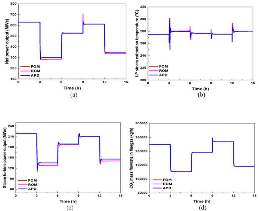
**Figure 4.** Comparison between APD/FOM/ROM: (a) net power output; (b) LP steam extraction temperature; (c) steam turbine output; and (d) CO<sub>2</sub> mass flowrate in flue gas.
