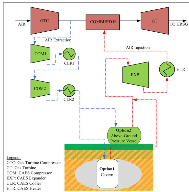
**Figure 1.** Schematic representation of CAES system integrated with NGCC plant.
