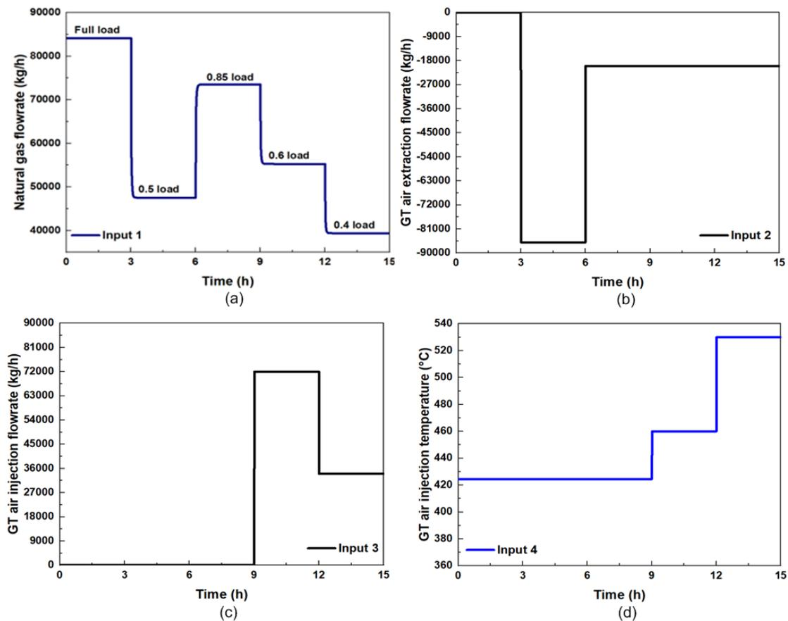
**Figure 3.** Simulated inputs for testing the ROM performance: (a) natural gas flowrate, (b) air extraction flowrate, (c) air injection flowrate, and (d) air injection temperature.
