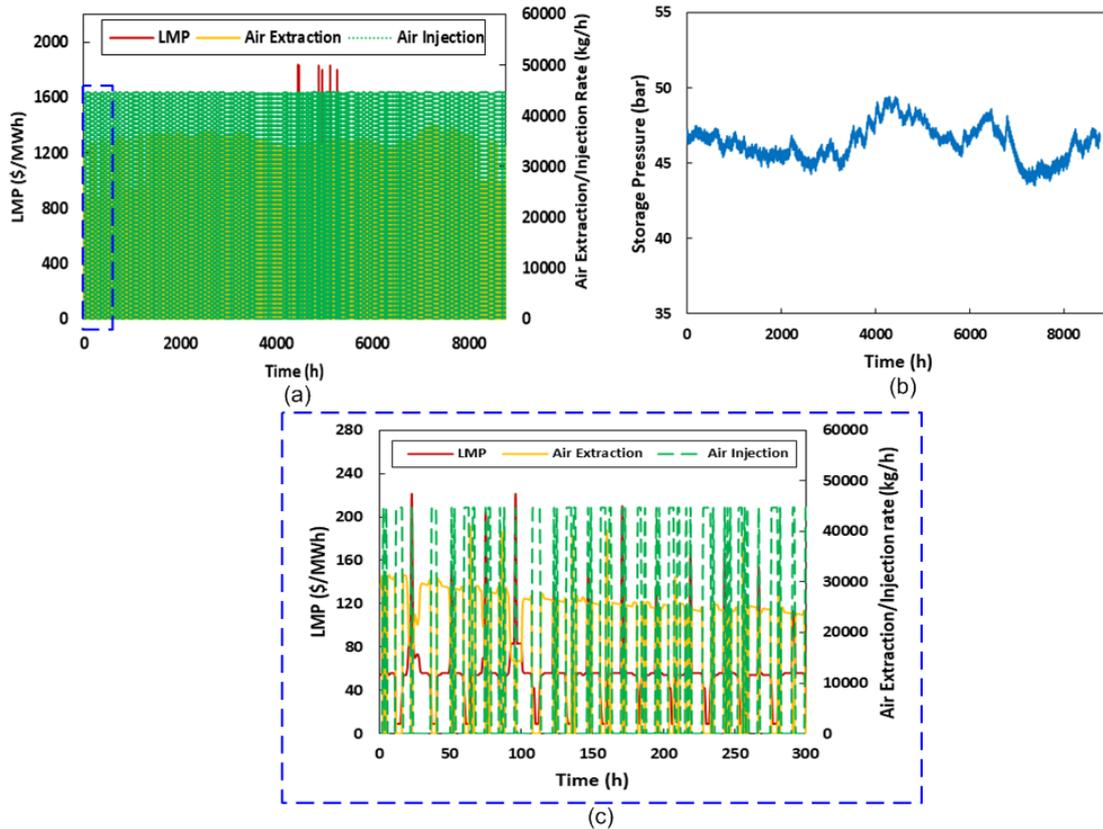
**Figure 7.** Optimization results for Princeton Base Case\_60 region: (a) air extraction and injection profile, (b) cavern storage pressure profile, and (c) zoomed view of air extraction and injection profile.
