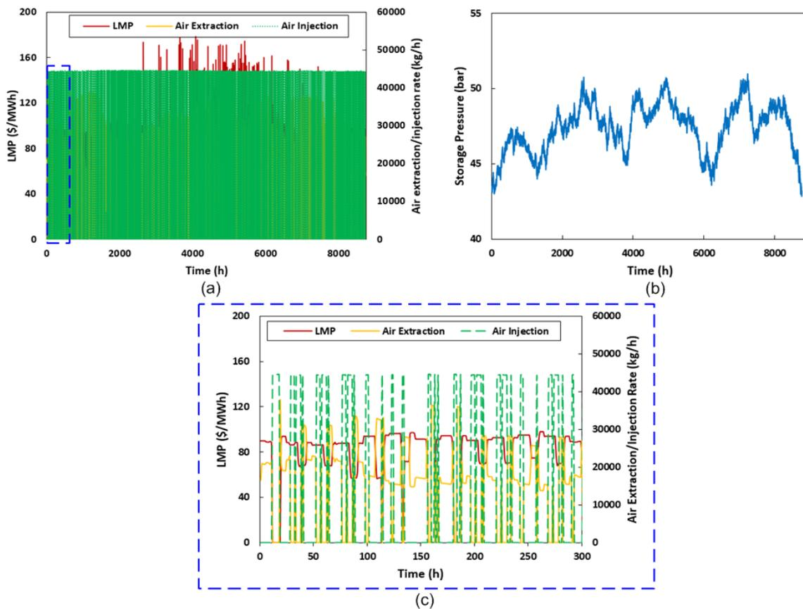
**Figure 6.** Optimization results for CAISO\_100 region: (a) air extraction and injection profile, (b) cavern storage pressure profile, and (c) zoomed view of air extraction and injection profile.
