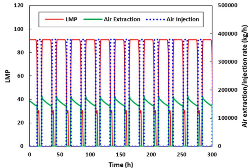
**Figure 8.** Air extraction and injection profile for a specific LMP.
