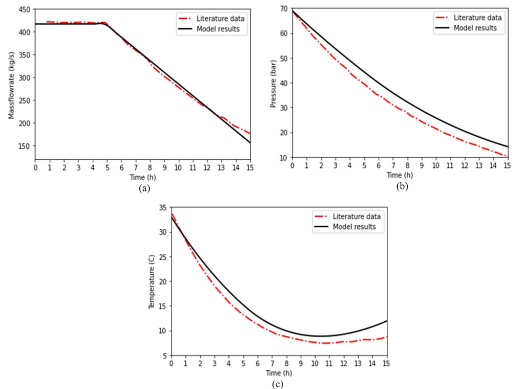
**Figure 2.** Model validation results: (a) dynamics of mass flowrate; (b) pressure change in the cavern; and (c) temperature change in the cavern.
