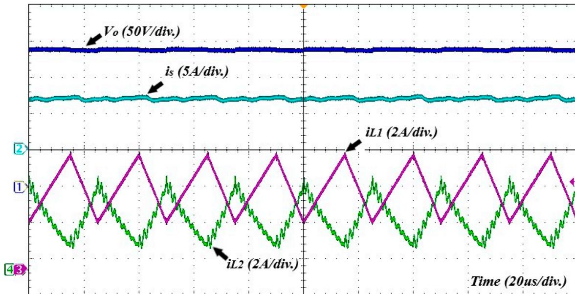
**Figure 15.** Open-loop waveforms. From top to bottom: output voltage  $V_o$  (blue trace), input current  $i_s$  (cyan trace), inductor current  $i_{L1}$  (magenta trace), and inductor current  $i_{L2}$  (green trace); test at  $D = 0.6$ .
