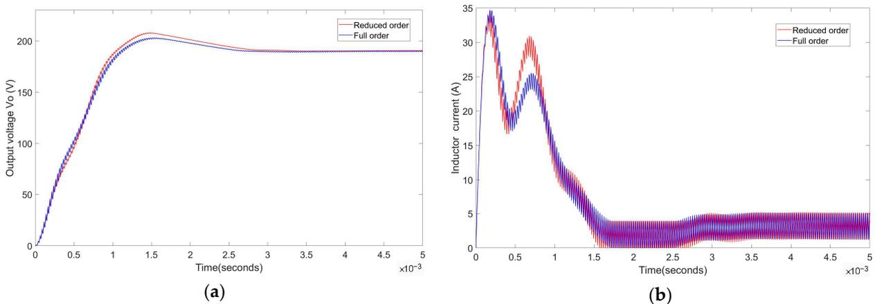
**Figure 7.** Comparison between the reduced-order model and the full-order model: (a) output voltage; (b) current of  $L_2$ .
