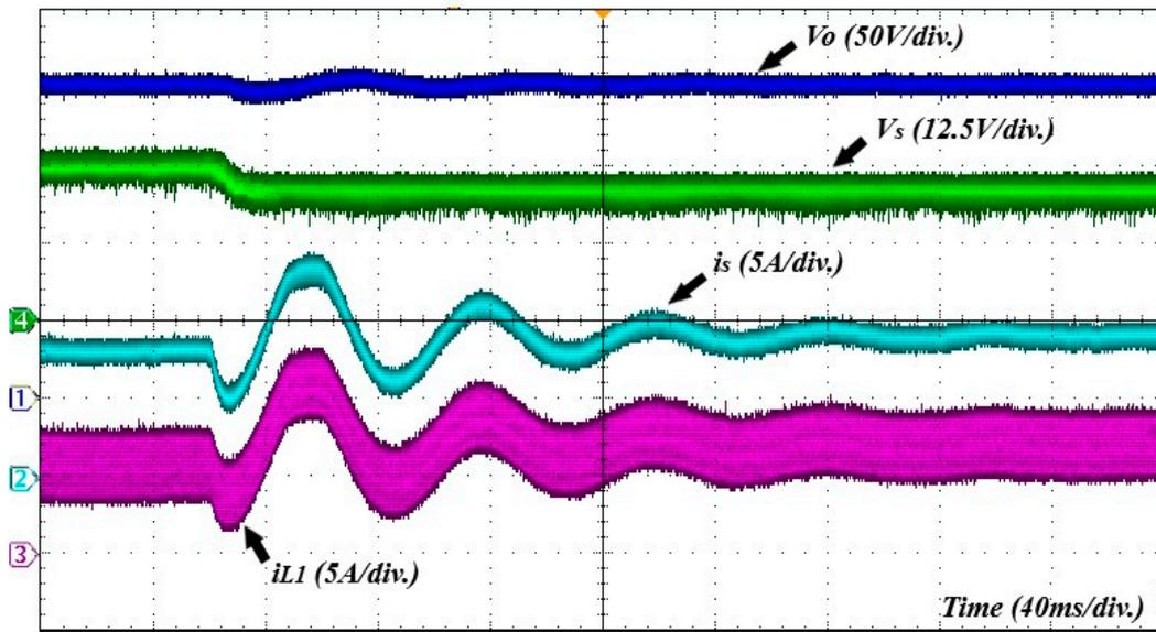
Figure 17. Transient response under input voltage change. From top to bottom: output voltage  $V_o$  (blue trace), input voltage  $V_s$  (green trace), input current  $i_s$  (cyan trace), and inductor current  $i_{L1}$  (magenta trace).
