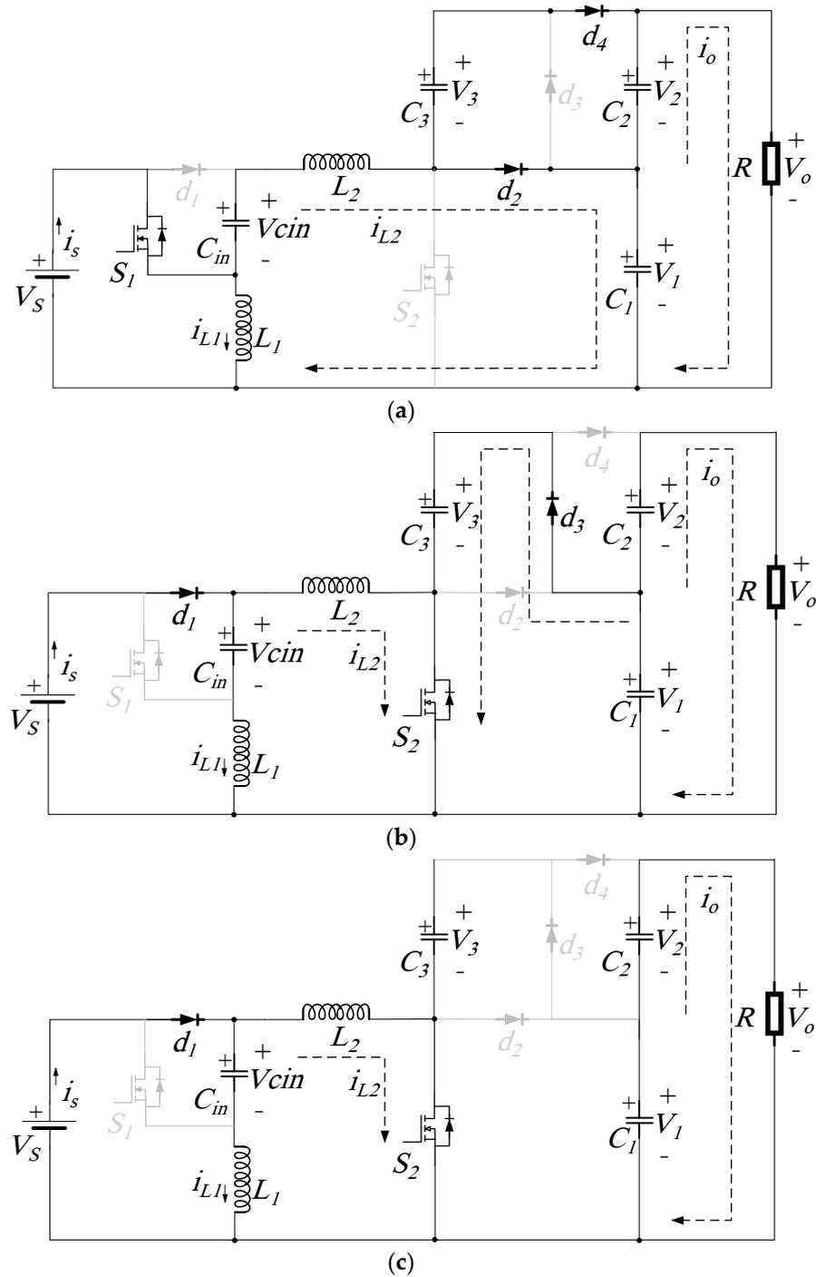
Figure 3. Operating modes during a switching period: (a) Mode I; (b) Mode II; (c) Mode III.
