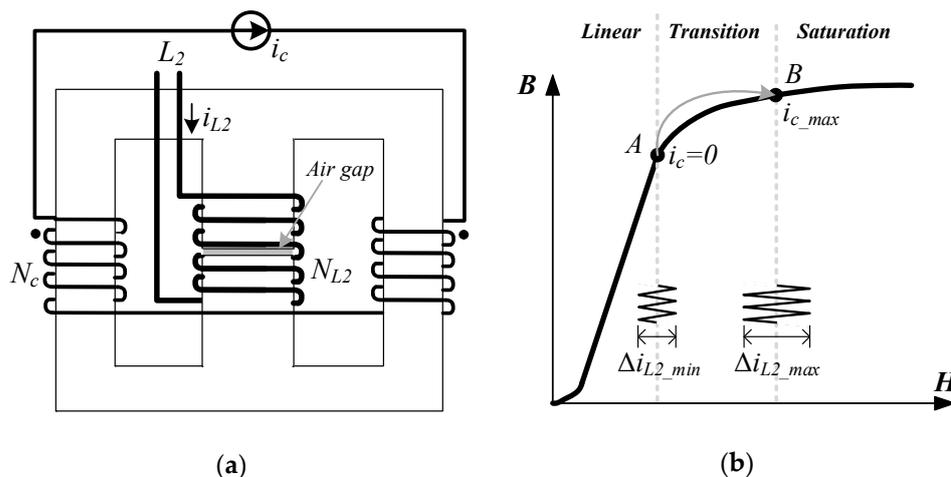
Figure 4. VI structure [18]: (a) winding distribution; (b) operating points on the B–H curve. Point A represents the limit of the linear region, and point B represents the limit of the transition region.
