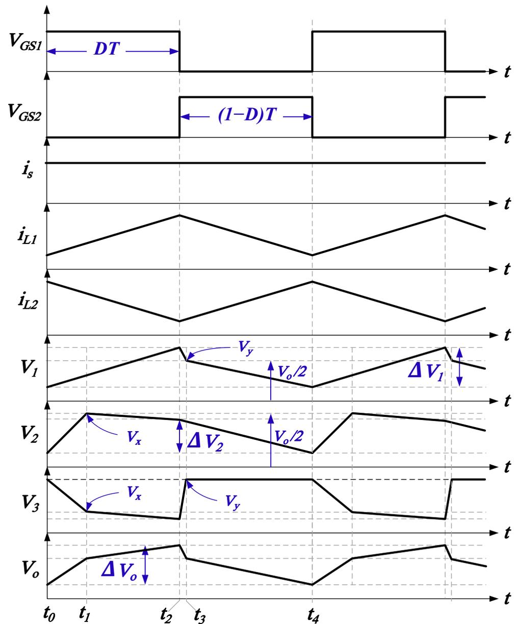
Figure 2. Steady-state waveforms of the main converter.
