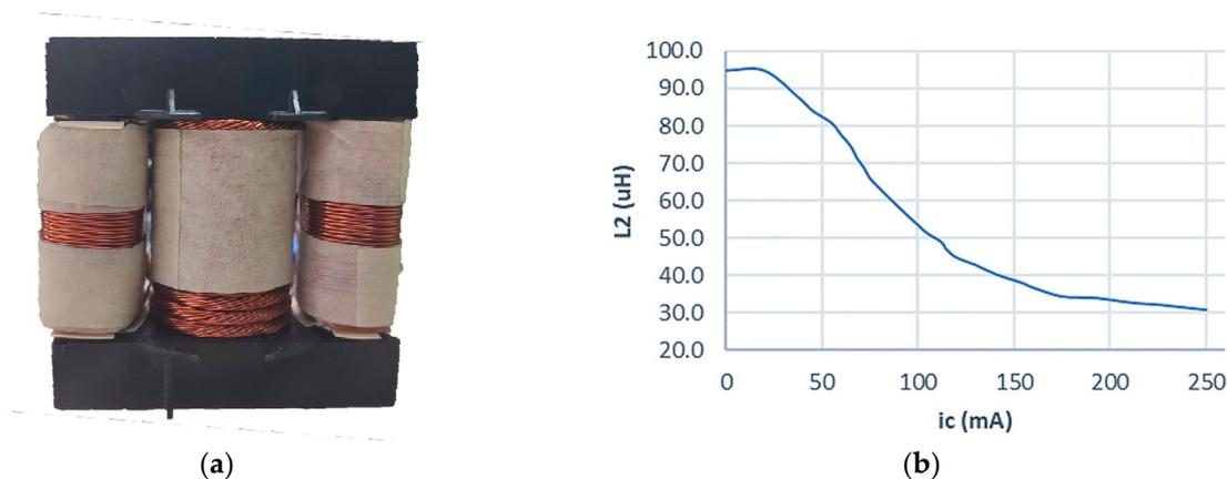
**Figure 14.** VI graphical representation: (a) prototype; (b) inductance curve.
