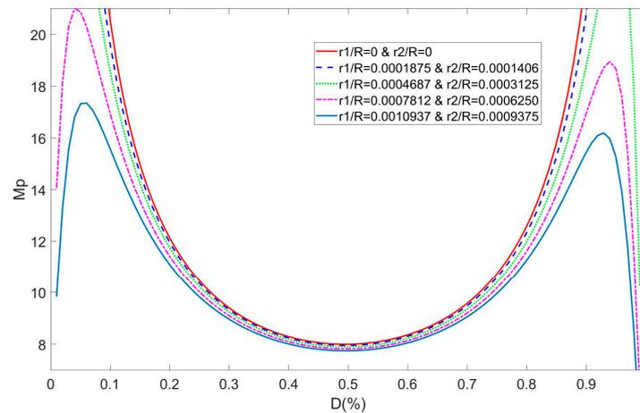
Figure 6. Voltage gain versus duty cycle considering ESR of inductors.
