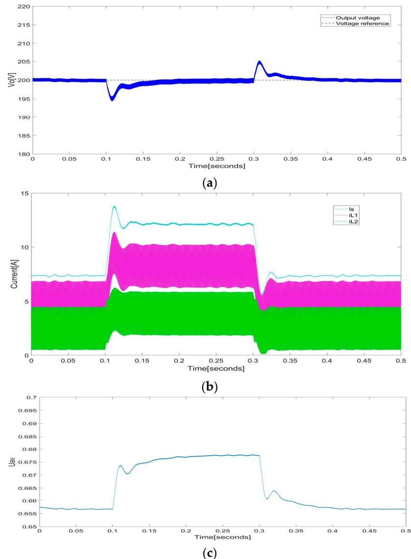
**Figure 11.** Simulated transient of the proposed DC-DC boost converter under a load step change from 60% to 100% and vice versa: (a) output voltage  $V_o$  (blue trace) and reference (dotted line); (b) from top to bottom: input current  $i_s$  (cyan trace), inductor current  $i_{L1}$  (magenta trace), and inductor current  $i_{L2}$  (green trace); (c) control law  $u_{av}$ .
