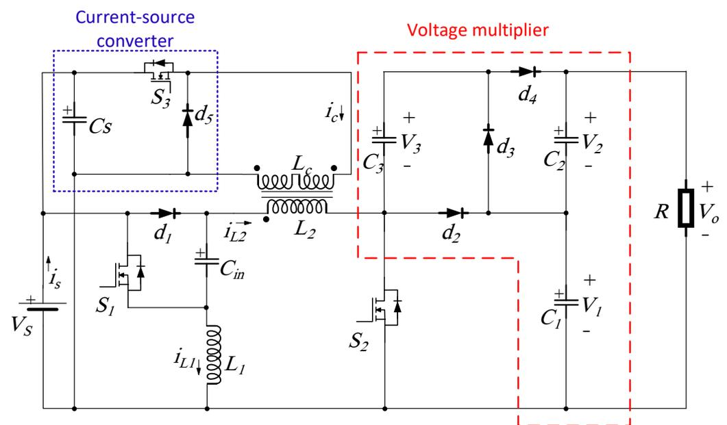
**Figure 1.** The schematic diagram of the proposed converter and its power stages.
