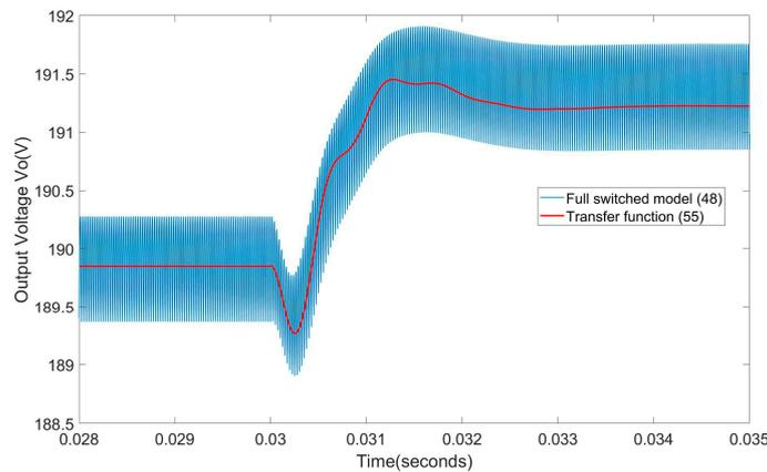
Figure 8. Comparison between the fully switched model and the transfer function  $G_u(s)$ .
