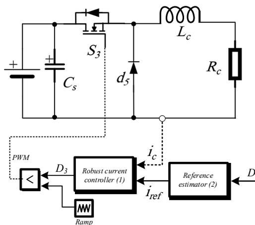
Figure 5. Schematic diagram of the power stage for the VI.
