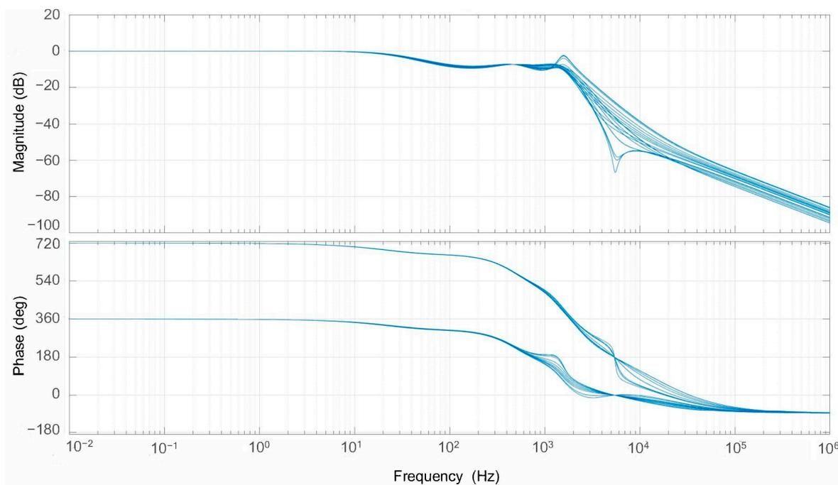
**Figure 10.** Bode diagram of closed-loop response. From top to bottom: magnitude diagram (top) and phase diagram (bottom).
