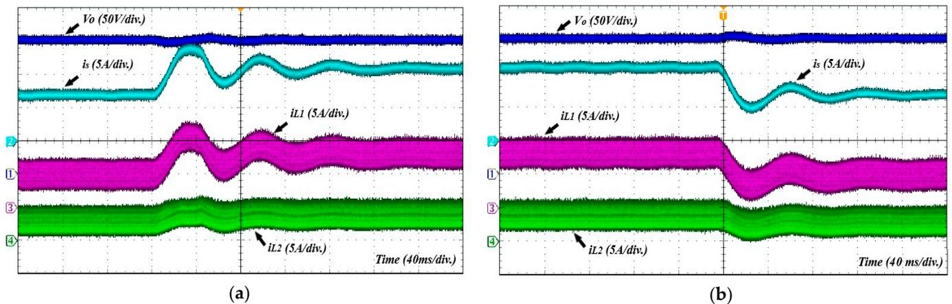
**Figure 16.** Transient response under load variation. From top to bottom: output voltage  $V_o$  (blue trace), input current  $i_s$  (cyan trace), inductor current  $i_{L1}$  (magenta trace), and inductor current  $i_{L2}$  (green trace): (a) from 60% to 100%; (b) from 100% to 60%.
