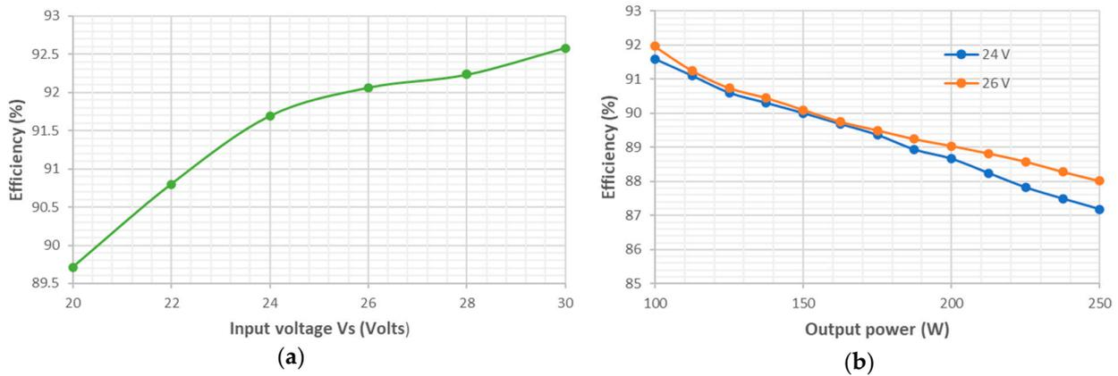
Figure 18. Efficiency test of the converter: (a) efficiency test for different input voltages; (b) efficiency test for different output loads.
