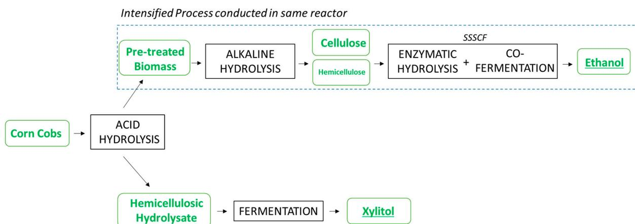
**Figure 1.** Flowchart outlining the experiments conducted for the valorization of corncobs in processes carried out in a column reactor for ethanol and xylitol production.
