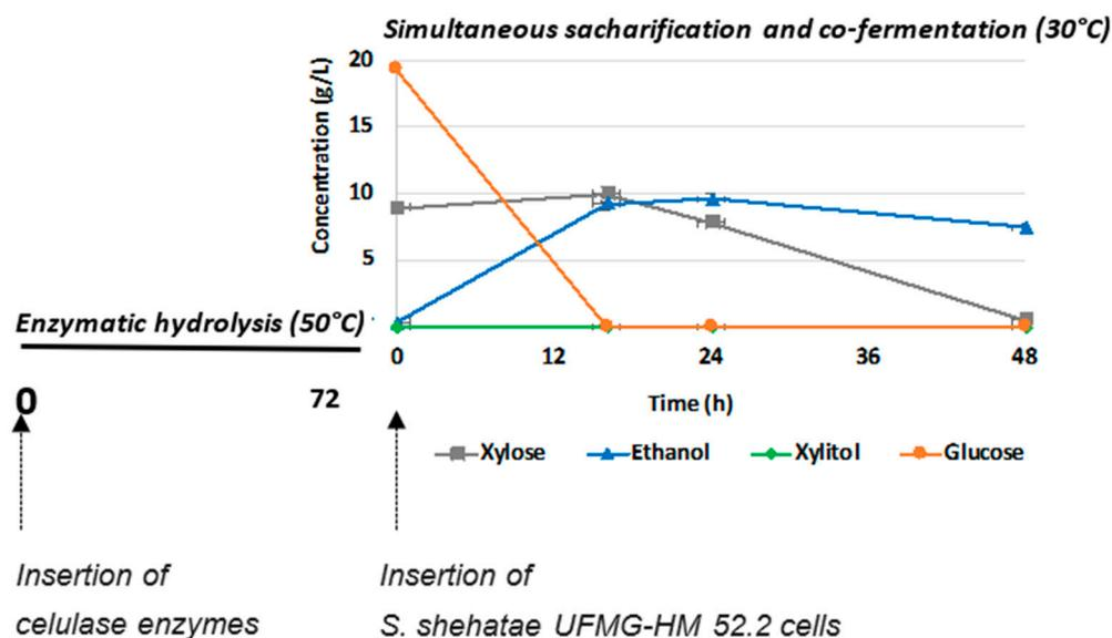
**Figure 7.** Ethanol production from corn cob enzymatic hydrolysate using *Scheffersomyces parashehatae* UFMG-HM 52.2 in column reactor operated as fluidized bed reactor.
