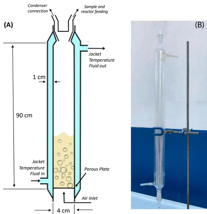
**Figure 2.** (A) Flowchart of the column reactor and (B) a photograph of the actual apparatus.
