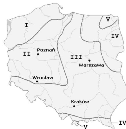
**Figure 2.** Climatic zones in Poland according to PN EN 12831 (Zone numbering in Table 2).
