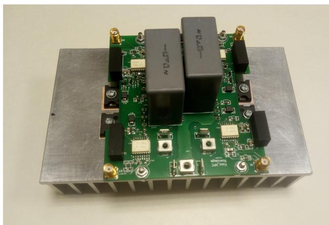
**Figure 6.** The laboratory setup of inverter with anti-parallel reverse-blocking transistors in the horizontal branch.
