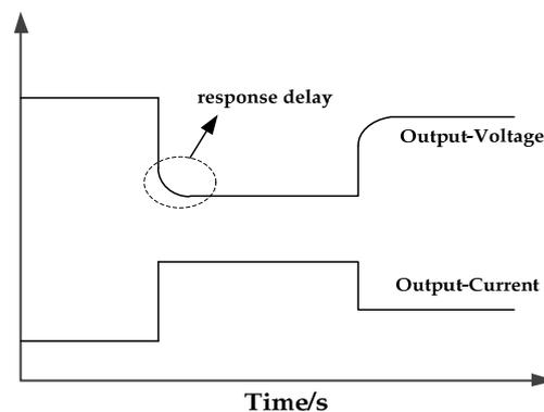
**Figure 5.** Dynamic response of fuel cell.
