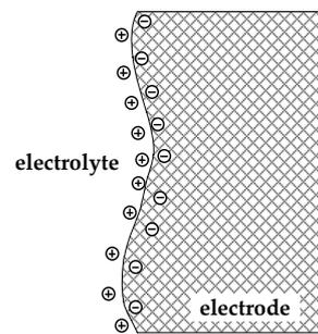
**Figure 4.** Capacitance effect at electrode interface.
