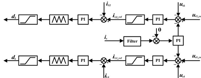
Figure 20. The control block diagram of the boost-type differential inverter.
