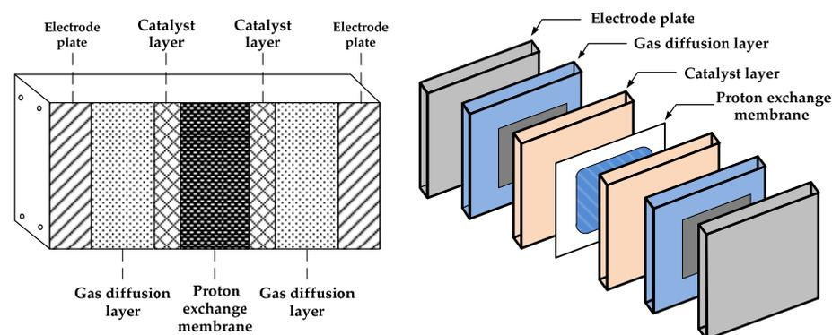
**Figure 2.** Structure diagram of PEMFC fuel cell.
