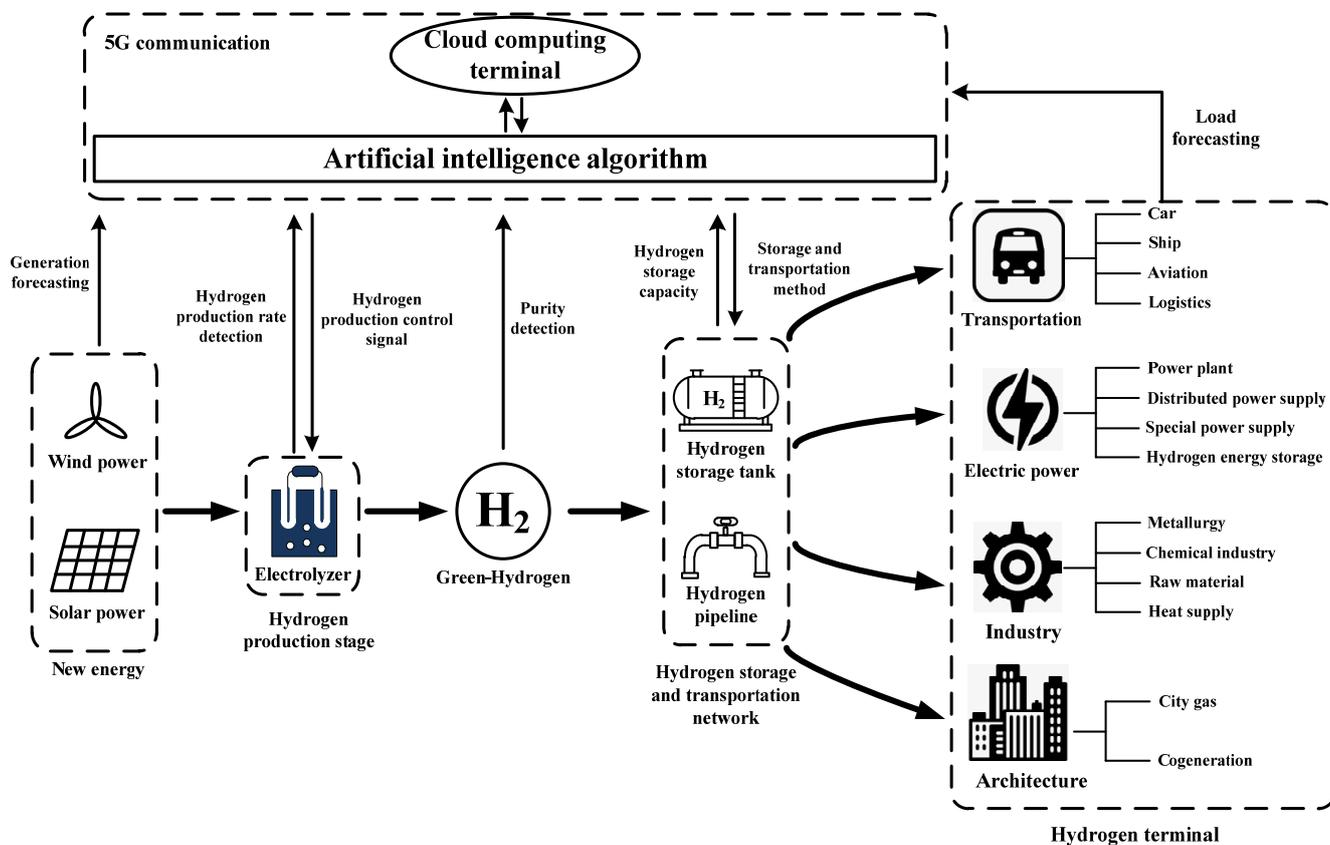
Figure 21. Schematic diagram of green hydrogen energy system.
