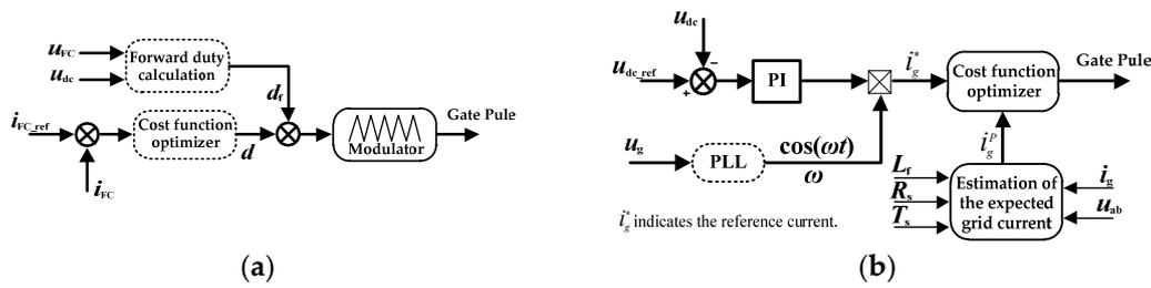
Figure 18. The control block diagram of Boost+ H6 converter.
