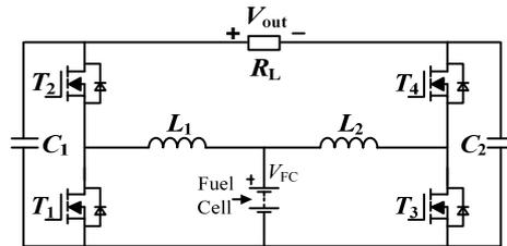
Figure 19. The boost-type differential inverter.
