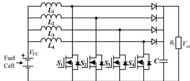
Figure 11. The four-phase interleaved DC/DC converter.
