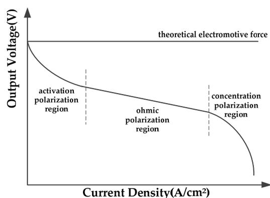
**Figure 3.** Volt-ampere characteristic curve fuel cell.
