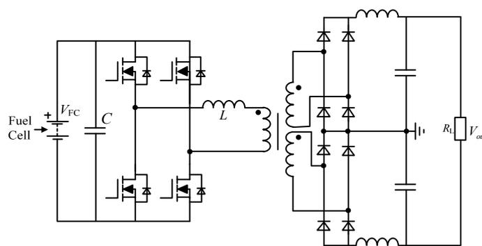
Figure 9. Phase-shifted full-bridge converter.
