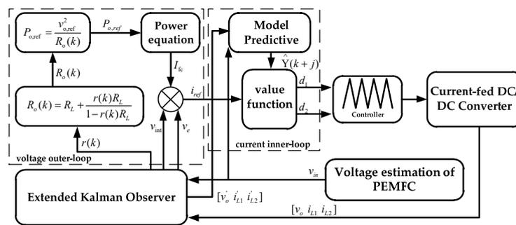
Figure 8. Control block diagram of Current-fed DC/DC Converter.
