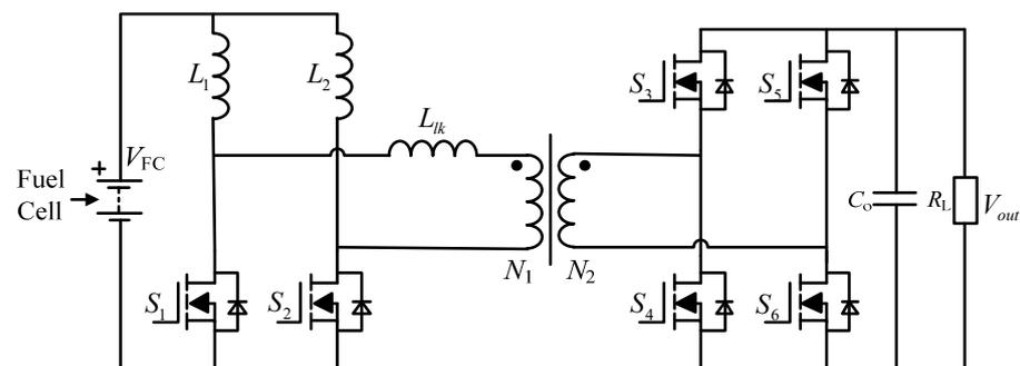
Figure 7. Current-fed DC/DC Converter.
