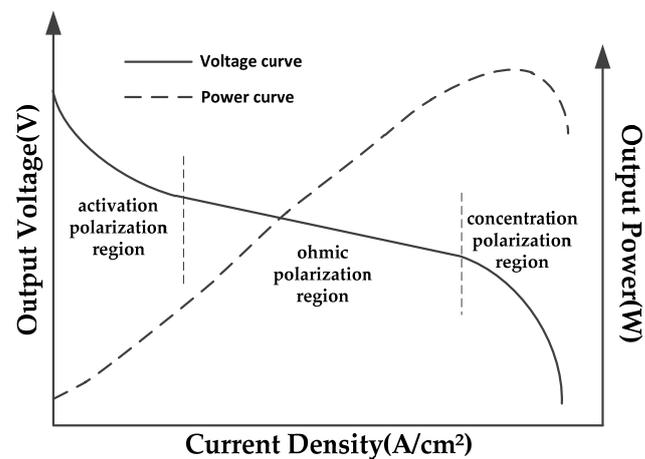
Figure 6.  $V$ - $I$  and  $P$ - $I$  characteristic curves of fuel cells.
