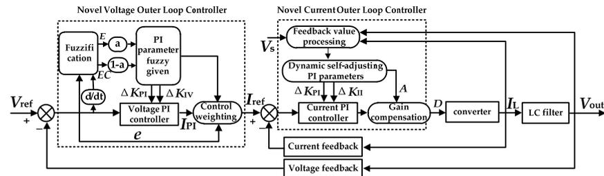
Figure 10. Novel double closed-loop controller's block diagram.
