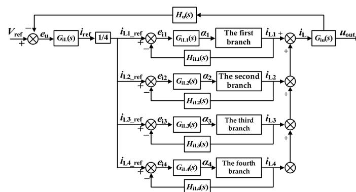
Figure 12. Control block diagram of four-phase interleaved converter.
