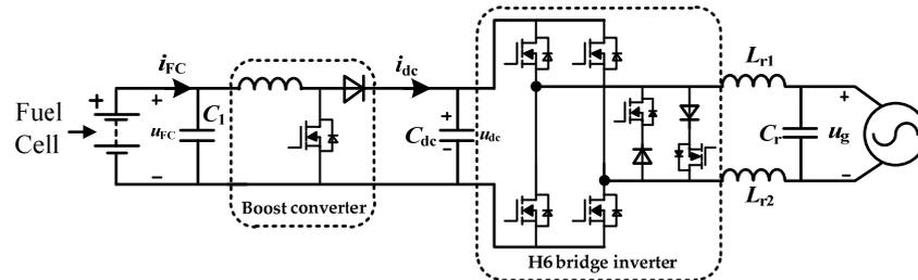
Figure 17. Circuits of single-phase grid-tied PEMFC system.
