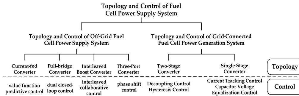
**Figure 1.** Classification of fuel cell power generation.
