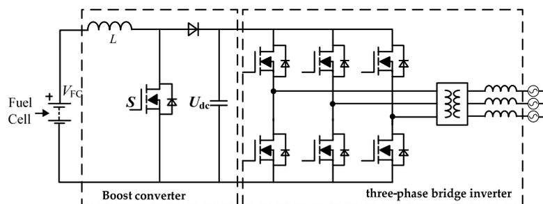
Figure 15. Boost+ three-phase bridge inverter topology.
