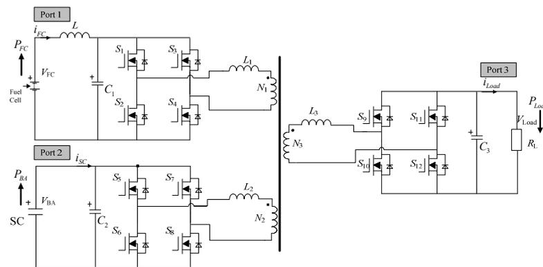
Figure 13. Three-port triple-active-bridge converter.
