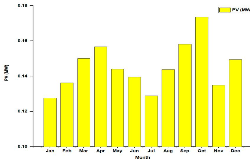
Figure 11. Monthly generated power from solar PV in Abha [63].
