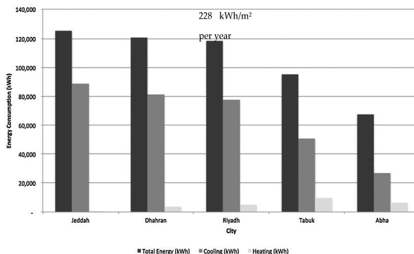
Figure 1. Total annual energy consumption, space cooling and space heating for a villa located in five cities [2].
