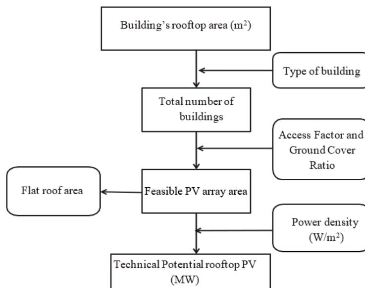
**Figure 10.** A methodology for determining the technical potential of rooftop solar PV installations in residential and commercial areas.
