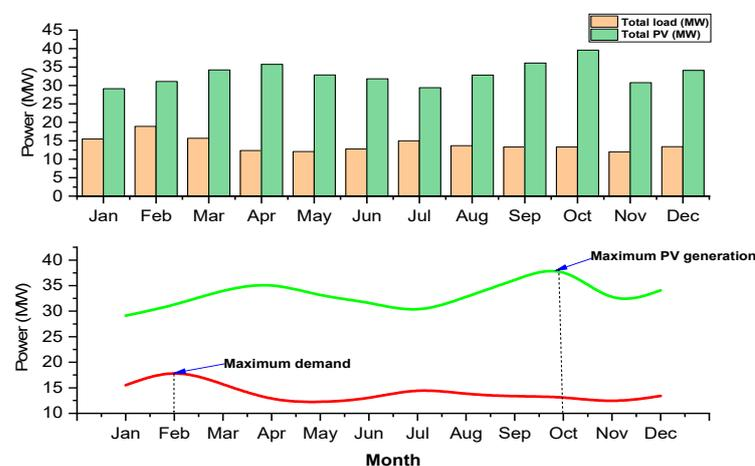
Figure 15. Residential load profile and PV production.
