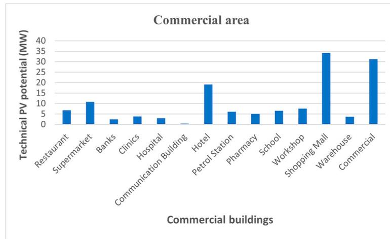
Figure 14. Technical rooftop PV potential for commercial buildings.
