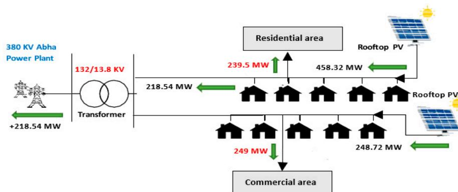
**Figure 18.** Abha case study network after connecting rooftop PV.
