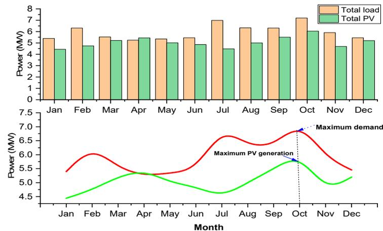
**Figure 16.** Service buildings load profiles and PV production.
