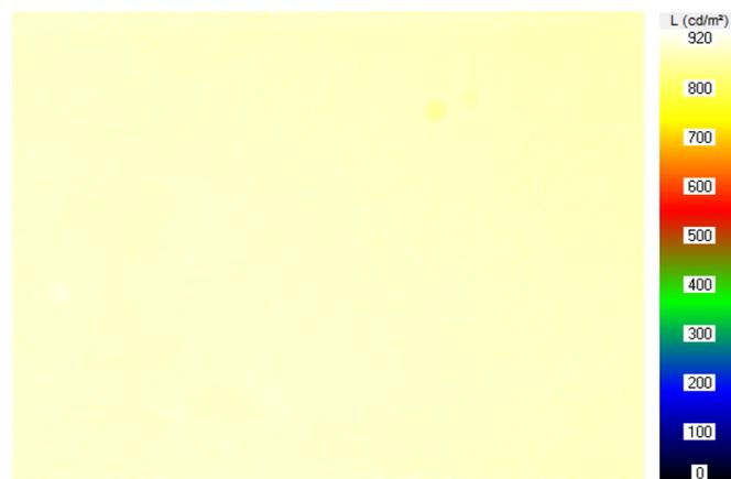
**Figure 3.** The view of the luminance distribution on the surface with reference luminance for 280 mm measurement distances (LMK 98-3 Color).
