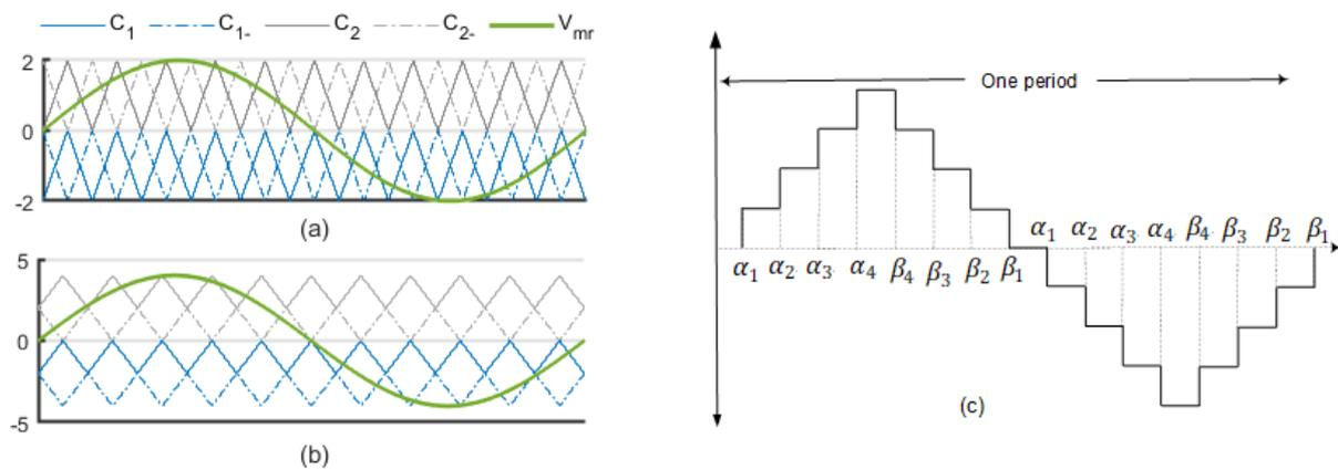
**Figure 12.** Various sub-techniques for LSC PWM scheme: (a) opposite-phase PWM for FB structure [106], (b) alternate opposite-phase PWM for FB structure [106], and (c) synthesized nine-level voltage waveform for SHE modulation [108].
