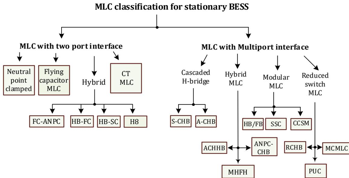
**Figure 2.** Categories of MLC configurations for stationary BESSs.
