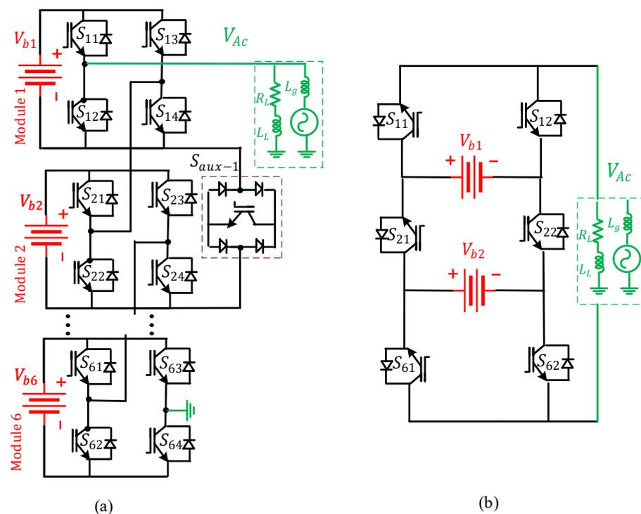
**Figure 7.** Schematic diagram of reduced-switch MLC for (a) modified cascaded CHB and (b) packed U-cell configuration.
