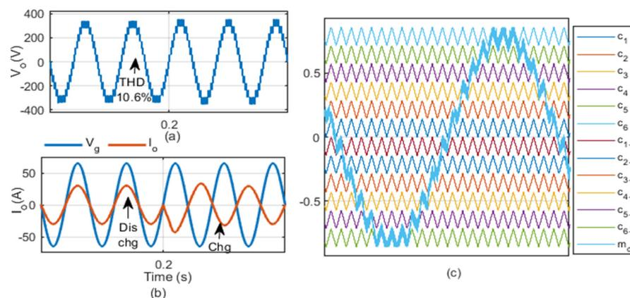
**Figure 20.** Simulation results for equal-phase LSC modulation: (a) MLC output voltage, (b) injected current and grid voltage, and (c) twelve carrier signals and modulating–reference signal from the high–level controller.
