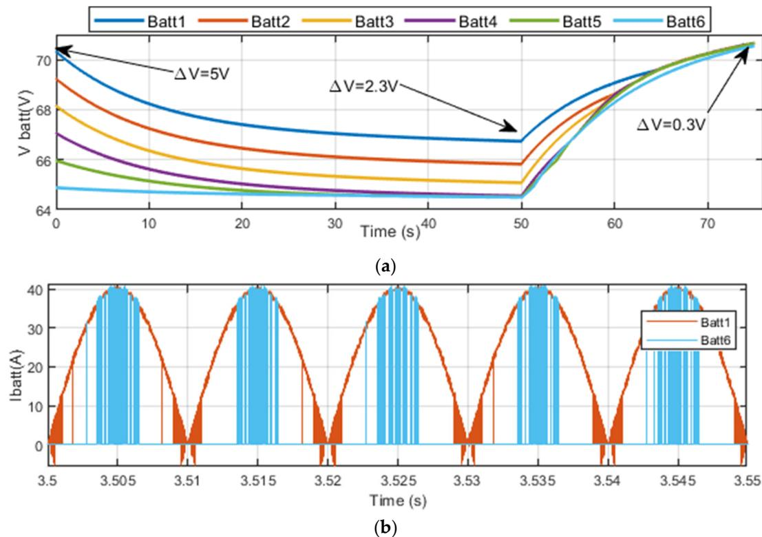
**Figure 23.** (a) Battery-module voltage profile during a charge-discharge-cycle test for AOP-PWM method with initial imbalance of 5.5 V, and (b) battery-module current profile for two modules with maximum and minimum OCV.
