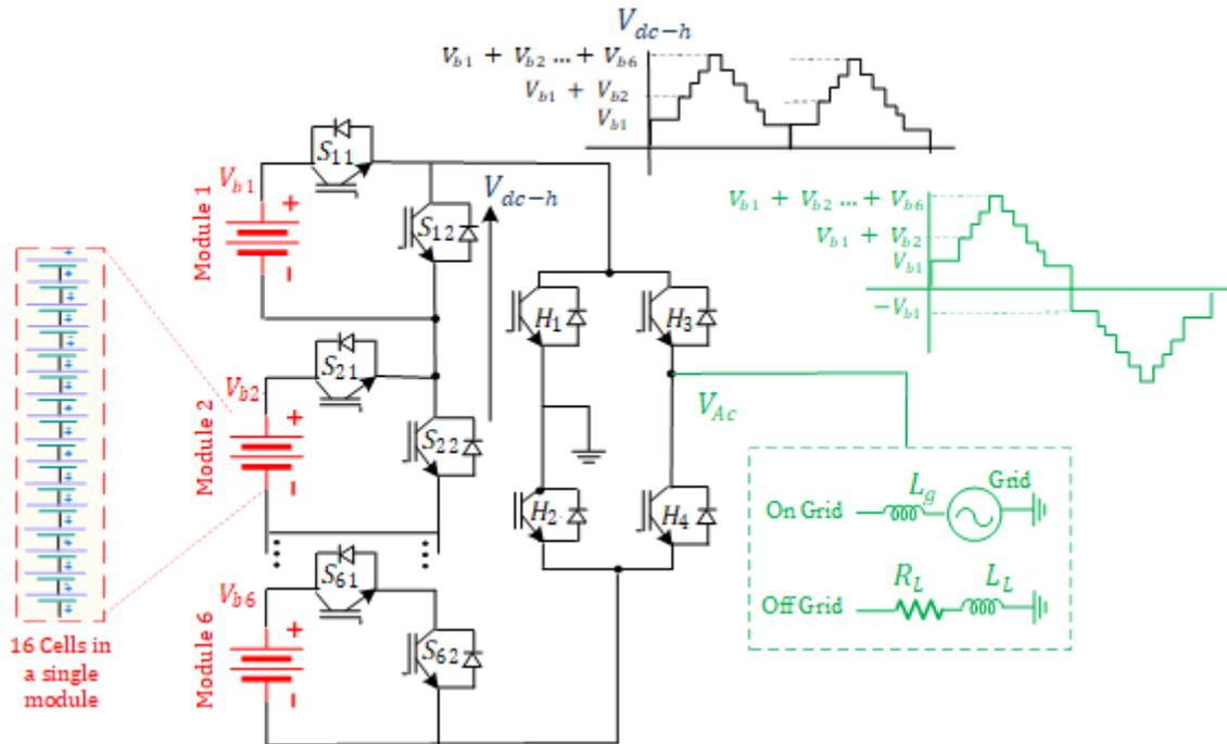
**Figure 6.** Schematic diagram of multiport 13-level RCHB topology comprising six isolated battery modules.
