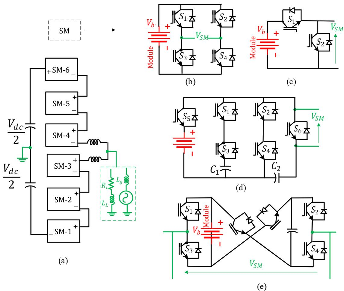
**Figure 8.** (a) Schematic diagram of a modular MLC in a single-phase system. Various configuration of SM, including (b) FB, (c) HB, (d) stacked switched capacitors, and (e) cross-connected SM configuration.
