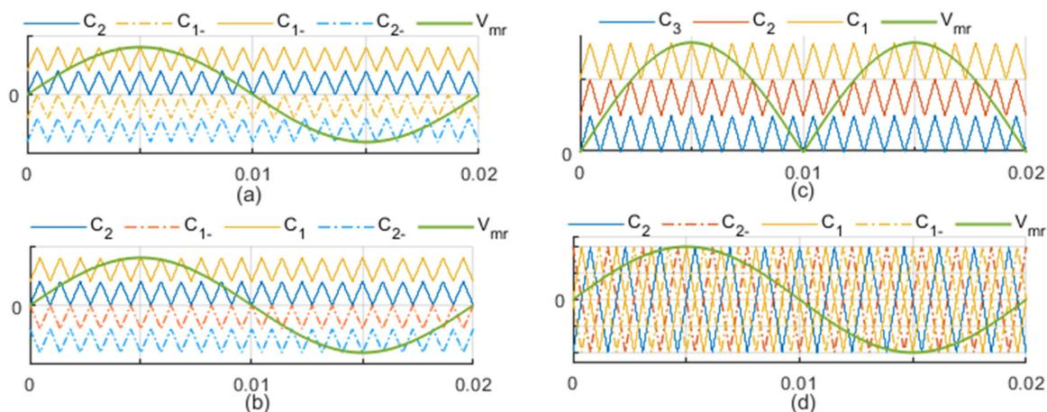
Figure 11. Various sub-techniques for LSC-based PWM scheme [105,106]: (a) equal-phase LSC PWM for FB structure, (b) opposite-phase LSC PWM for FB structure, (c) equal-phase LSC-PWM for HB structure, and (d) PSC PWM for FB structure.
