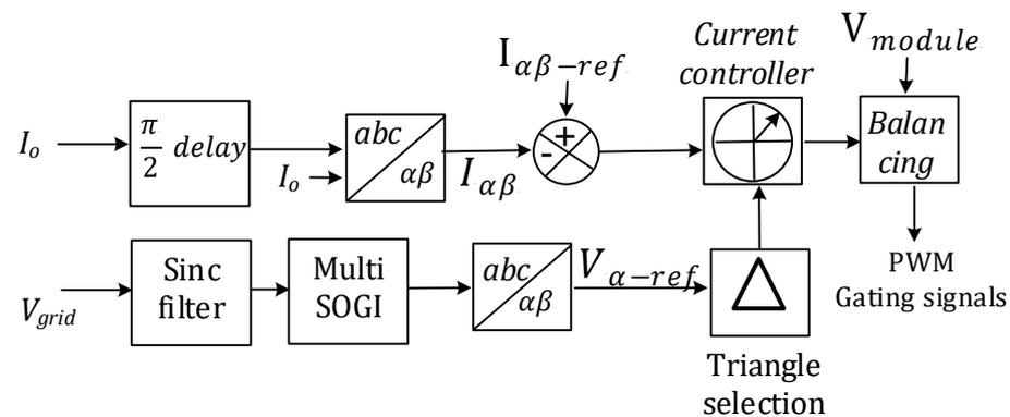
**Figure 15.** Schematic view of high-level direct-current controller [121].
