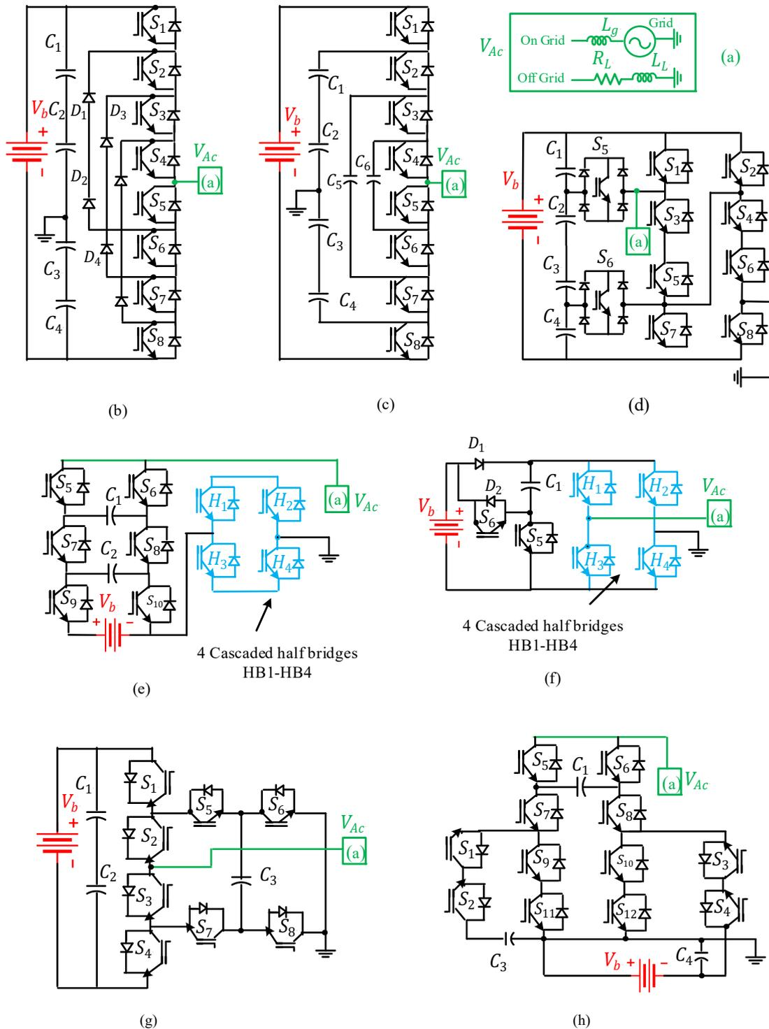
**Figure 3.** (a) Grid-connected and standalone load for MLC. Multiple configurations of the two-port MLC system fed by single/non-isolated BESSs. These include (b) NPC topology, (c) flying-capacitor topology, (d) cascaded-T configuration, (e) hybrid HB-FC topology, (f) hybrid SC-HB topology, (g) hybrid MLC (H8) topology, and (h) hybrid FC-ANPC topology.
