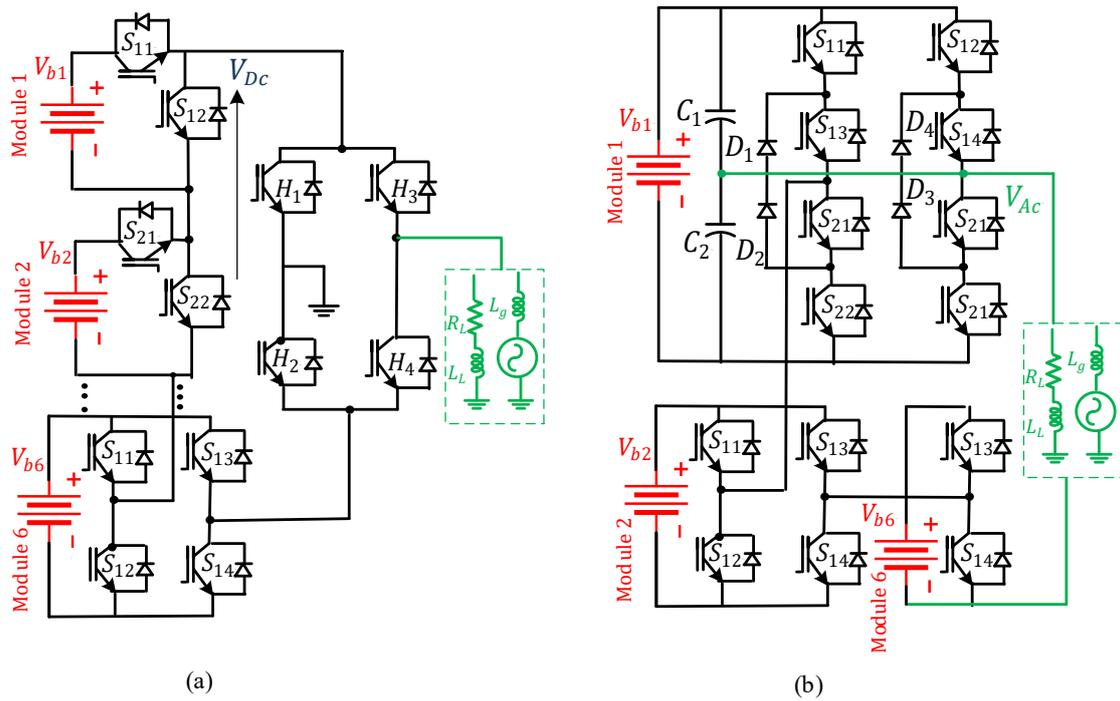
**Figure 9.** Schematic diagram of a hybrid MLC for (a) asymmetric cascaded configuration and (b) ANPC-CHB configuration.
