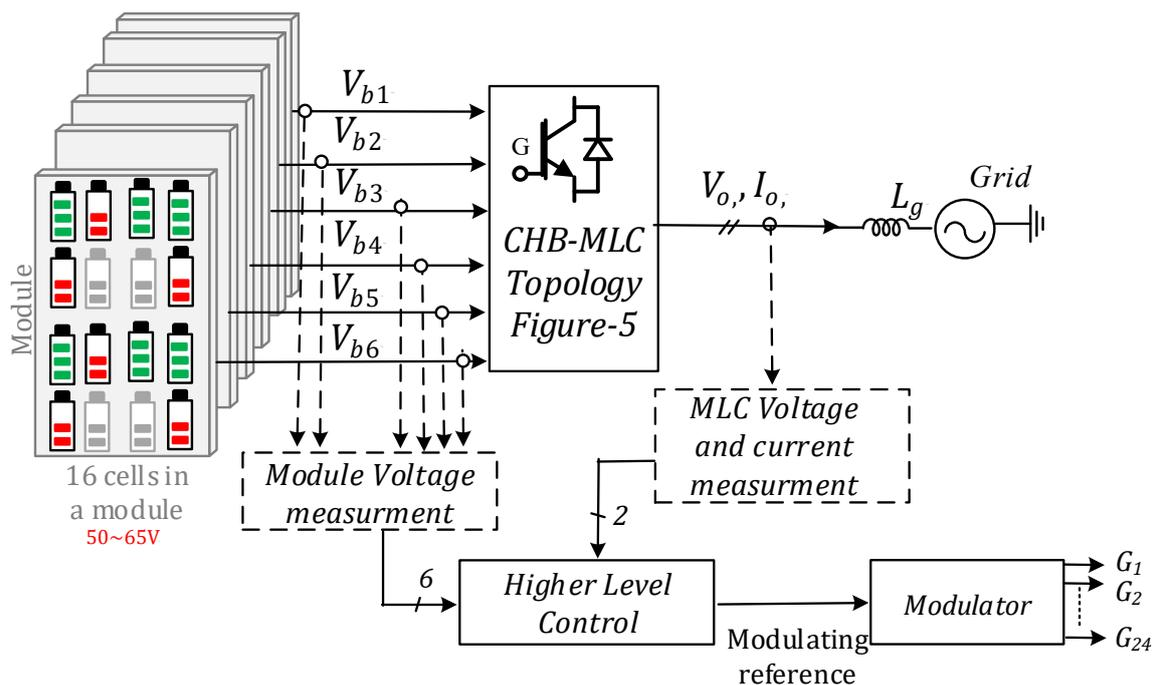
**Figure 19.** Schematic representation of single-phase CHB-MLC with voltage and current measurements.
