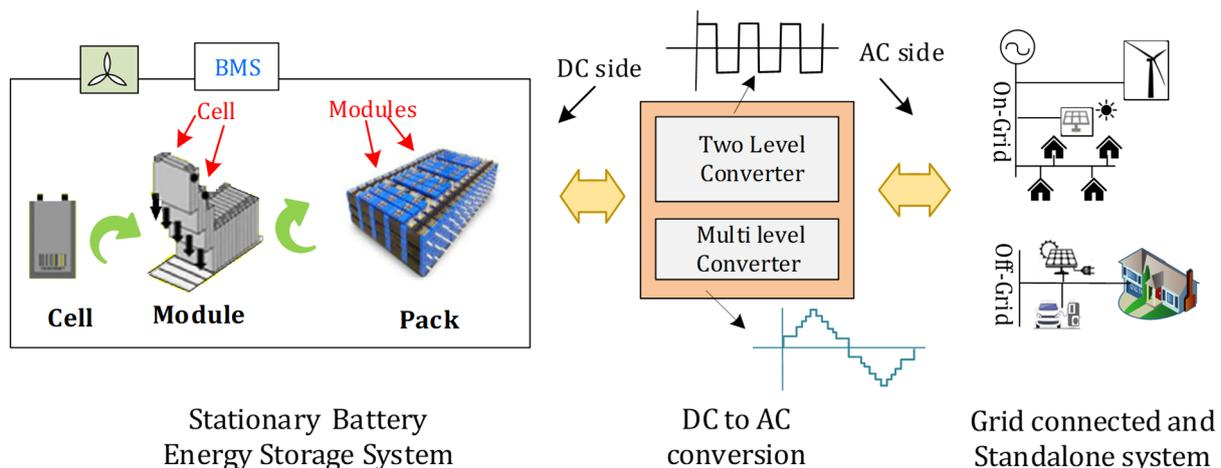
**Figure 1.** Schematic overview of stationary BESSs, power electronics converter, grid-connected system, and off-grid load.
