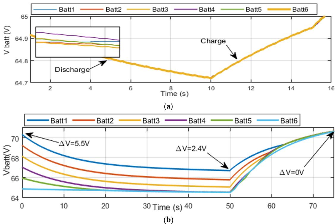
**Figure 21.** Battery-module voltage profile during a charge–discharge-cycle test for EP-PWM with (a) no initial imbalance in the module voltage and (b) a maximum initial imbalance of 5.5 V.
