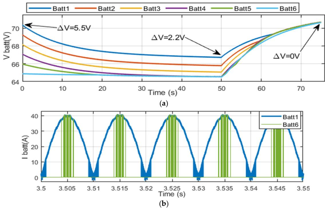
**Figure 22.** (a) Battery-module voltage profile during a charge-discharge-cycle test for OP-PWM method with initial imbalance of 5.5 V and (b) battery-module current profile for two modules with maximum and minimum OCV.
