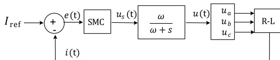
**Figure 16.** Schematic representation of the sliding-mode control scheme with a low-pass filter, reported in [130,131].
