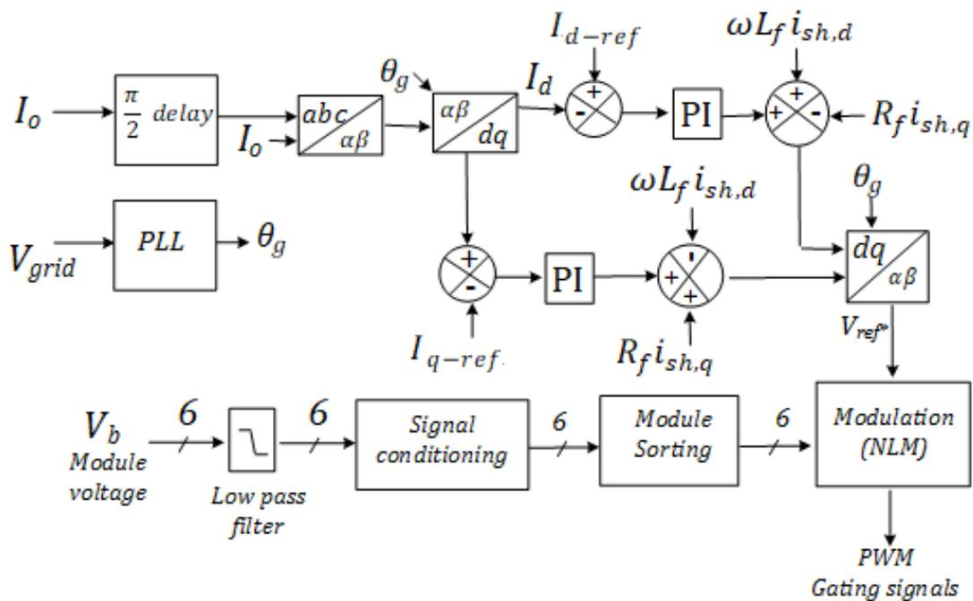
Figure 14. High-level VOC controller for CHB MLC [118].
