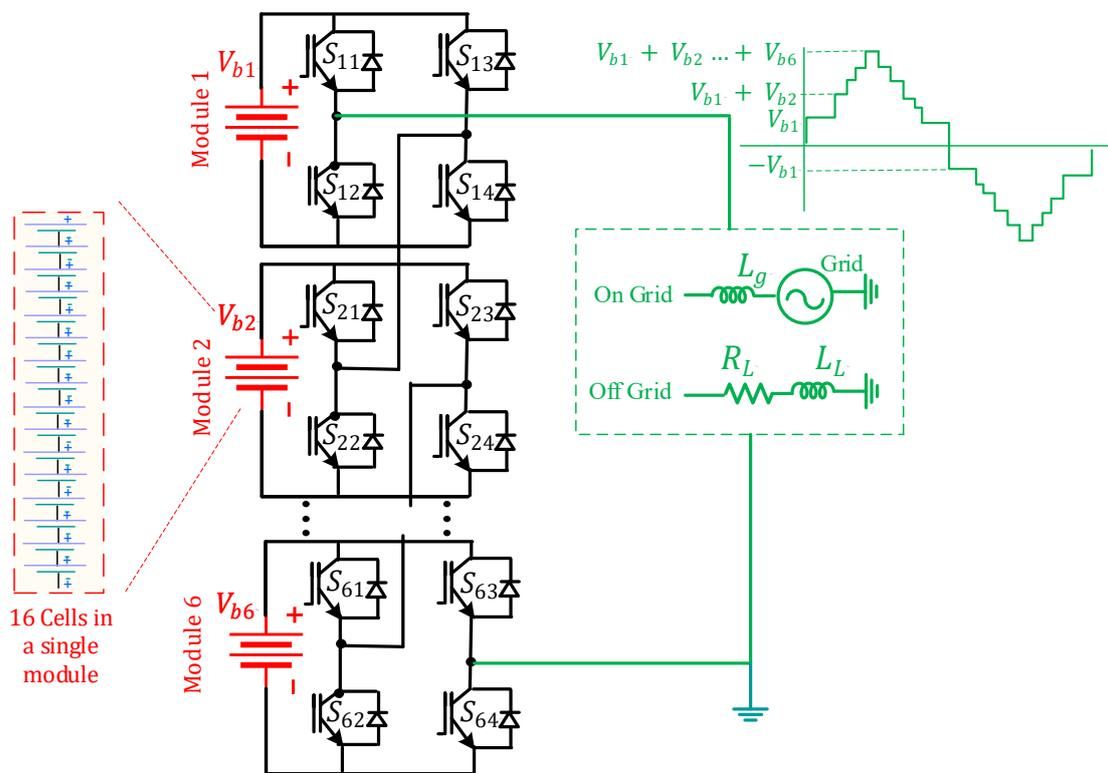
**Figure 5.** Schematic diagram of a multiport 13-level CHB system comprising six isolated battery modules.
