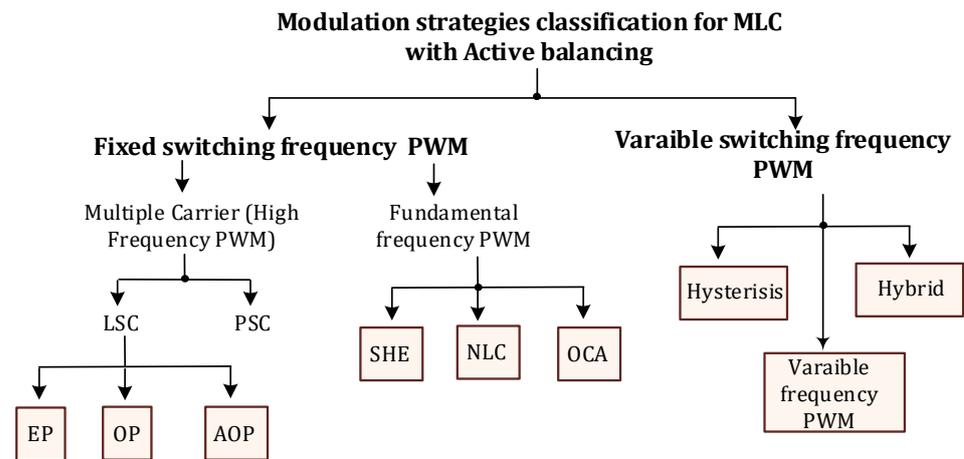
Figure 10. Modulation techniques for the MLC in compliance with the active-balancing role.
