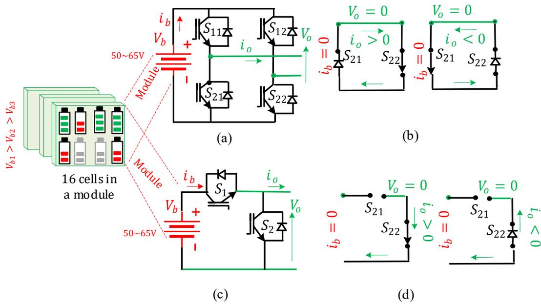
**Figure 4.** Operating modes of full-bridge and half-bridge interfaces with a single battery module: (a) generic full-bridge structure, (b) module-bypass state during discharging mode for full bridge, (c) generic half-bridge structure, and (d) module-bypass state during discharging state for half bridge.
