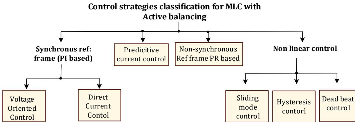
Figure 13. High-level control techniques for MLCs.
