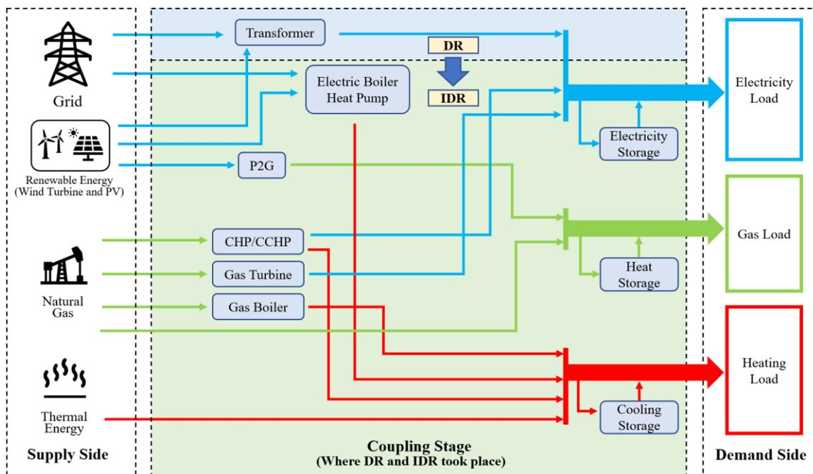
**Figure 5.** The schematic diagram of a typical integrated community energy system (source: authors’ edition).
