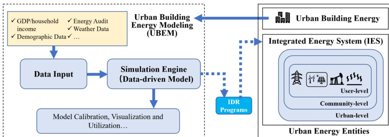
**Figure 7.** Schematic diagram of IES scheduling using IDR optimized by the UBEM model (source: authors' edition).
