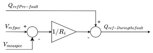
Figure 5. The control block of the voltage droop control.
