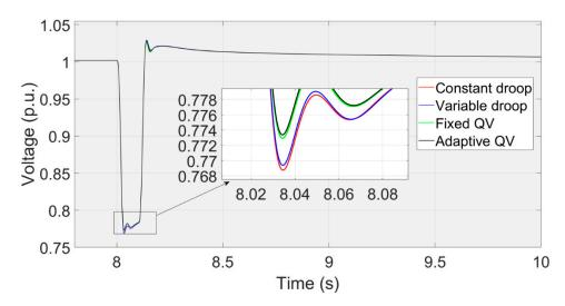
Figure 17. The transient voltage at the PCC using AC transmission.
