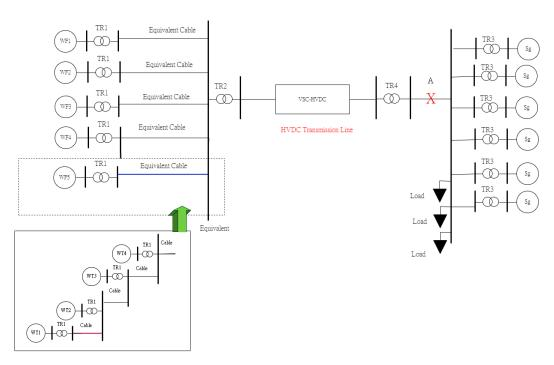
Figure 12. HVDC Test system.
