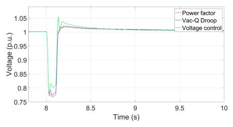
**Figure 19.** The transient voltage at the PCC using DC transmission.
