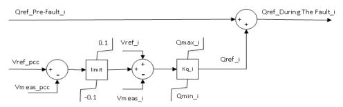
Figure 4. The control block of the adaptive QV control.
