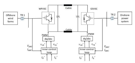
Figure 6. The control strategy of VSC-HVDC connected OWF.
