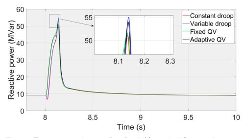
Figure 18. The transient reactive power from the wind farm using AC transmission.
