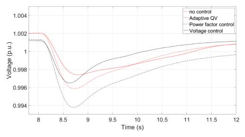
Figure 25. Transient voltage in Section 3.8.
