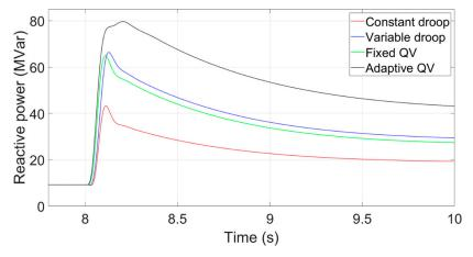
Figure 14. Transient Reactive power with an AC transmission system.
