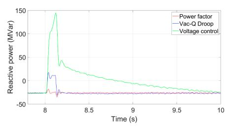
Figure 20. The transient reactive power from the wind farm using DC transmission.
