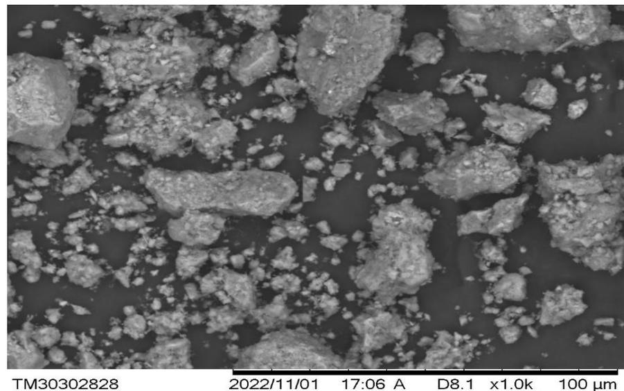
**Figure 7.** Micrographs of hardened samples of PC + 15% fly ash,  $\times 7000$ .
