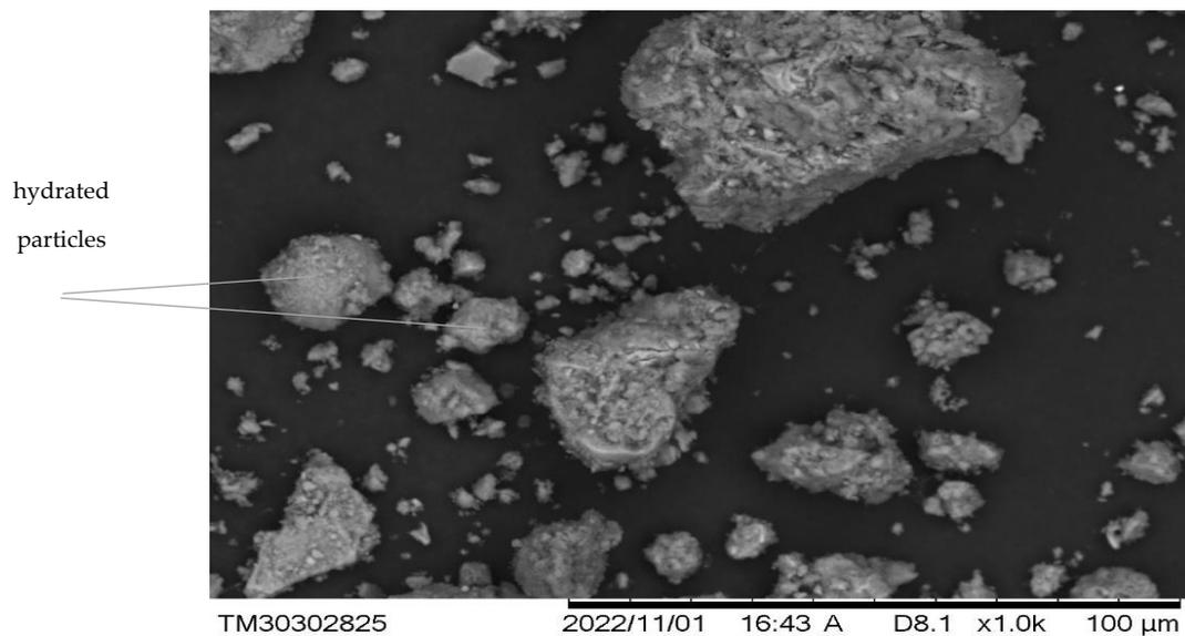
**Figure 4.** Micrographs of hardened samples without additives after 28 days of hardening,  $\times 1000$ .
