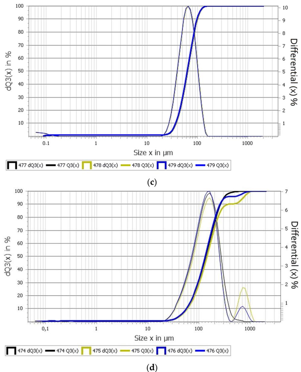
**Figure 1.** Particle size distribution: (a) fly ash sample; (b) fly ash sample b; (c) ash samples from ash disposal area; (d) ash samples from hydraulic ash disposal area.
