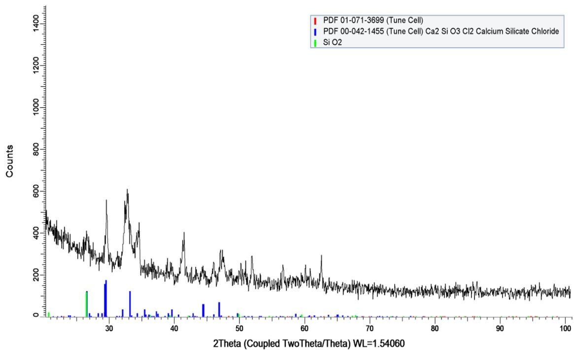
**Figure 8.** X-ray patterns of samples of PC + with fly ash 15% and superplasticizer, hardened within 3 days.
