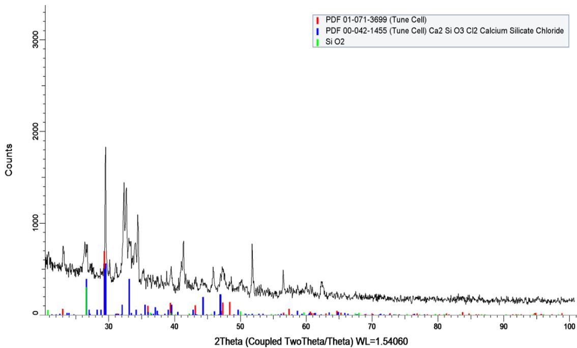
**Figure 9.** X-ray patterns of samples of PC + with fly ash 15% and superplasticizer, hardened within 7 days.
