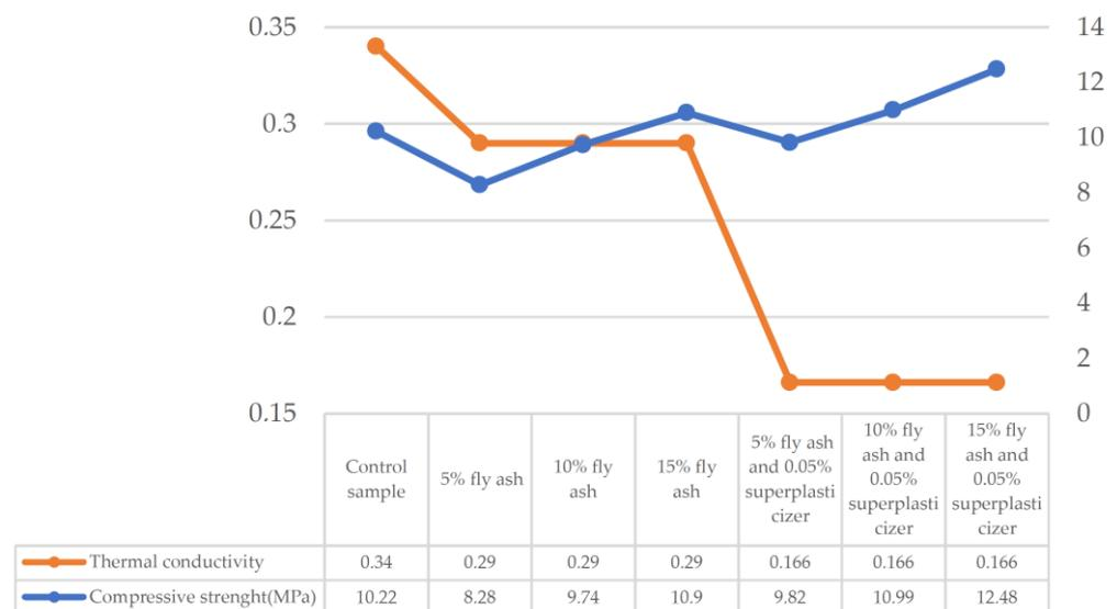
Figure 3. Dependence of polystyrene concrete compressive strength on thermal conductivity.
