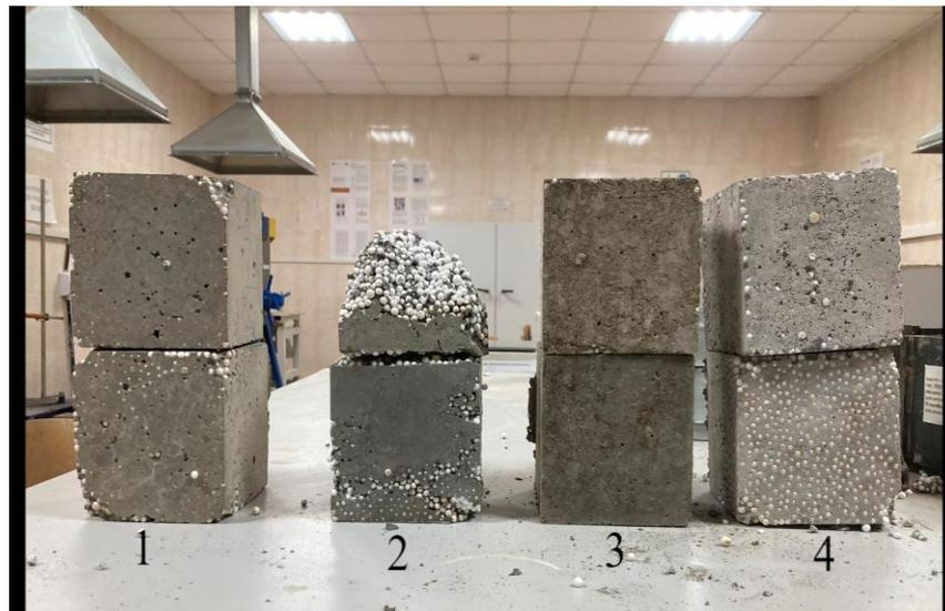
**Figure 2.** Prepared samples, where 1—control sample; 2—sample with the addition of superplasticizer; 3—sample with the addition of fly ash; 4—sample with the addition of fly ash and superplasticizer.
