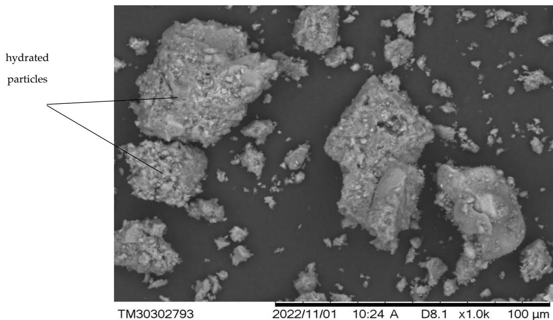
**Figure 5.** Micrographs of hardened samples of PC + 15% fly ash after 28 days of hardening,  $\times 10,000$ .
