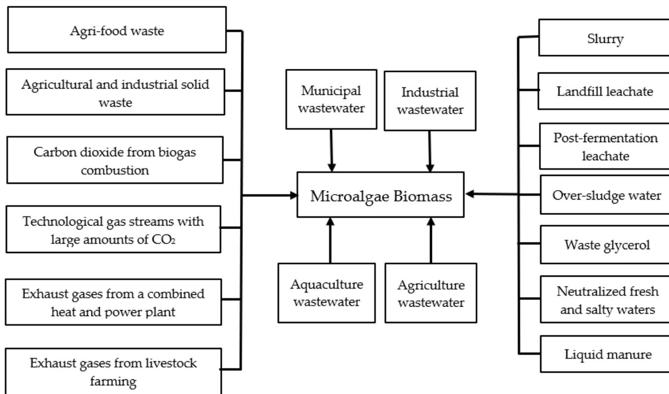
**Figure 2.** Primary types of waste used for microalgal biomass production.
