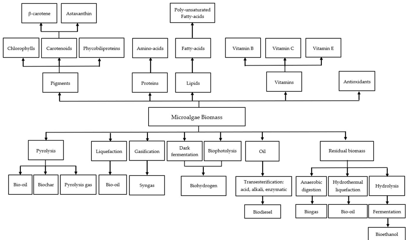
**Figure 1.** Primary processes used for converting microalgal biomass into biofuels, together with the major value-added products harvestable from microalgae.
