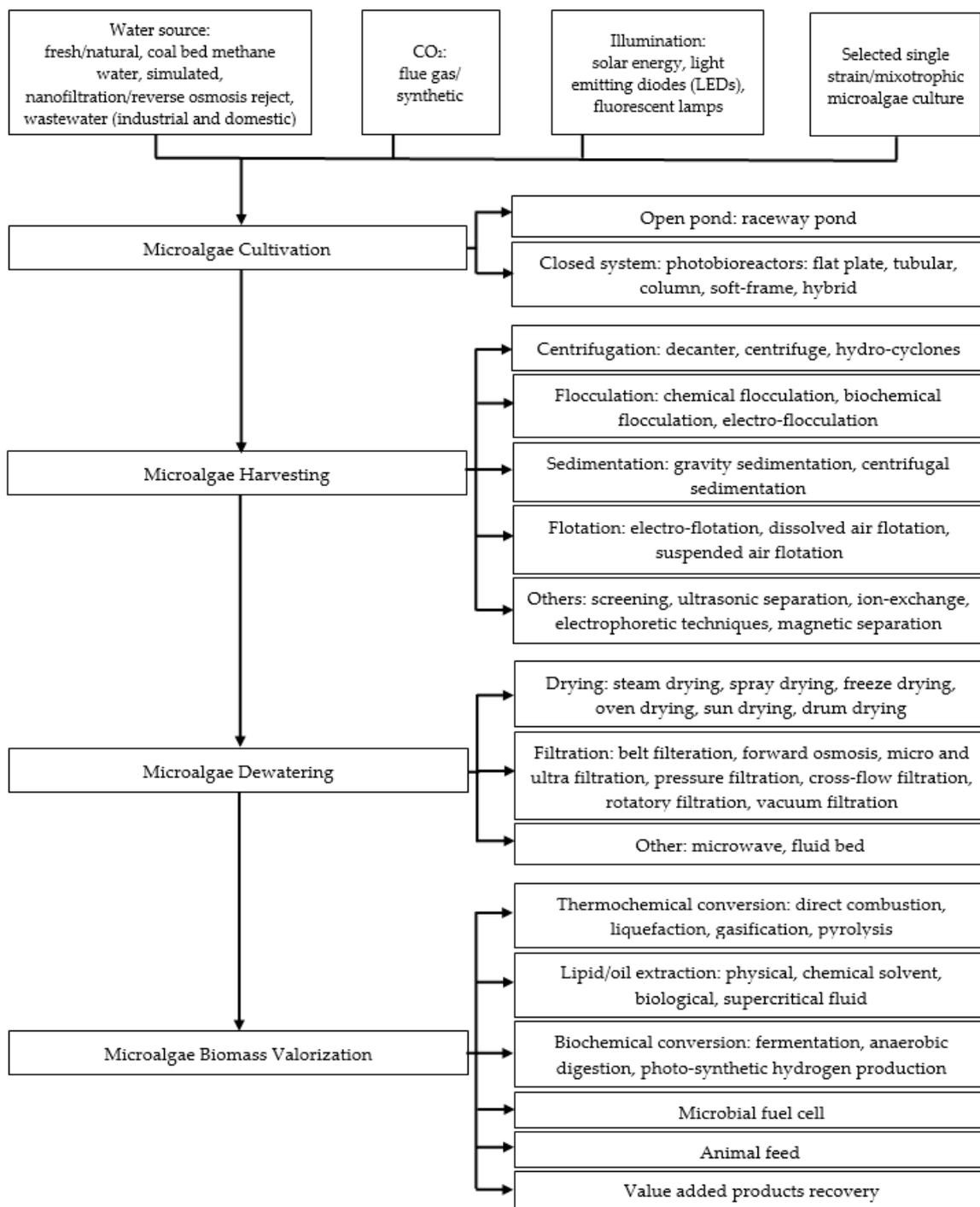
**Figure 4.** The many available process steps in microalgal biomass cultivation and microalgal-to-biofuel conversion.
