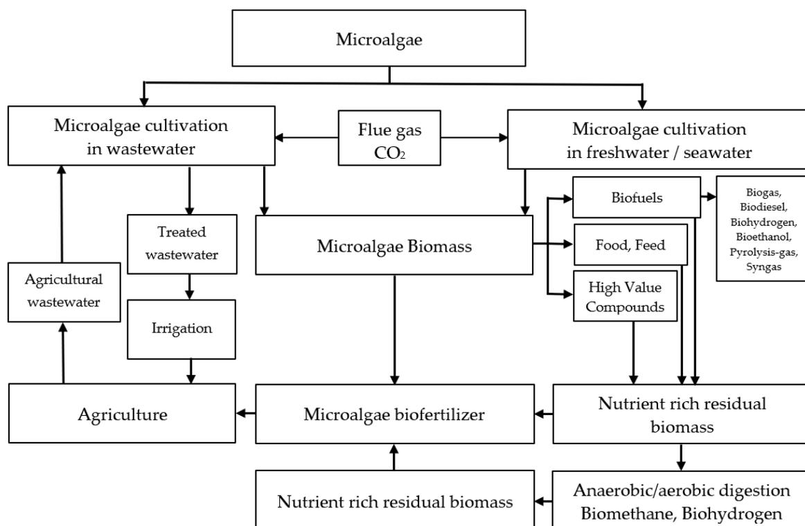
Figure 8. Microalgae biomass in a comprehensive biorefinery concept.
