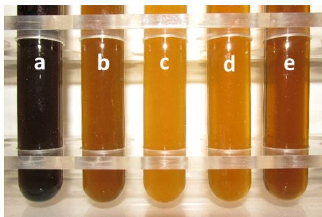
**Figure 8.** Visual changes in the quality of the liquid fraction of the digestate after successive stages of purification (a—liquid raw digestate; b—solution A (after struvite precipitation); c—solution A after FO with 0.5 mol/dm<sup>3</sup> NaCl; d—solution A after FO with 1 mol/dm<sup>3</sup> NaCl; e—solution A after FO with 3 mol/dm<sup>3</sup> NaCl).
