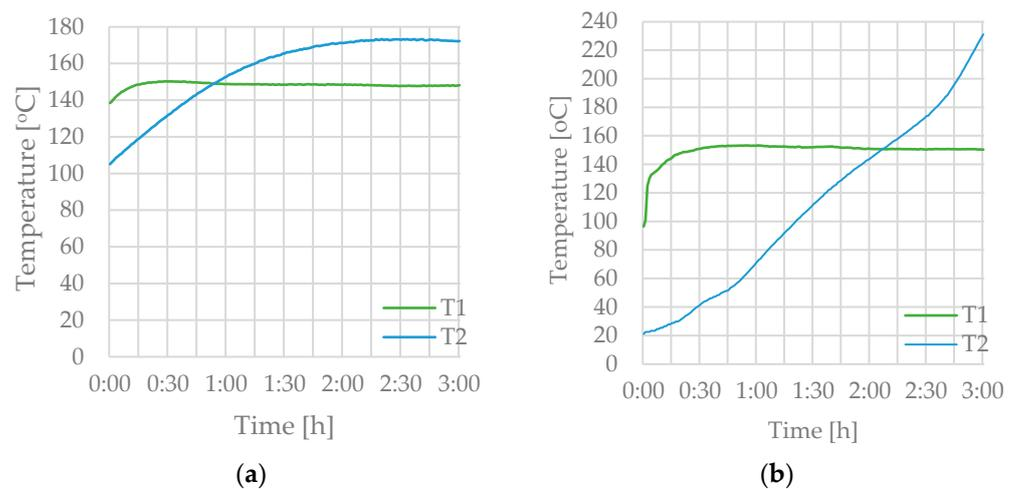
**Figure 5.** The temperature of sludge dust in a 50.27 cm<sup>3</sup> basket: (a) at a furnace temperature of 148 °C with no evidence of dust ignition, (b) at a furnace temperature of 150 °C with a dust ignition.
