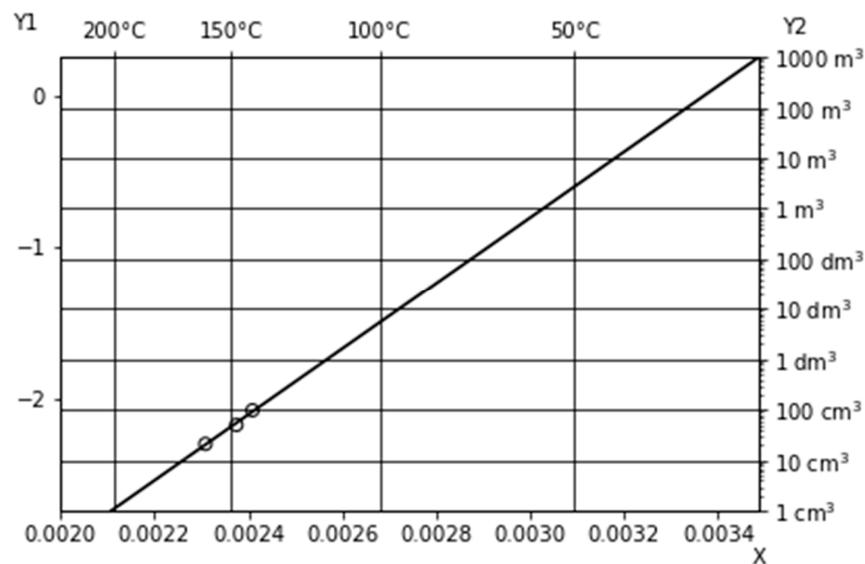
**Figure 10.** Pseudo-Arrhenius graph of the self-ignition temperature of the sludge dust.
