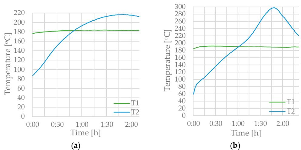
**Figure 7.** The temperature of sludge pellets in a 21.21 cm<sup>3</sup> basket: (a) at a furnace temperature of 186 °C with no evidence of dust ignition, (b) at a furnace temperature of 188 °C with a dust ignition.
