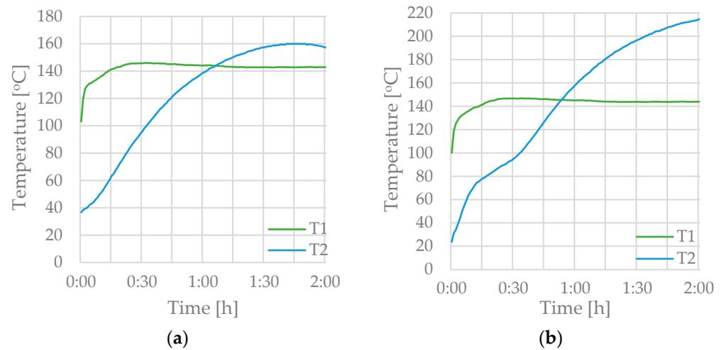
**Figure 6.** The temperature of sludge dust in a 98.17 cm<sup>3</sup> basket: (a) at a furnace temperature of 142 °C with no evidence of dust ignition, (b) at a furnace temperature of 144 °C with a dust ignition.
