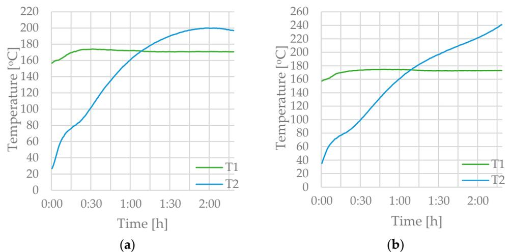
**Figure 8.** The temperature of sludge pellets in a 50.27 cm<sup>3</sup> basket: (a) at a furnace temperature of 170 °C with no evidence of dust ignition, (b) at a furnace temperature of 172 °C with a dust ignition.
