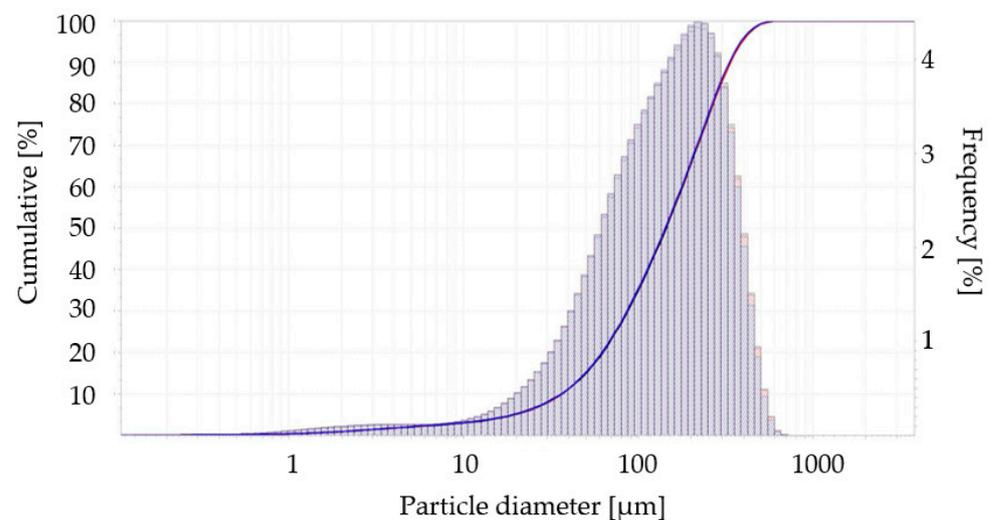
**Figure 1.** The frequency distribution and cumulative frequency of particle size distribution of sludge dust (measurement 1).
