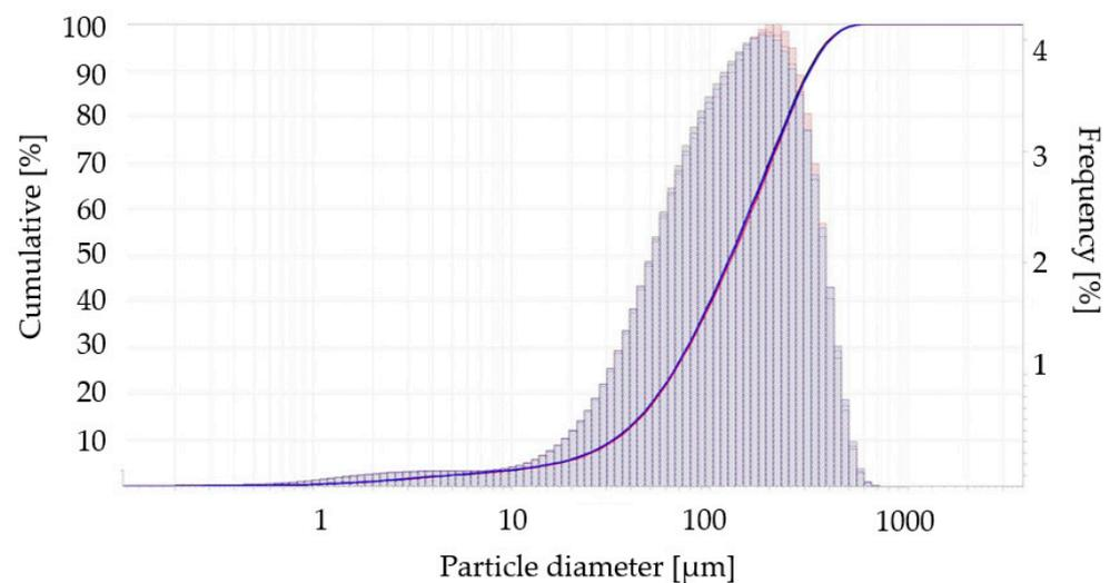
**Figure 2.** The frequency distribution and cumulative frequency of particle size distribution of sludge dust (measurement 2).**Table 6.** Results of the third particle size distribution analysis in terms of cumulative frequency.
