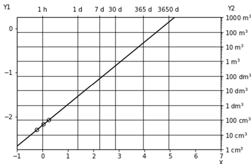
**Figure 13.** Dependence of the induction time of the combustion ( $t_i$ ) on the volume/surface ratio of the sludge pellets.
