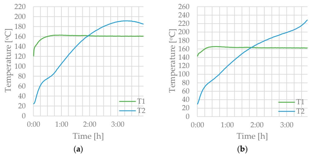
**Figure 9.** The temperature of sludge pellets in a 98.17 cm<sup>3</sup> basket: (a) at a furnace temperature of 160 °C with no evidence of dust ignition, (b) at a furnace temperature of 162 °C with a dust ignition.
