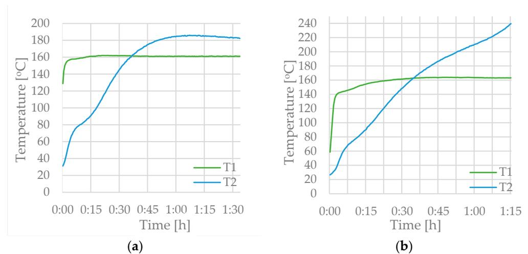
**Figure 4.** The temperature of sludge dust in a 21.21 cm<sup>3</sup> basket: (a) at a furnace temperature of 160 °C with no evidence of dust ignition, (b) at a furnace temperature of 162 °C with a dust ignition.
