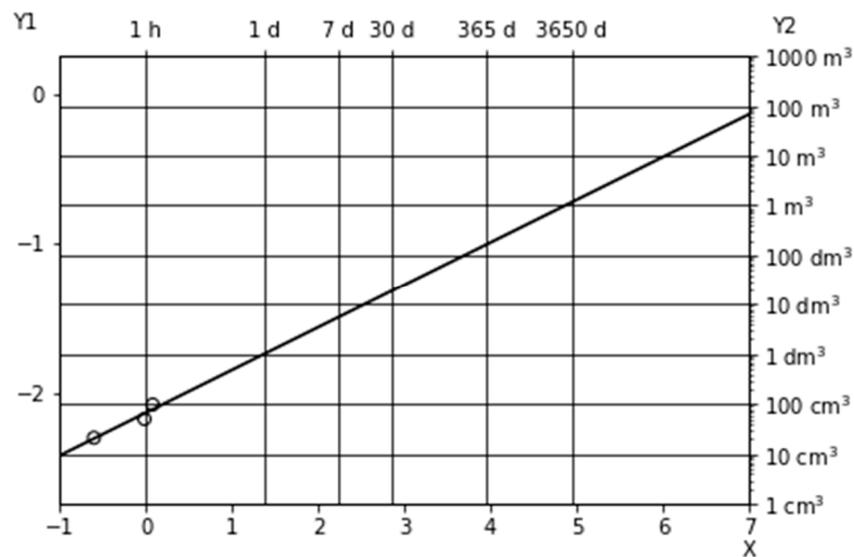
**Figure 11.** Dependence of the induction time of the combustion ( $t_i$ ) on the volume/surface ratio of the sludge dust.
