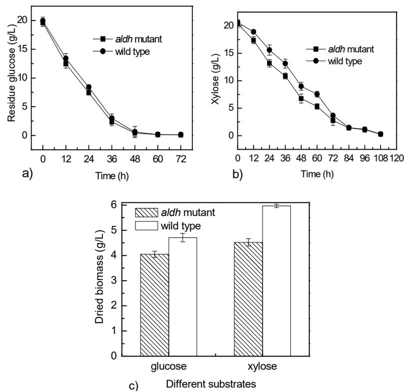
**Figure 6.** Xylose and glucose utilization and cell growth profile for *F. oxysporum* strain cs28 and mutant strain cs28pCAM-Pstal- $\Delta$ aldh. Cells were cultured in 50 mL of fermentation medium with 20 g/L of glucose (a) and 20 g/L of xylose (b), and dried biomass was weighed at 105 °C for 4 h (c). Symbols: ●: wild-type strain cs28; ■: *aldh* mutant strain cs28pCAM-Pstal- $\Delta$ aldh; □: wild-type strain cs28; ▨: *aldh* mutant strain cs28pCAM-Pstal- $\Delta$ aldh.
