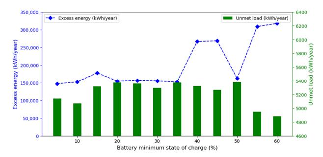
**Figure 17.** The effect of varying the battery SOC<sub>minimum</sub> percent value on the technical performance of the optimal charging system.
