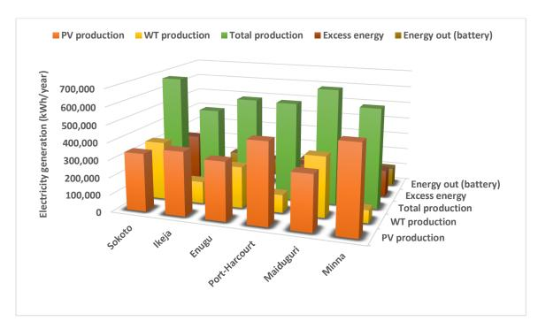
**Figure 8.** Yearly electric generation of the optimal charging station schemes (PV/WT/battery) in the considered locations.
