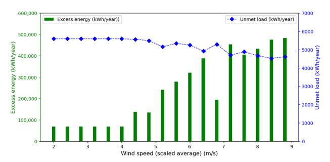
**Figure 15.** The effect of wind speed variation on the technical performance of the Sokoto PV/WT/battery EV charging model.
