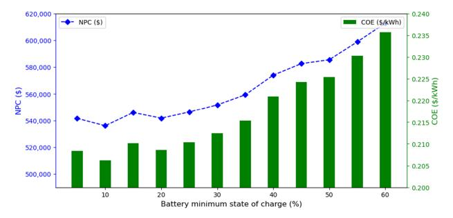
**Figure 12.** Effect of varying the battery SOC<sub>minimum</sub> on the NPC and the COE of the optimal charging system.
