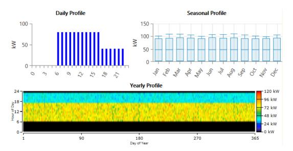
Figure 6. EV charging station system load profile.
