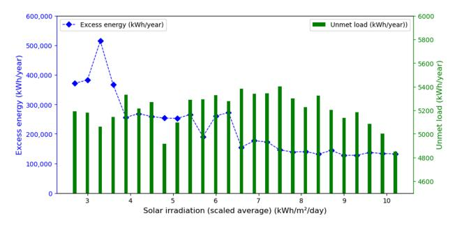
**Figure 16.** The impact of changing the solar radiation value on the excess energy and unfulfilled electric load of the optimal EV charging scheme.
