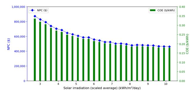
**Figure 11.** Impact of change in solar radiation value on the PV/WT/battery charging station costs in Sokoto.
