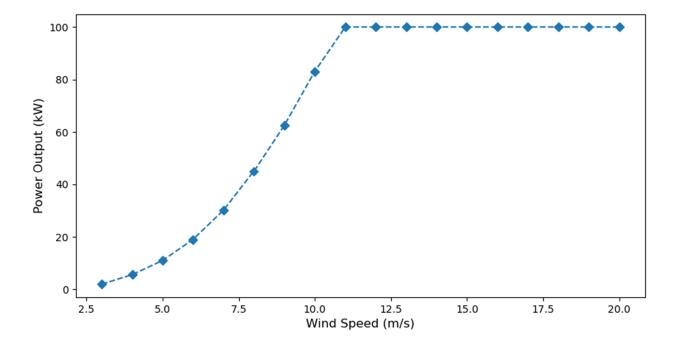
Figure 5. The WT power curve.
