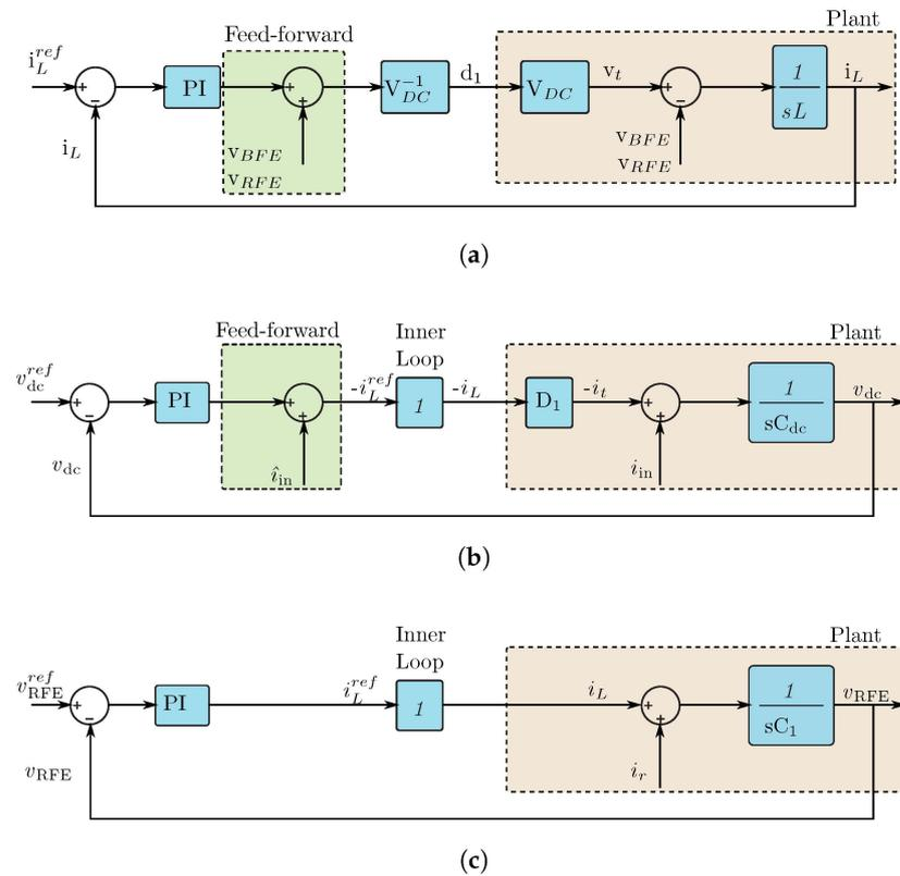
Figure 9. Control loops: (a) inductor current, (b) DC link voltage control loop, and (c) RFE terminal voltage control loop.
