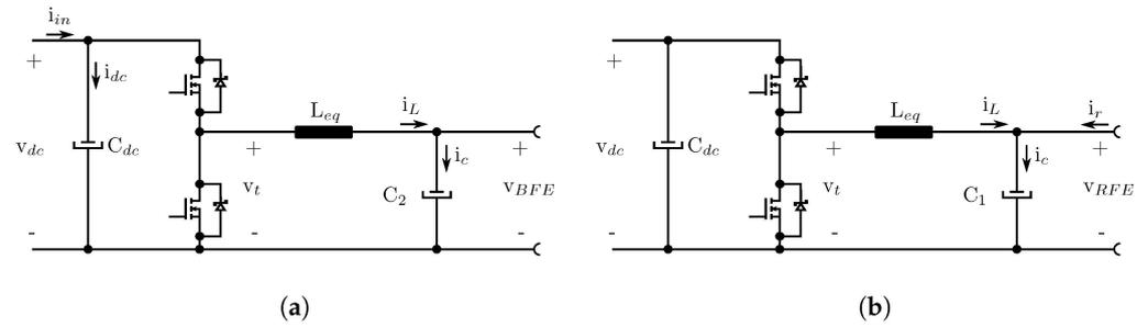
Figure 8. (a) Equivalent converter circuit diagram: (a) BFE and (b) RFE.
