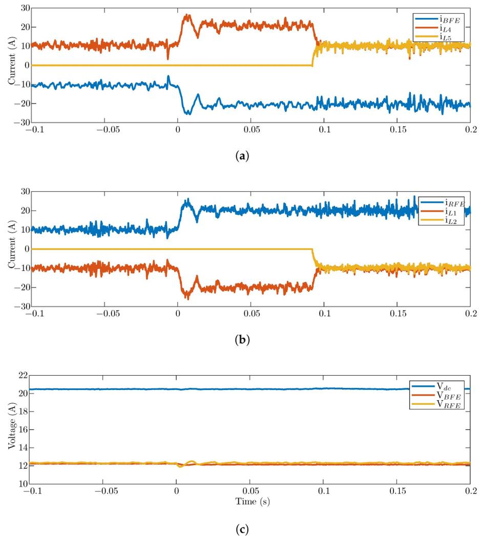
**Figure 11.** Converter response to a load step from 10 to 20 A. As the controller updates the RMS current value, it turns the second leg on and handles the current sharing, disturbing the terminal voltages. (a) BFE currents; (b) RFE currents; (c) BFE, DC, and RFE voltages.
