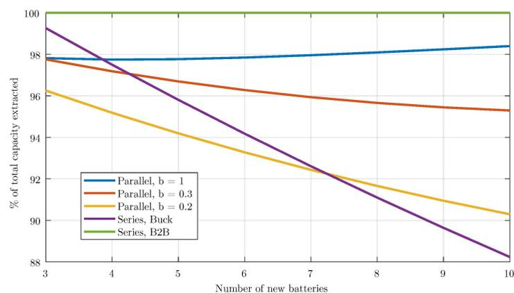
**Figure 5.** Percentage of energy extracted from a bank with 20 batteries depending on the system architecture, when the new batteries change ( $x$ -axis).
