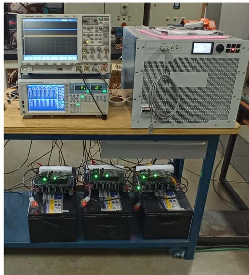
**Figure 10.** Test set-up with three smart battery modules in the series.
