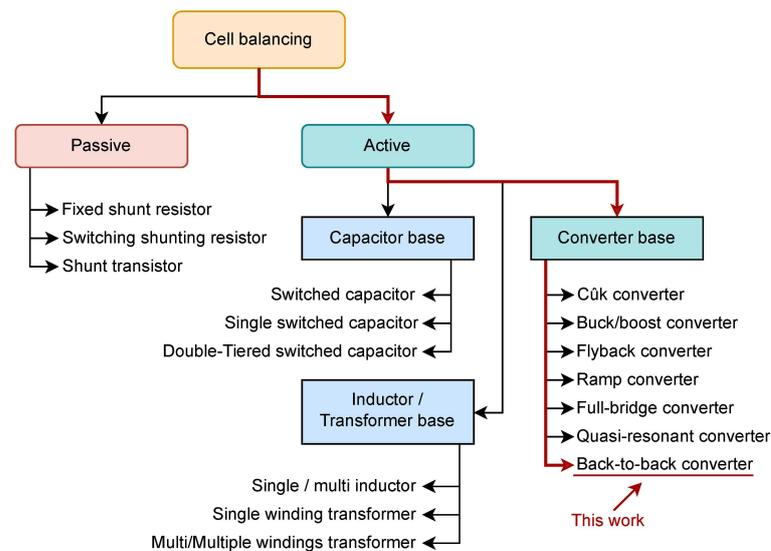
**Figure 1.** Classification of battery/cell equalization technologies [6].
