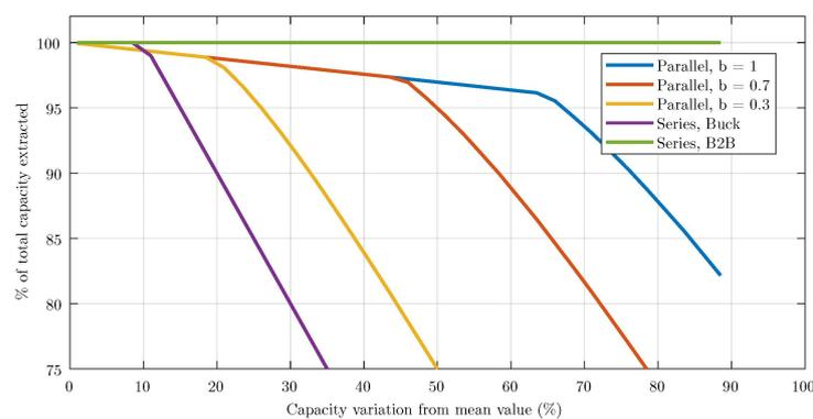
**Figure 4.** Bank extractable energy depending on the charge distribution and the implementation strategy.
