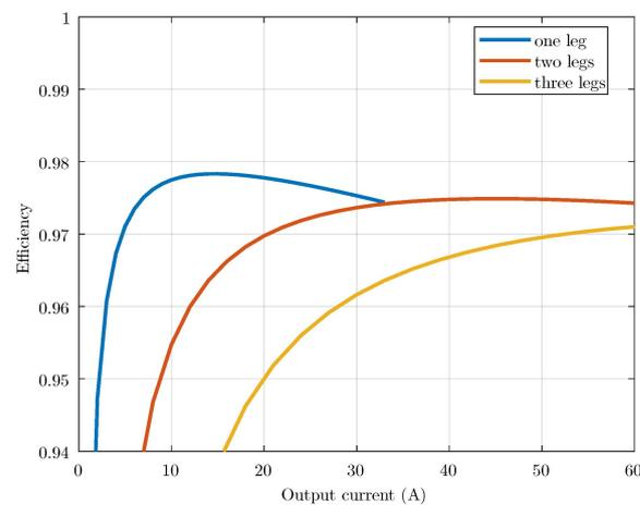
**Figure 7.** Full converter efficiency with one, two, or three switching legs.
