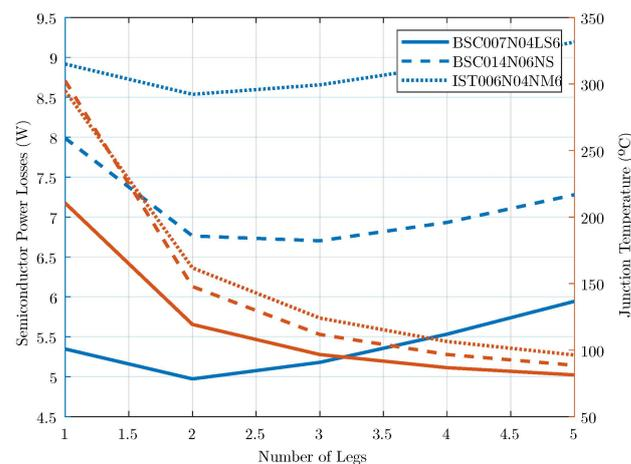
**Figure 6.** Semiconductor power losses (blue lines) and the estimated junction temperature (red lines).
