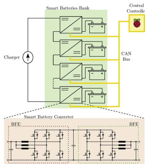
**Figure 2.** Proposed series cell-to-pack module-integrated bank based on back-to-back converters.
