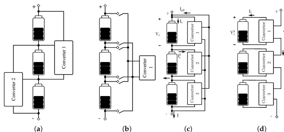
**Figure 3.** Equalization architectures based on energy redistribution balancing: (a) adjacent cell-to-cell, (b) direct cell-to-cell, (c) parallel cell-to-pack, and (d) series cell-to-pack.
