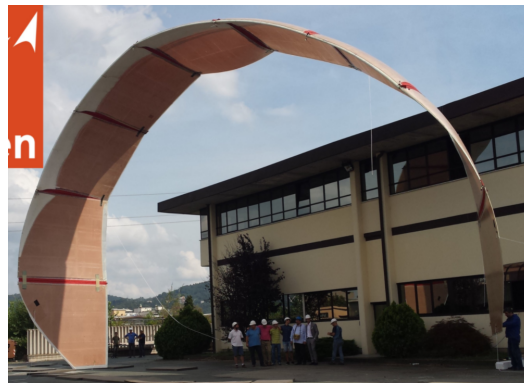
Figure 19. Semirigid curved wing of KiteGen. [46]. Reproduced with permission. All rights reserved.
