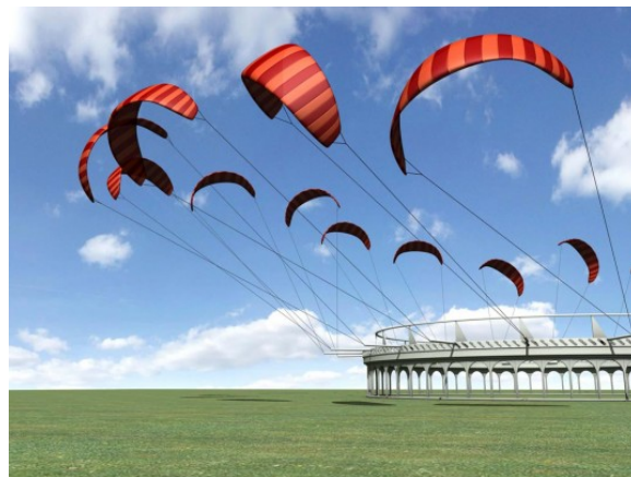
Figure 11. KiWiGen Carousel generator [68]. Reproduced with permission. All rights reserved.
