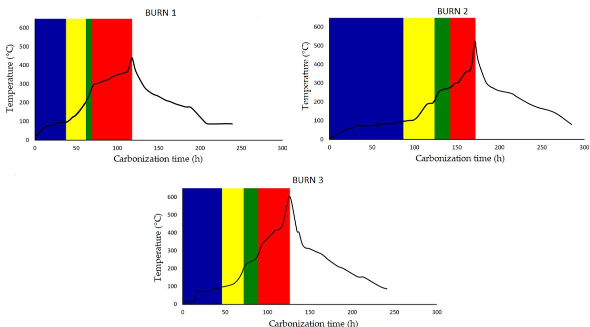
**Figure 6.** Heating ramps during carbonization in three burnings of Brazilian beehive kilns. Blue color = phase 1, yellow color = phase 2, green color = phase 3, red color = phase 4, white color = phase 5. This carbonization process includes the following species: Madrone, White oak, and Red oak.
