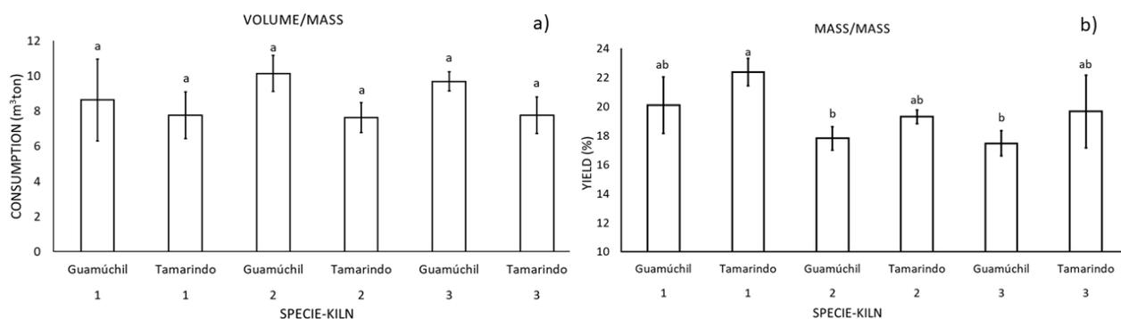
**Figure 10.** (a) Firewood consumption, and (b) charcoal production yield in modified Brazilian beehive kilns. Values with the same letter are statistically equal, according to Tukey test ( $p \geq 0.05$ ).
