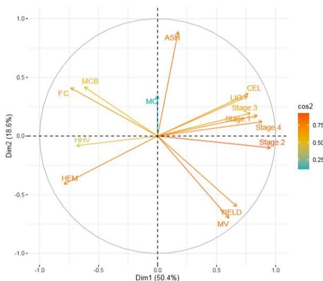
**Figure 13.** Principal Component Analysis (PCA), representing the two main components. MC = moisture content (%), MCB: wood moisture content MV = volatile material (%), FC = fixed carbon (%), ASH = ash content (%), HHV = Heating value, CEL = Cellulose, Lig = Lignin, HEM = Hemicelulosa.
