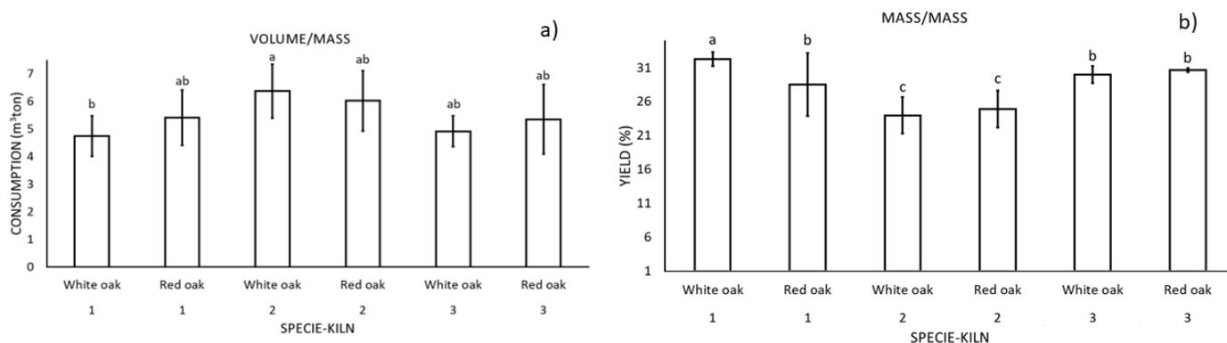
**Figure 11.** (a) Firewood consumption and (b) charcoal production yield in Argentine half-orange kilns. Values with the same letter are statistically equal, according to Tukey test ( $p \geq 0.05$ ).
