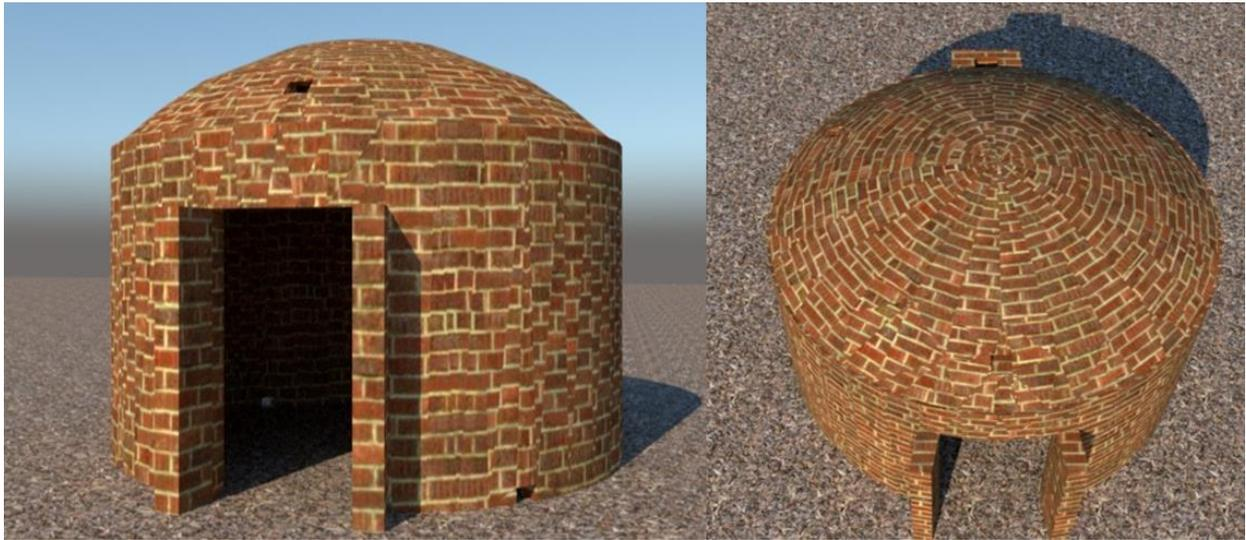
**Figure 3.** Design of a modified Brazilian beehive type kiln.
