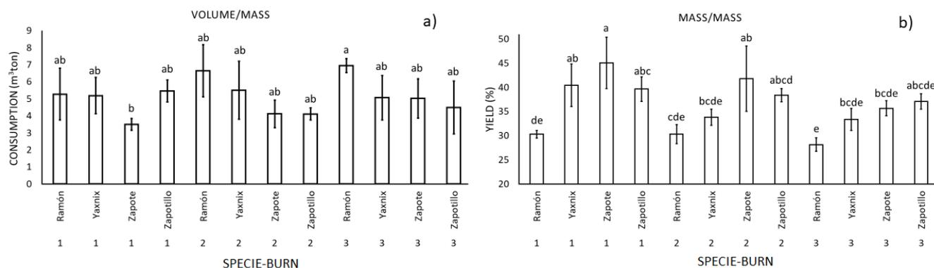
**Figure 12.** (a) Firewood consumption and (b) charcoal production yield in industrial metal kilns. Values with the same letter are statistically equal, according to Tukey test ( $p \geq 0.05$ ).
