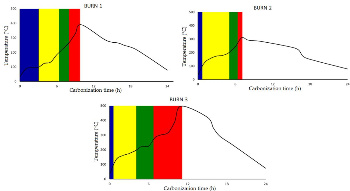
**Figure 9.** Heating ramps during carbonization in three burnings of industrial metal kilns. Blue color = phase 1, yellow color = phase 2, green color = phase 3, red color = phase 4, white color = phase 5. This carbonization process includes the following species: Ramón, Yaxnic, Zapote, and Zapotillo.
