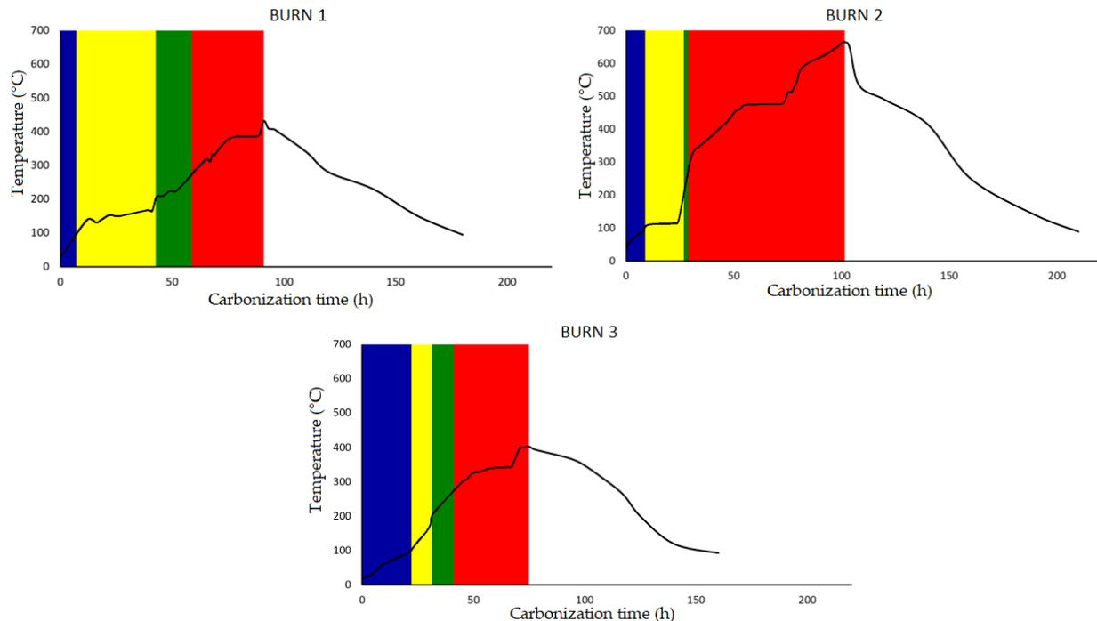
**Figure 8.** Heating ramps during carbonization in three burnings of Argentine half-orange kilns. Blue color = phase 1, yellow color = phase 2, green color = phase 3, red color = phase 4, white color = phase 5. This carbonization process includes the following species: White oak and Red oak.
