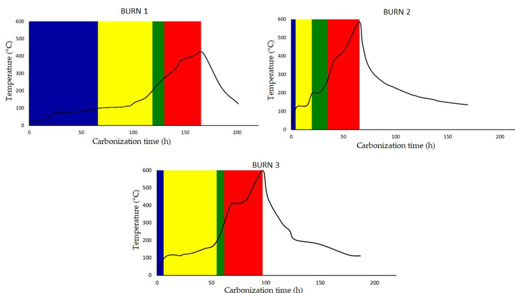
**Figure 7.** Heating ramps during carbonization in three burnings of modified Brazilian beehive kilns. Blue color = phase 1, yellow color = phase 2, green color = phase 3, red color = phase 4, white color = phase 5. This carbonization process includes the following species: Guamúchil and Tamarindo.
