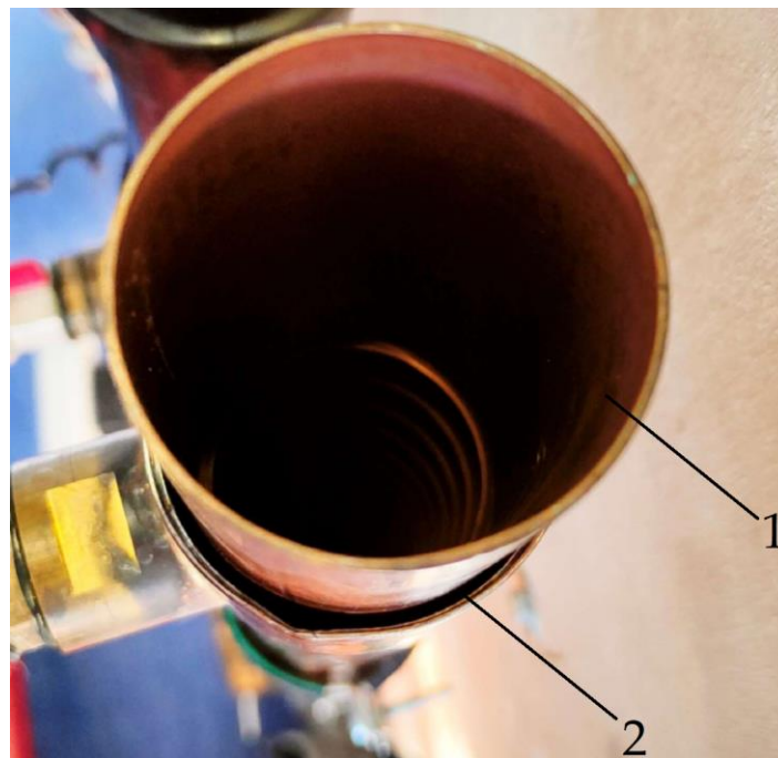
Figure 7. Typical cross section of a vertical heat exchanger; 1—grey water drain, 2—cold water drain.
