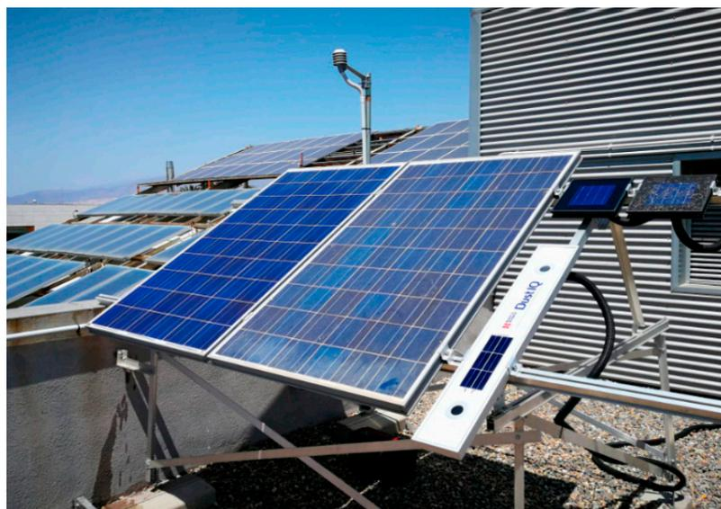
**Figure 3.** Outdoor PV panel testing facility with clean and dusty panels [30].
