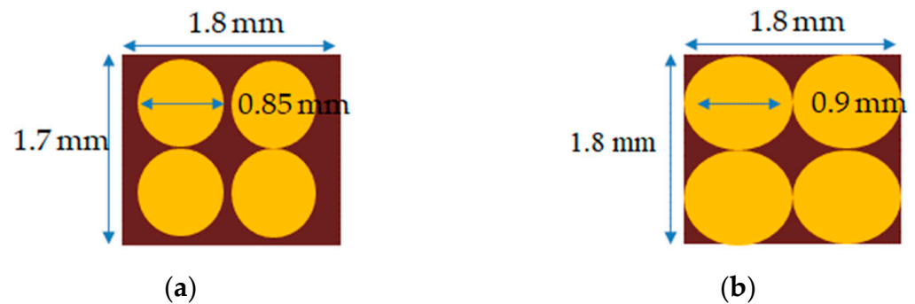
Figure 13. Coil empty space comparison: (a) 0.85 m, (b) 0.9 mm.
