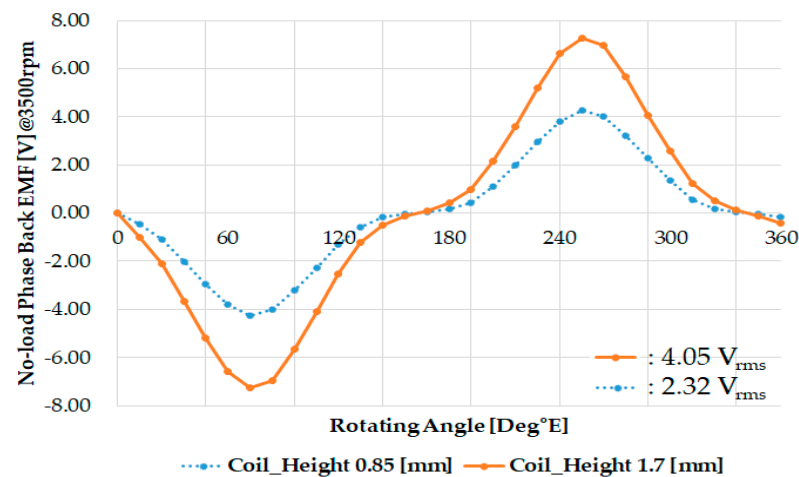
Figure 8. No load phase back-EMF compared to coil height 0.85 mm (Blue) and coil height 1.7 mm (Red).
