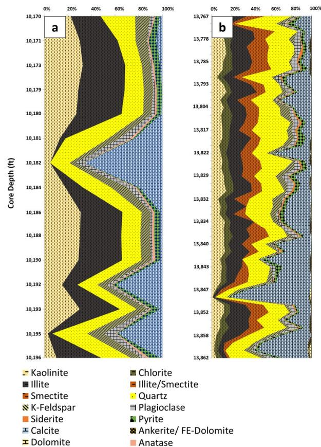
**Figure 4.** Whole-rock XRD mineralogy for: (a) Well CFU 31F-2 in Cranfield field, MS, and (b) a well in the East Feliciana Parish, LA.
