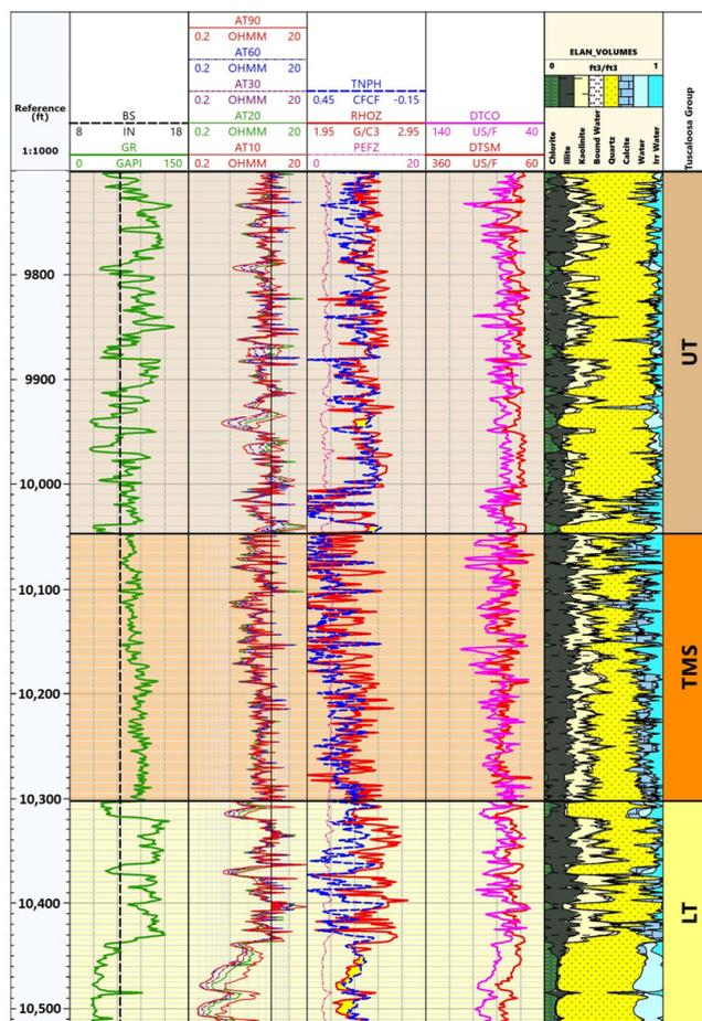
**Figure 3.** Type log of Well CFU 31F-2 in Cranfield field, MS.
