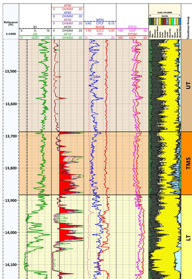
**Figure 2.** Type log of the Tuscaloosa Marine Shale in a well in the East Feliciana Parish, LA.
