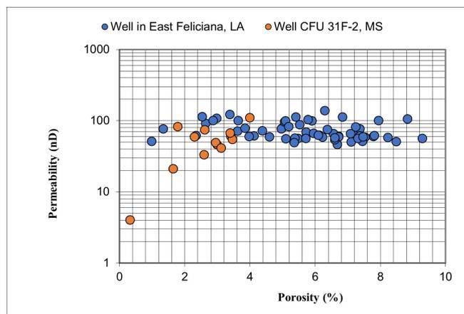
**Figure 5.** Plot showing permeability versus porosity estimates for samples acquired from a well in the East Feliciana Parish, LA (data points in blue), and Well CFU 31F-2 in Cranfield field, MS (data points in orange).
