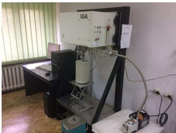
**Figure 5.** IGA-001 gravimetric sorption system used to investigate methane sorption kinetics and methane sorption isotherms.
