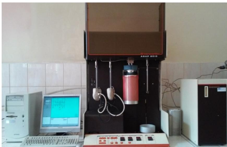
**Figure 6.** ASAP 2010 volumetric sorption analyser.
