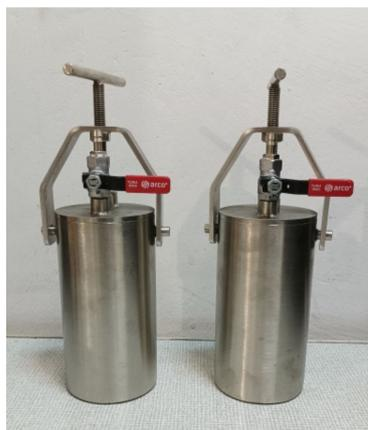
**Figure 2.** Hermetically sealed containers for coal sampling.
