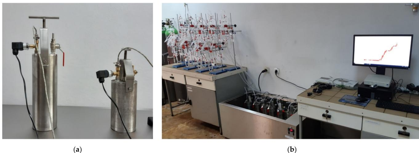
**Figure 3.** Central Mining Institute test stand for methane-bearing capacity identification by the USBM direct method: (a) Hermetically sealed steel containers with pressure and temperature sensors; (b) Central Mining Institute USBM dedicated test stand.
