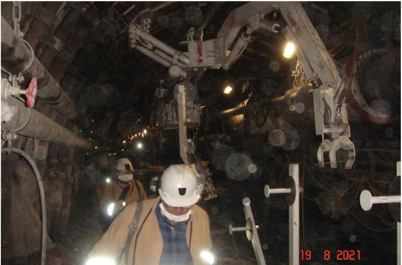
**Figure 20.** View of the MZT-M installed in an underground excavation.
