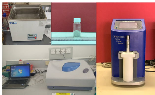
Figure 7. Zeta potential (ZP) measurements; Zeta-sizer (SZ-100) ( bottom left ), the ultrasonic bath ( top left ), and Zeta-check (Particle Matrix GmbH) ( right ).
