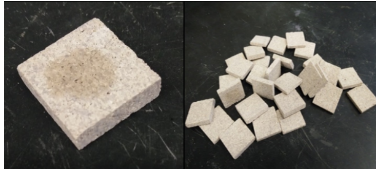
Figure 5. Indiana limestone (ILS) core sample slices are cleaned with methanol and toluene to remove possible existing salts, crude oil, and other deposits ( right ); core sample slices are in a hydrophilic (water-wet) state ( left ).
