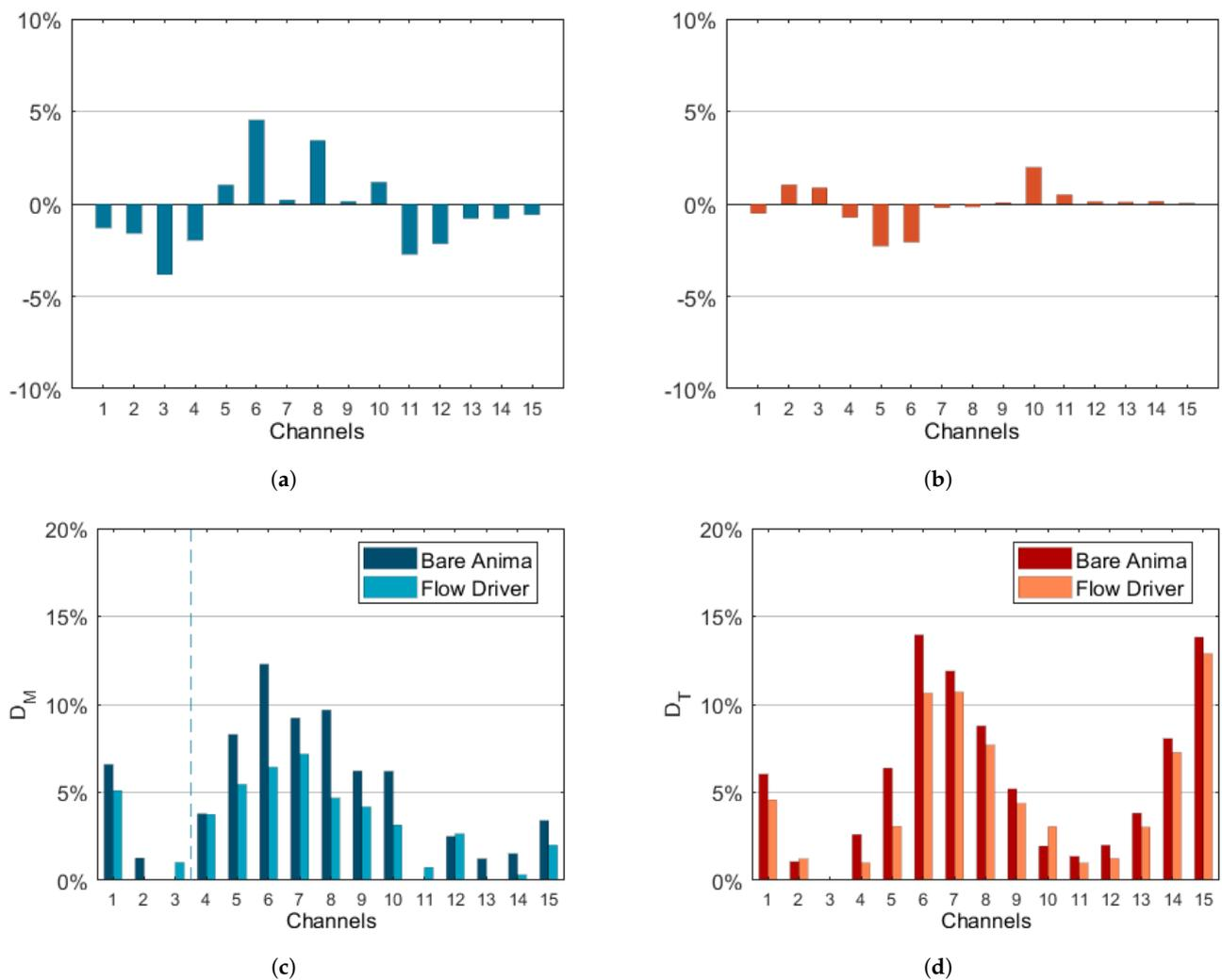
**Figure 9.** Deviation of coolant inlet conditions of flow driver configuration from reference case. (a) Percentual variation of coolant flow rates. (b) Percentual variation of inlet temperatures. (c) Coolant flow rate maldistribution. (d) Inlet temperature maldistribution.
