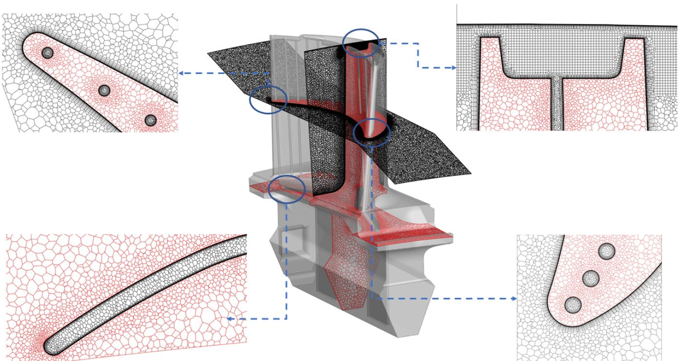
**Figure 4.** Flow mesh (black); solid mesh (red).
