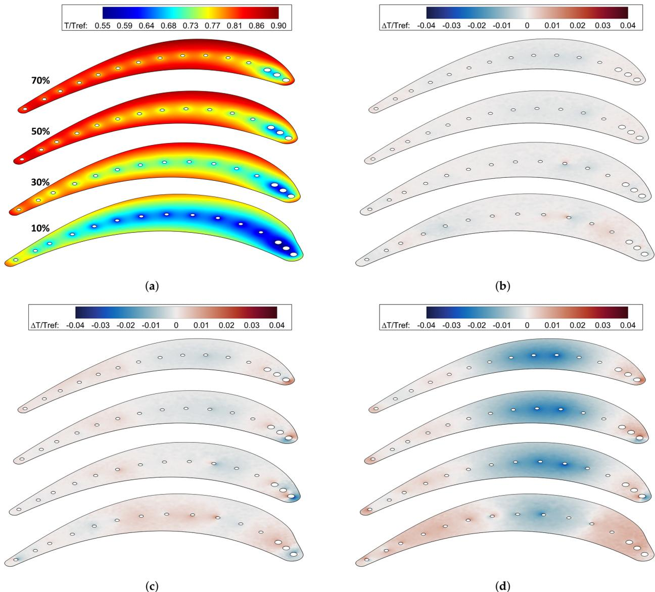
**Figure 13.** Variation of temperature profile—from bottom to top: 10%, 30%, 50%, and 70% of blade span. (a) Temperature profile on BA. (b) Temperature difference with VB. (c) Temperature difference with FD. (d) Temperature difference with DIFF.
