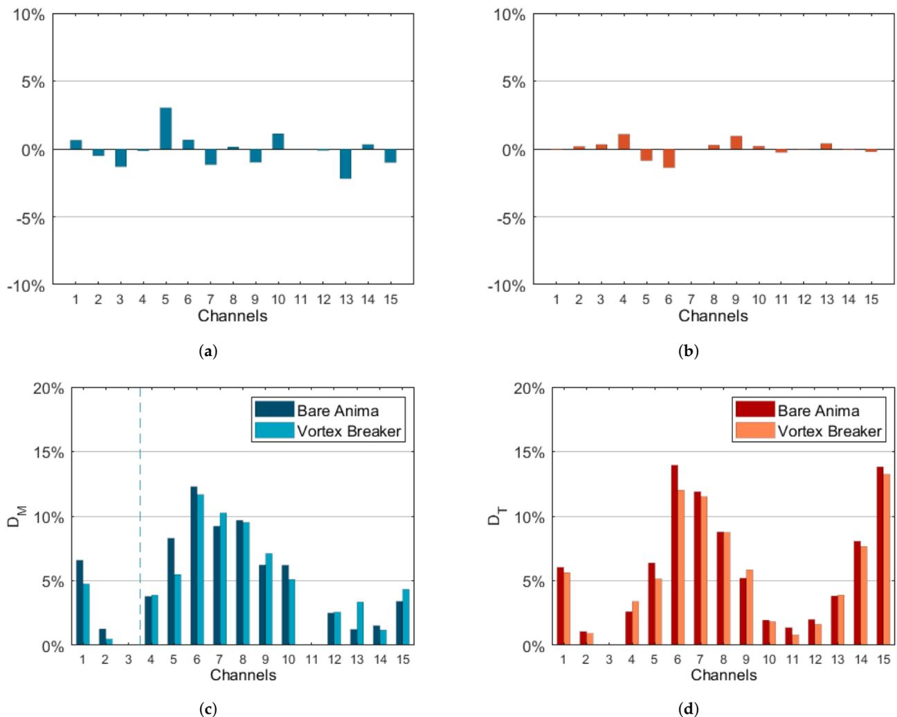
**Figure 8.** Deviation of coolant inlet conditions of vortex breaker configuration from reference case. (a) Percentual variation of coolant flow rates. (b) Percentual variation of inlet temperatures. (c) Coolant flow rate maldistribution. (d) Inlet temperature maldistribution.
