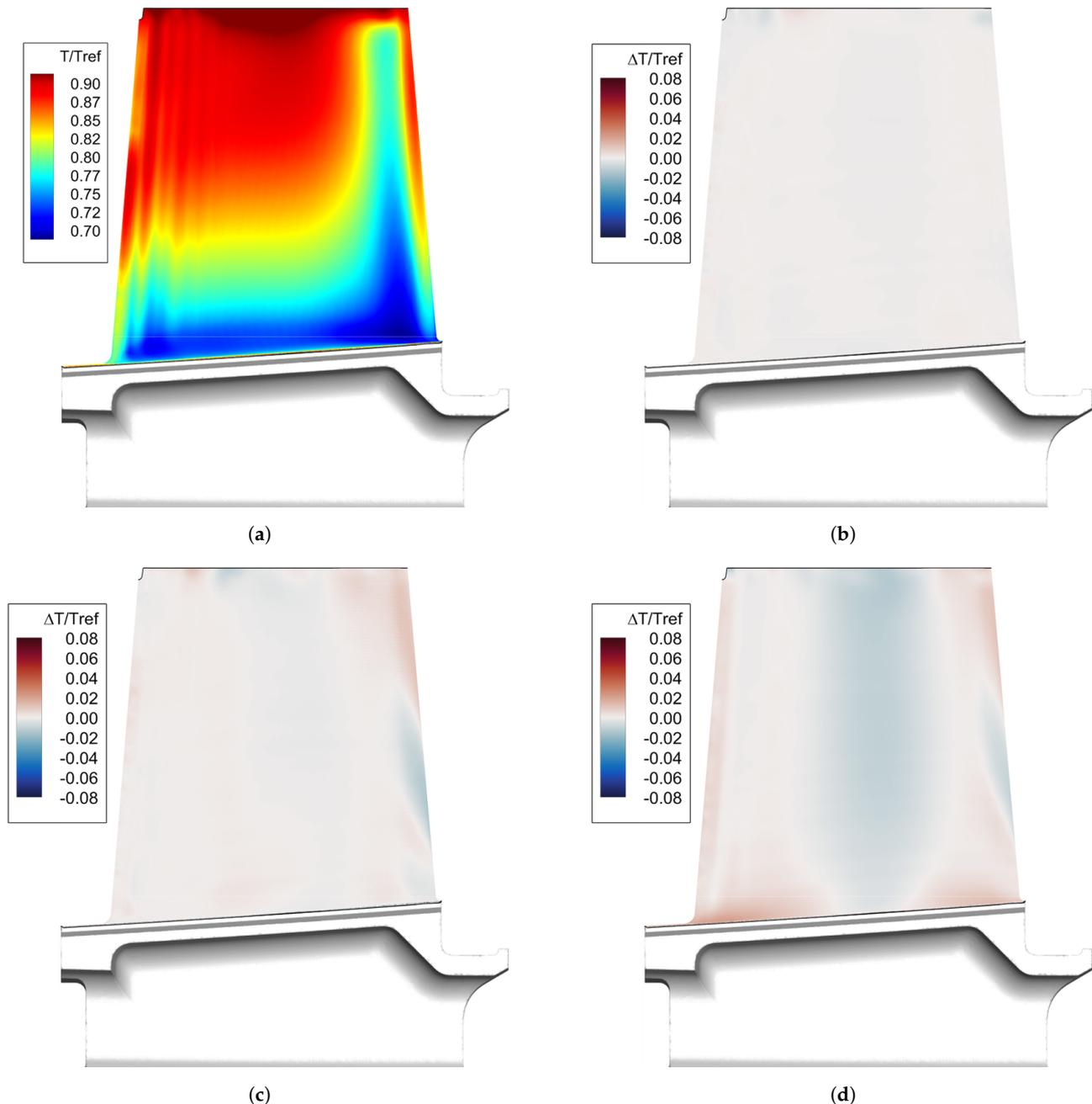
**Figure 11.** Variation of temperature profile—pressure side. (a) Temperature profile on BA. (b) Temperature difference with VB. (c) Temperature difference with FD. (d) Temperature difference with DIFF.
