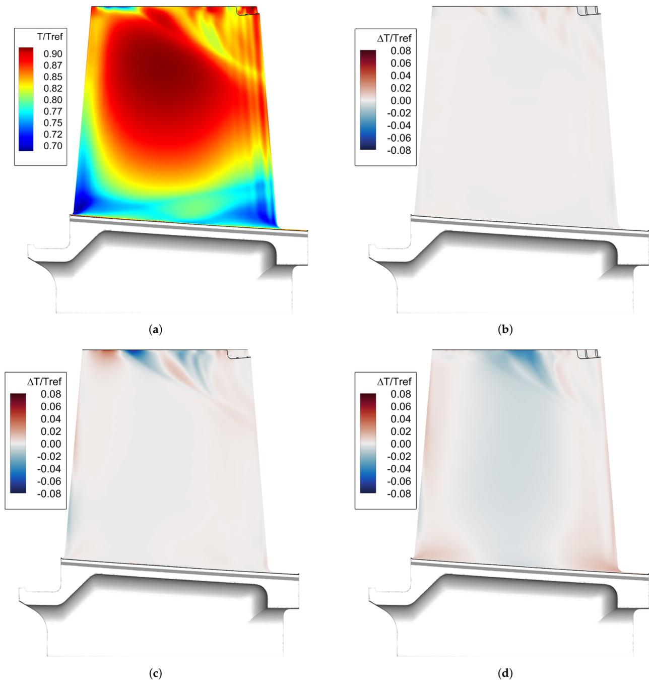
**Figure 12.** Variation of temperature profile—suction side. (a) Temperature profile on BA. (b) Temperature difference with VB. (c) Temperature difference with FD. (d) Temperature difference with DIFF.
