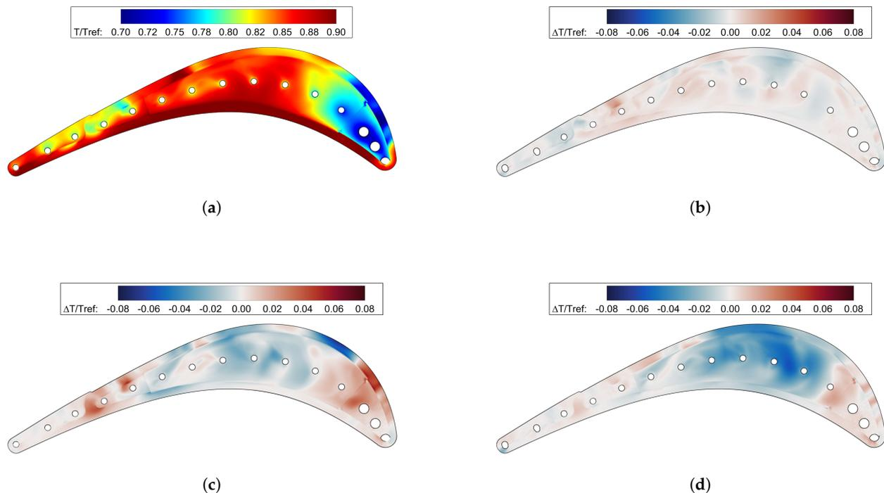
**Figure 15.** Temperature over blade tip. (a) Temperature profile on BA. (b) Temperature difference with VB. (c) Temperature difference with FD. (d) Temperature difference with DIFF.
