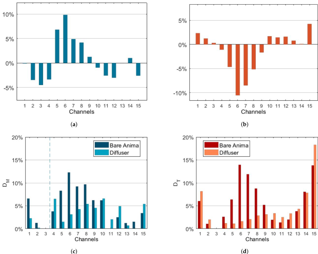
**Figure 10.** Deviation of coolant inlet conditions of diffuser configuration from reference case. (a) Percentual variation of coolant flow rates. (b) Percentual variation of inlet temperatures. (c) Coolant flow rate maldistribution. (d) Inlet temperature maldistribution.
