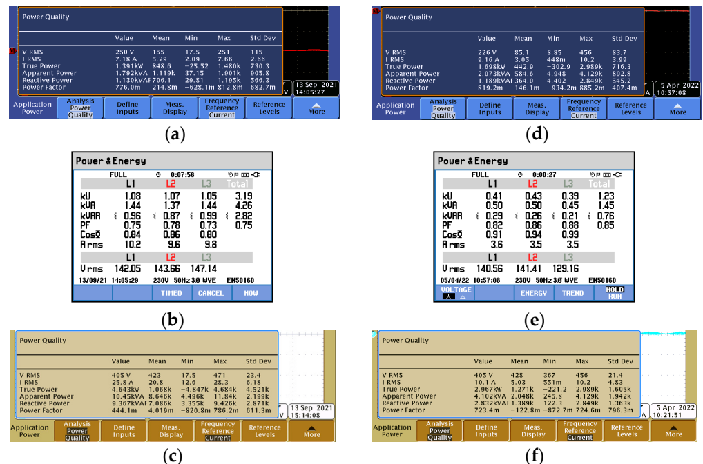
Figure 11. Dual-phase-inverter measured input and output powers: (a) measured single-phase output power; (b) measured output power delivered to the three-phase loads; (c) measured input power.
