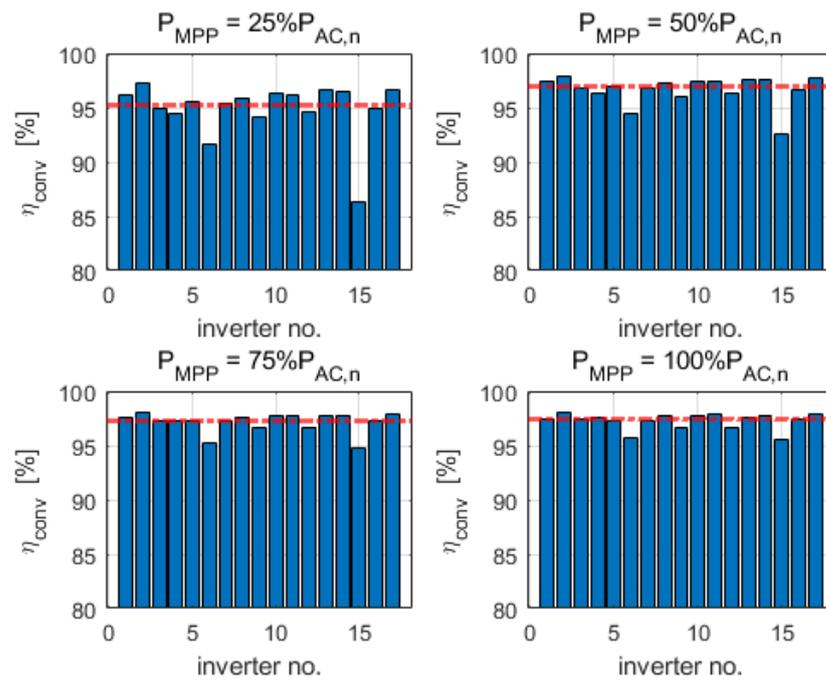
Figure A9. Conversion efficiencies of 3-phase PV inverters at  $U_{MPPT,max}$ .
