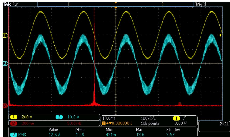
Figure 12. Example waveforms and the current spectrum of a 1-phase PV inverter.
