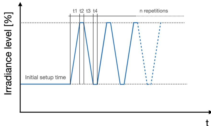
Figure 1. Test sequence for fluctuations of irradiation intensities.
