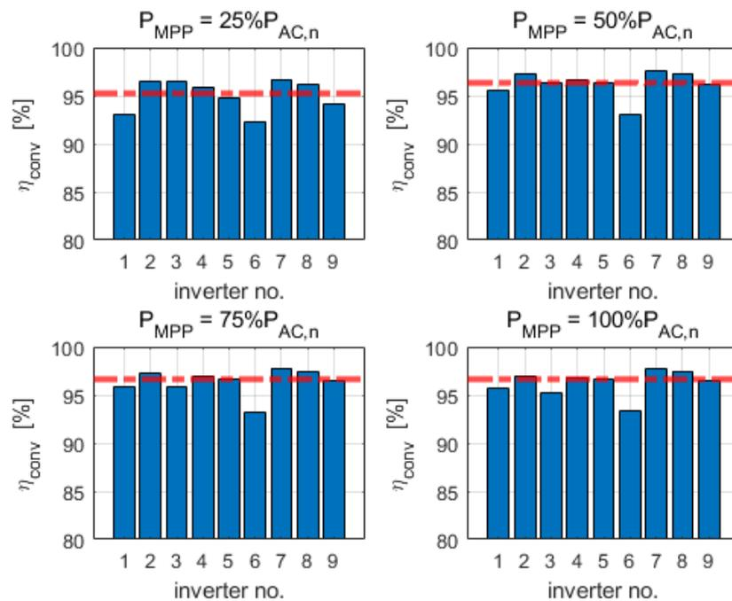
Figure A3. Conversion efficiencies of 1-phase PV inverters at  $U_{MPPT,max}$ .
