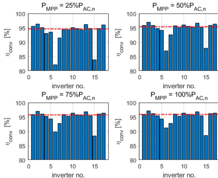
Figure A8. Conversion efficiencies of 3-phase PV inverters at  $U_{MPPT,min}$ .
