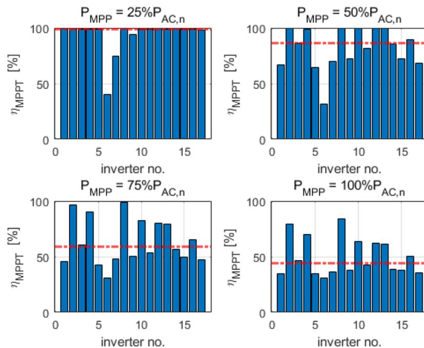
Figure A11. MPPT efficiencies of 3-phase PV inverters at  $U_{MPPT,min}$ .
