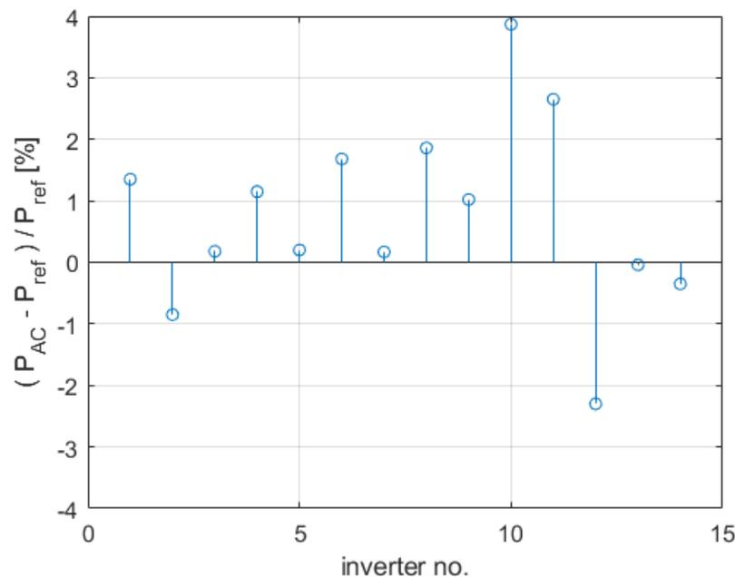
**Figure 7.** Comparison of power measured by the inverter ( $P_{AC}$ ) and reference power analyzer ( $P_{ref}$ ).
