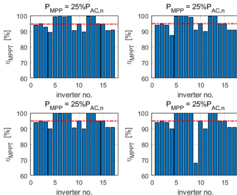
Figure A12. MPPT efficiencies of 3-phase PV inverters at  $U_{MPPT,max}$ .
