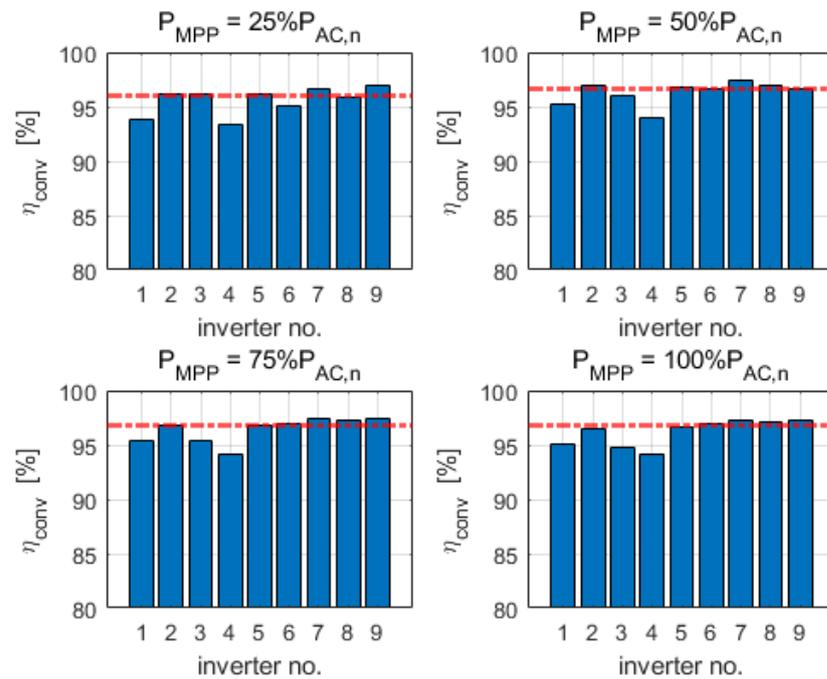
Figure A1. Conversion efficiencies of 1-phase PV inverters at  $U_{MPPT,n}$ .
