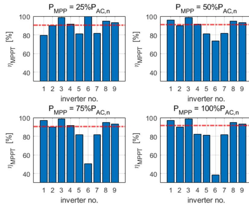
Figure A6. MPPT efficiencies of 1-phase PV inverters at  $U_{MPPT,max}$ .
