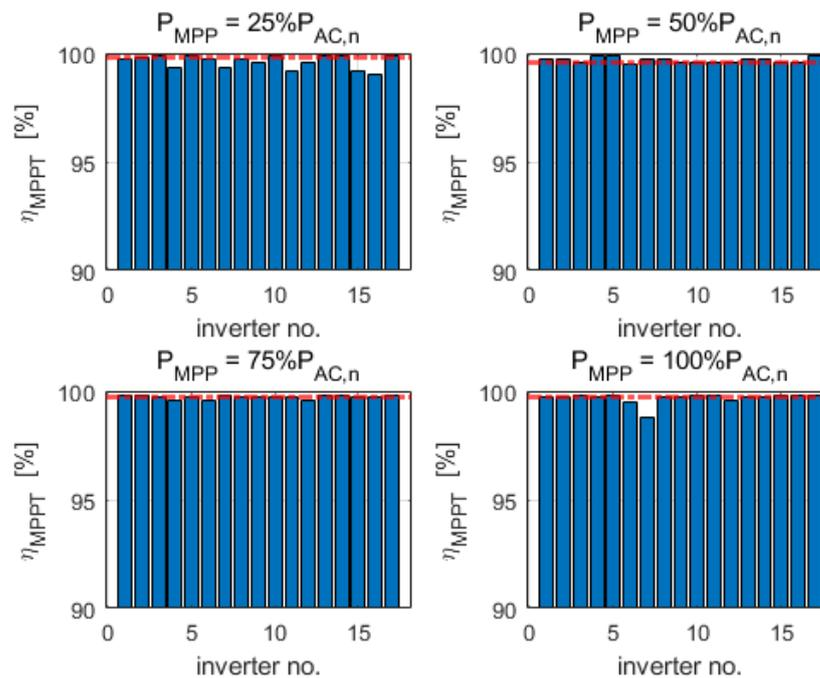
Figure A10. MPPT efficiencies of 3-phase PV inverters at  $U_{MPPT,n}$ .
