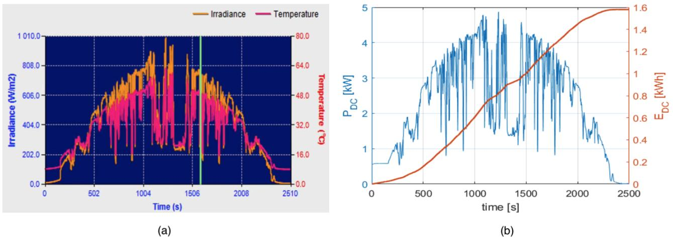
Figure 5. Dynamic MPPT testing procedure (a) and sample results of a tested inverter (b).
