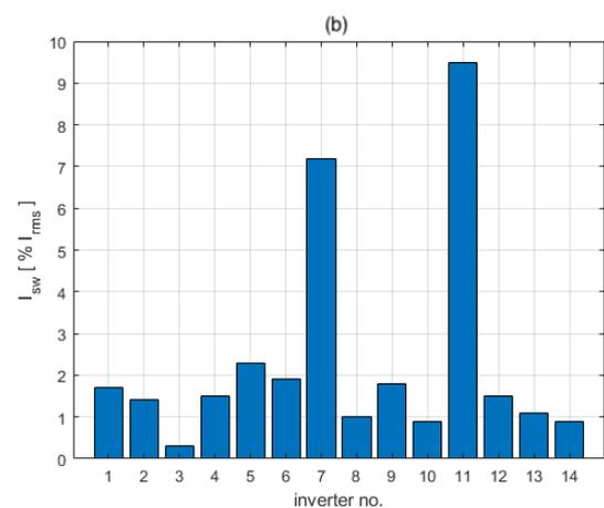
**Figure 11.** Switching frequency harmonic current emissions of the 1-phase (a) and 3-phase (b) PV inverters.
