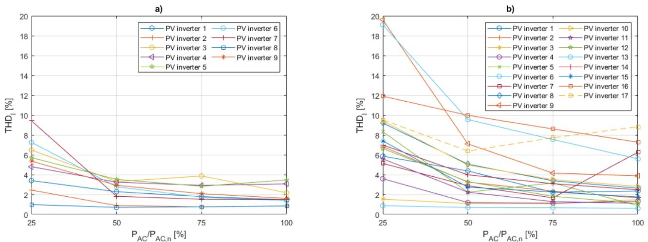
**Figure 10.**  $THD_i$  of the 1-phase (a) and 3-phase (b) PV inverters in relation to their active power generations.
