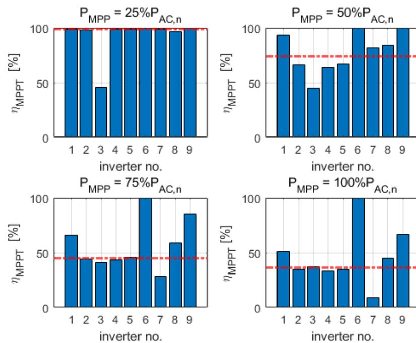
Figure A5. MPPT efficiencies of 1-phase PV inverters at  $U_{MPPT,min}$ .
