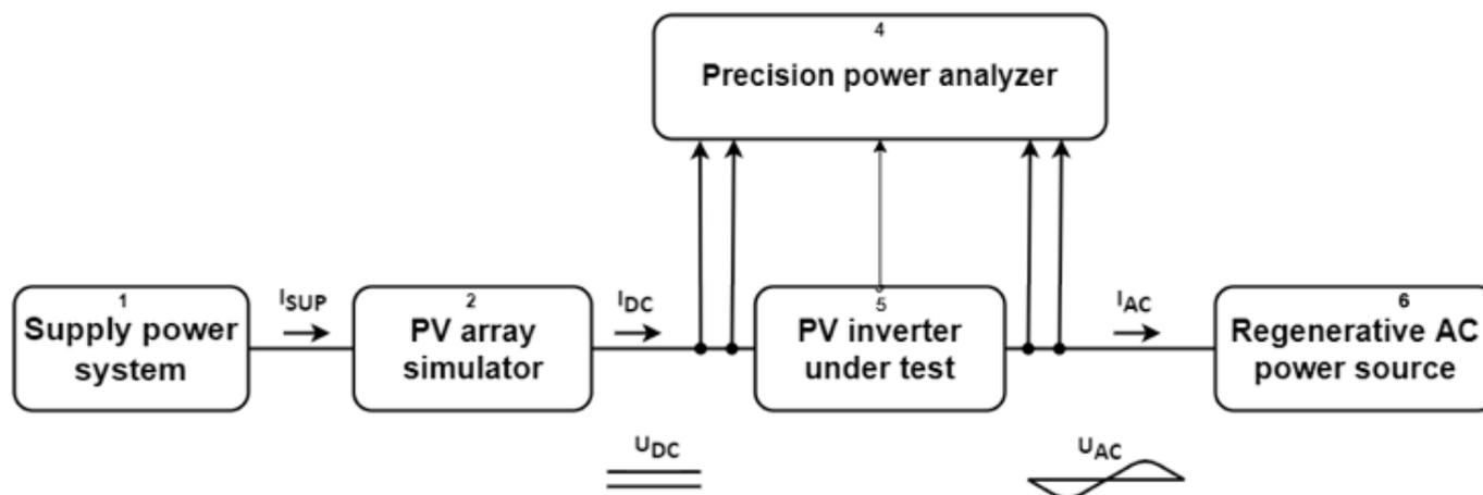
**Figure 2.** Block diagram of the laboratory stand for tests of PV inverters.
