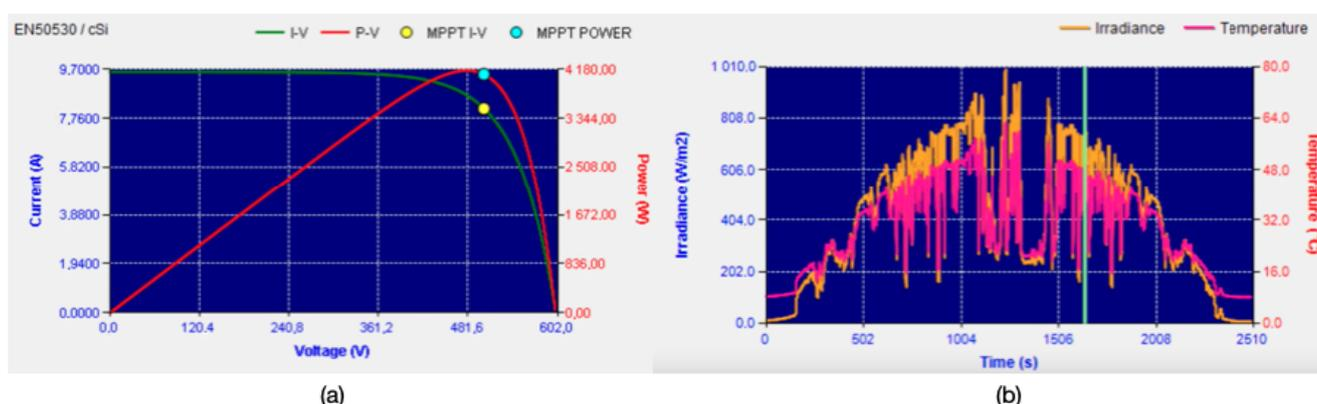
Figure 3. Exemplary current-voltage (a) and irradiance-time (b) characteristics from the PV simulator.
