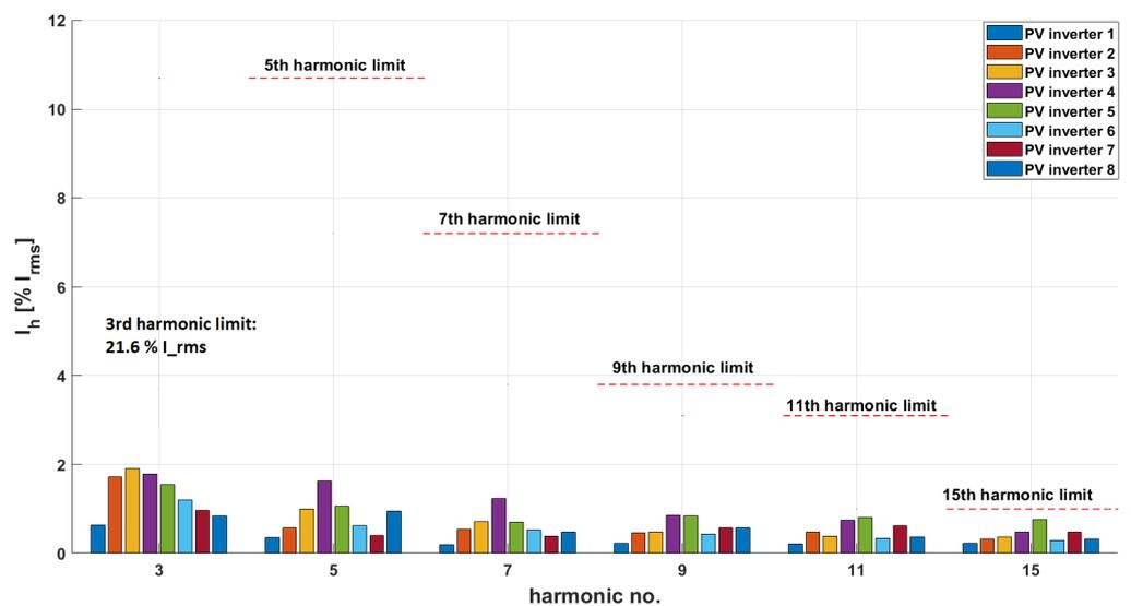
Figure 9. Harmonic current emissions of the tested 1-phase PV inverters.
