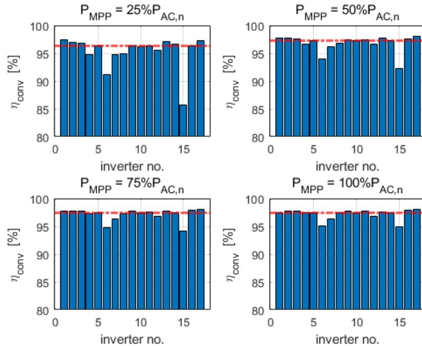
Figure A7. Conversion Efficiencies of 3-phase PV inverters at  $U_{MPPT,n}$ .
