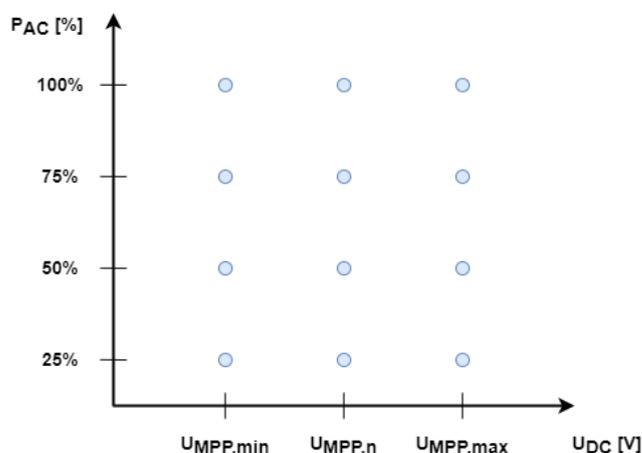
Figure 4. Graphical presentation of the operating point matrix of the tested PV inverters.
