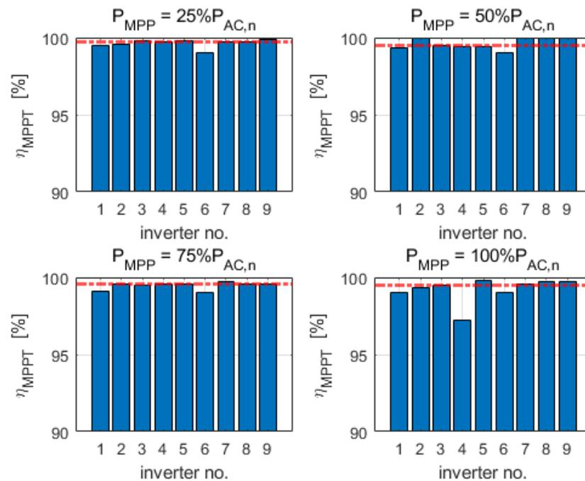
Figure A4. MPPT efficiencies of 1-phase PV inverters at  $U_{MPPT,n}$ .
