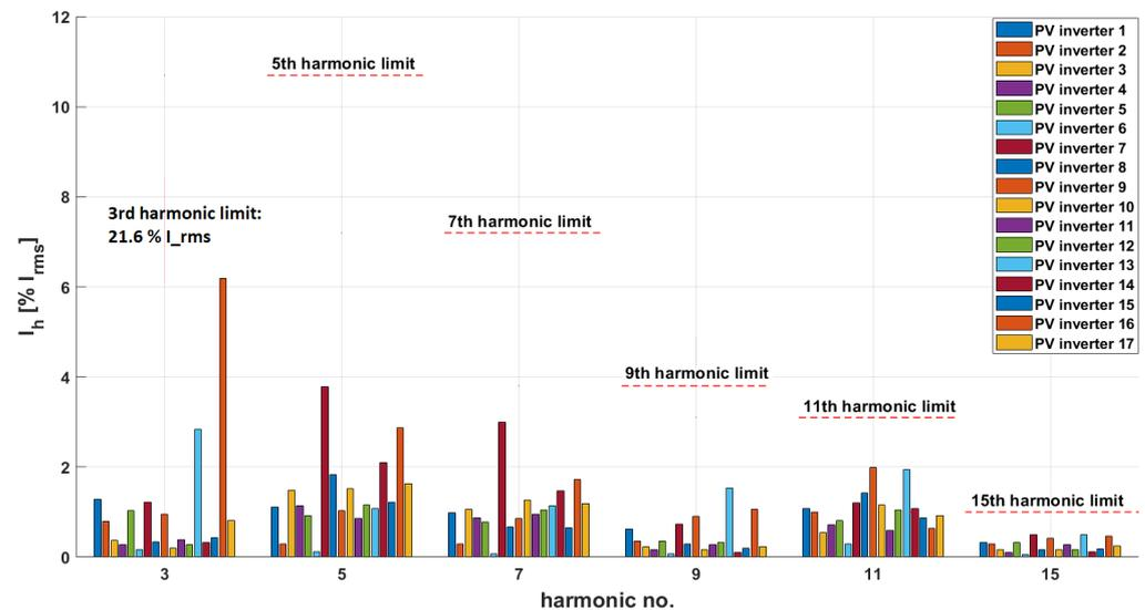
Figure 8. Harmonic current emissions of the tested 3-phase PV inverters.
