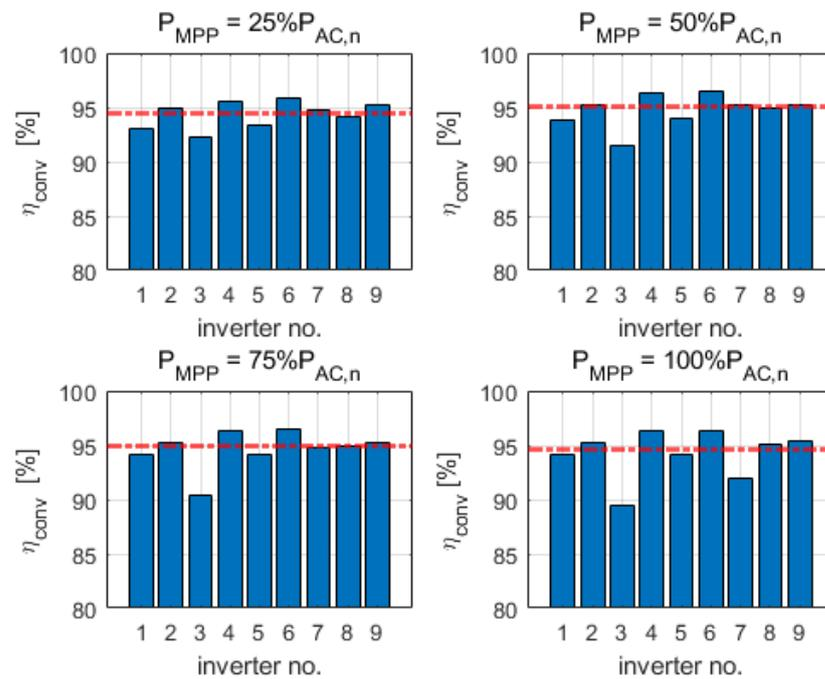
Figure A2. Conversion efficiencies of 1-phase PV inverters at  $U_{MPPT,min}$ .
