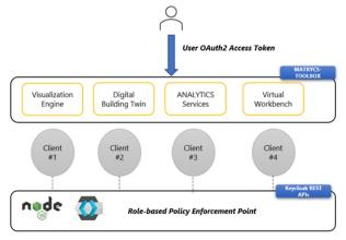
Figure 7. MATRYCS Toolbox integration with security layer.
