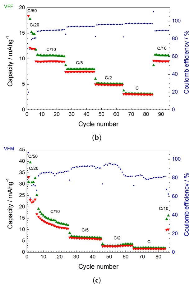
**Figure 5.** Cyclability and Coulombic efficiency of the studied cathode materials: FFF (a), VFF (b), and VFM (c). Charge (green “up” triangles) and discharge capacities (red “down” triangles) are compared to the Coulombic efficiency (blue dots) in consecutive cycles.
