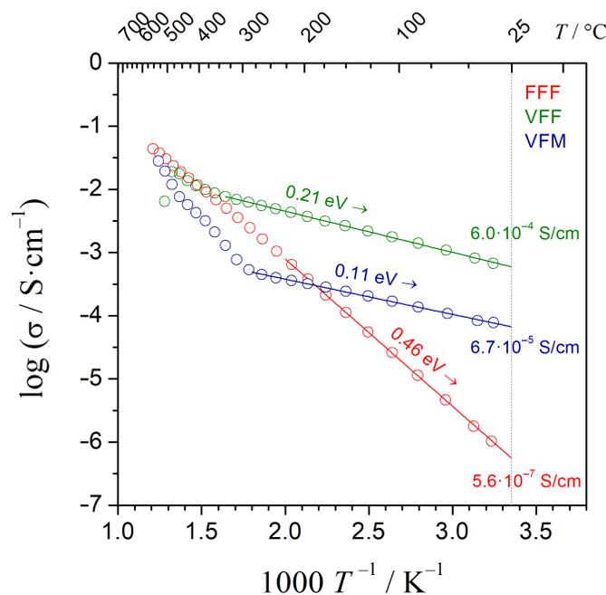
**Figure 2.** Electrical conductivity of nanocrystalline materials used for further cathode layer preparation. The values of the activation energy and conductivity at room temperature are given for each composition.
