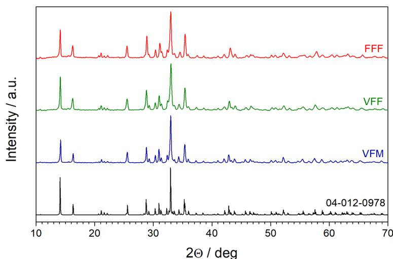
**Figure 1.** XRD patterns of nanocrystallized alluaudite-like glasses. A reference pattern of Na<sub>2</sub>Fe<sub>2</sub>Mn(PO<sub>4</sub>)<sub>3</sub> alluaudite (ICDD Card No. 04-012-0978) is given at the bottom.
