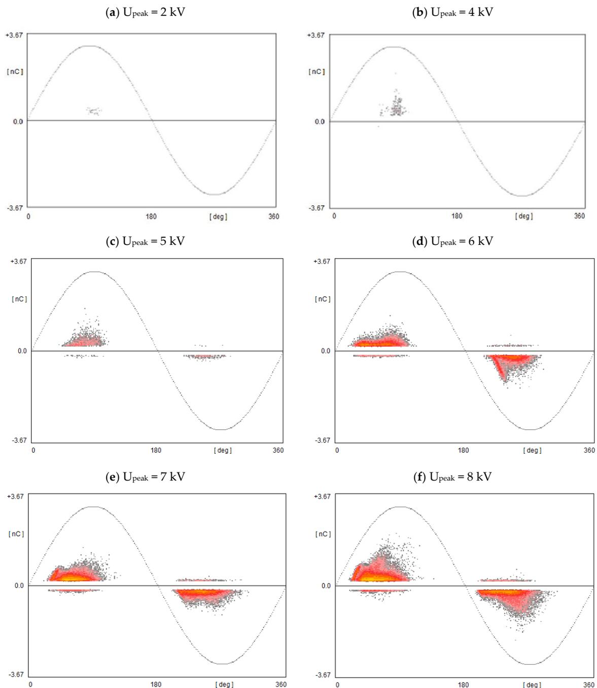
**Figure 4.** PRPD patterns at mixed DC 10 kV and additional 50 Hz AC content with a magnitude  $U_{peak}$ : (a) 2 kV, (b) 4 kV, (c) 5 kV, (d) 6 kV, (e) 7 kV, (f) 8 kV.
