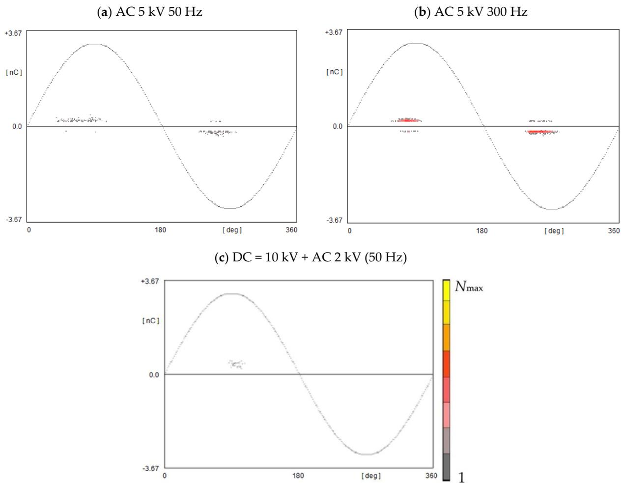
**Figure 3.** PRPD patterns acquired at inception voltage: (a) AC 50 Hz, (b) pure AC 300 Hz, (c) mixed DC 10 kV + AC 50 Hz 2 kV. (The scale for the number of pulses  $N$  presented on the right side of (c) is the same as for the other PRPD patterns presented in the article).
