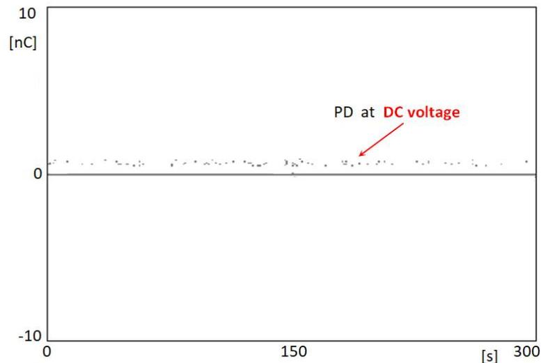
**Figure 5.** PD pattern at DC voltage (PD vs. time), at 10 kV; acquisition time 300 s.
