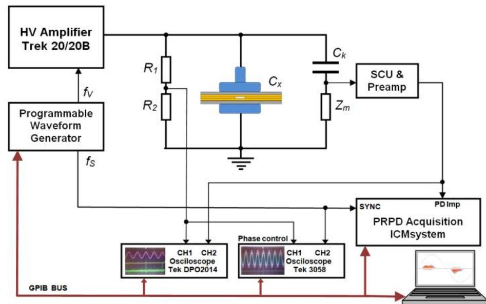
**Figure 2.** Measuring setup for PD measurements of DC voltage with superimposed harmonics:  $C_x$ —test object,  $Z_m$ —coupling impedance,  $C_k$ —coupling capacitor,  $R_1$ ,  $R_2$ —resistive divider, SCU—signal conditioning unit and preamplifier [29].
