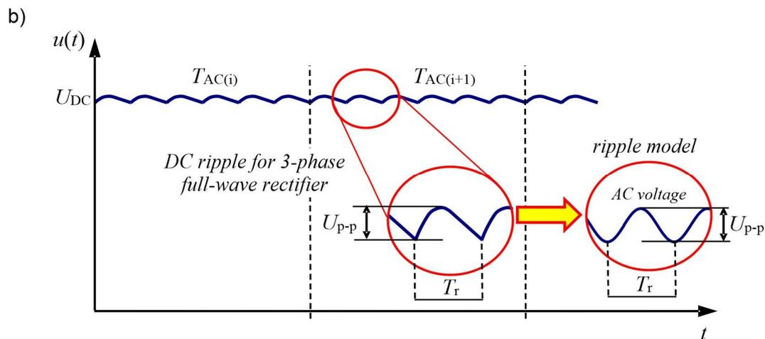
**Figure 1.** Measurement methodology and synchronization possibilities in HVDC networks for phase-resolved PD measurement: (a) concept and block diagram, (b) DC voltage with a single AC component as DC voltage with model ripple.
