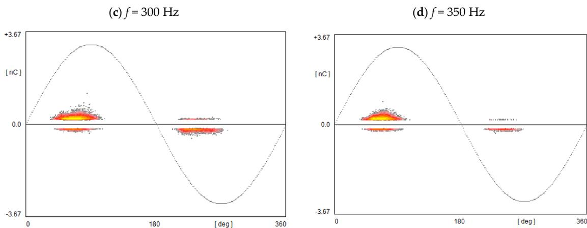
**Figure 6.** PRPD patterns at mixed DC 10 kV and AC 50 Hz  $U_{\text{peak}} = 6$  kV with frequency: (a) 50 Hz, (b) 150 Hz, (c) 300 Hz, (d) 350 Hz.
