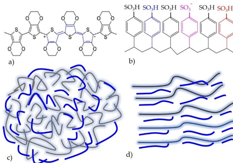
**Figure 3.** (a) Chemical structure of PEDOT; (b) chemical structure of PSS; (c) when PSS is added to PEDOT; a water dispersion solution is created; (d) when PEDOT:PSS is doped with conductive enhancers, a structural re-arrangement is formed, adapted from Ref. [42].
