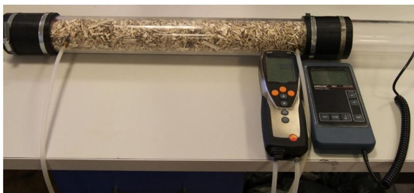
**Figure 3.** The apparatus for air permeability measurements filled with hemp shives.
