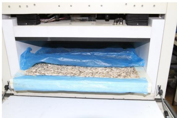
**Figure 2.** Heat flow meter—Fox 602 apparatus with hemp shives sample formed in the XPS frame.
