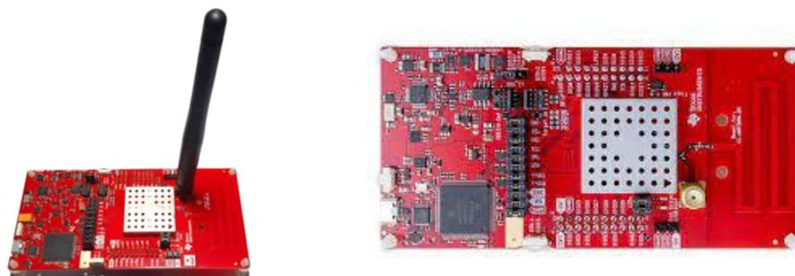
Figure 4. IEEE 802.15.4g Wi-SUN development board modelled LAUNCHXL-CC1352P.
