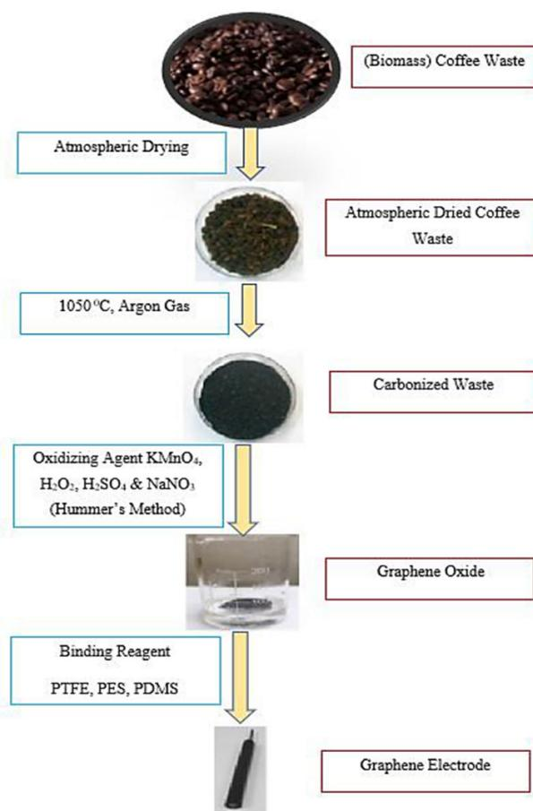
**Figure 2.** Schematic diagram of advanced Hummer's method for graphene oxide electrode.
