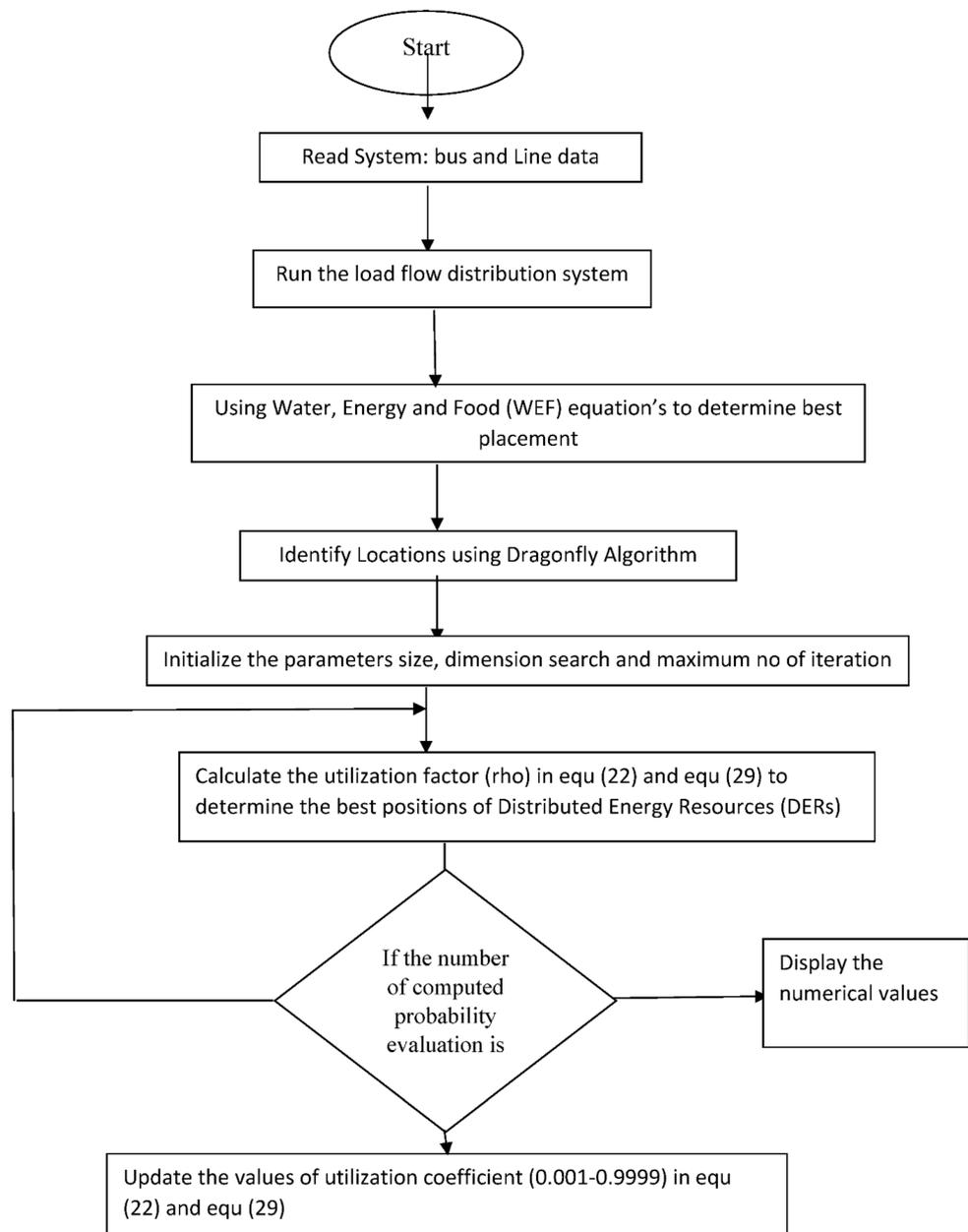
Figure 4. Optimal DG allocation methodology.
