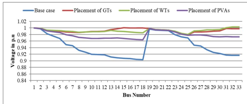
Figure 6. Voltage profile of 33 bus test system with optimal allocation of GTs, WT's, and PVAs placed in DS.
