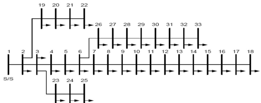
**Figure 2.** A case study of the 33-bus system under study [45].
