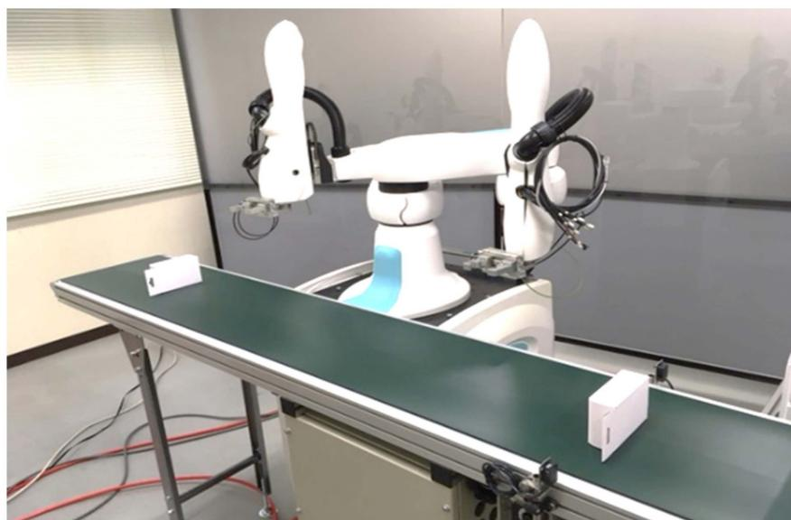
**Figure 9.** Experimental dual-arm robot system in pick-and-place operation.
