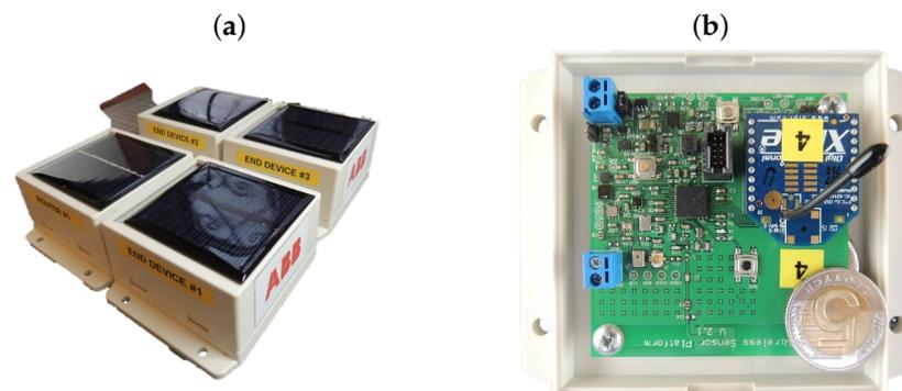
**Figure 2.** Picture of executive system devices—WSM, where (a) view with cover, (b) electronics' view.
