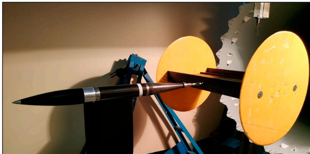
**Figure 4.** The sectional models on the strain-gauges balances.
