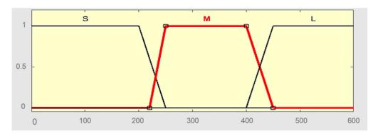
Figure 10. Membership functions of the latency variable for robust FLWADC.
