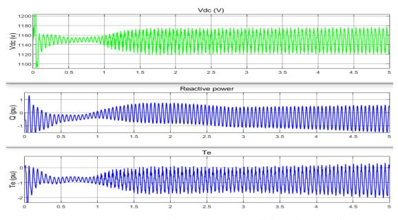
**Figure 14.** Capacitor voltage, reactive power, and electrical torque in k = 75%, v = 7 m/s with FLWADC. Ignored latency in time delay equal 500 ms.
