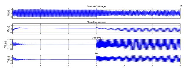
**Figure 8.** Capacitor voltage, reactive power stator voltage, and electrical torque in k = 25% to k = 75% & v = 7 m/s without damping.
