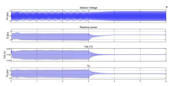
**Figure 9.** Damping of capacitor voltage, reactive power stator voltage, and electrical torque in k = 75% & v = 7 m/s with FLWADC (ignoring time delay).
