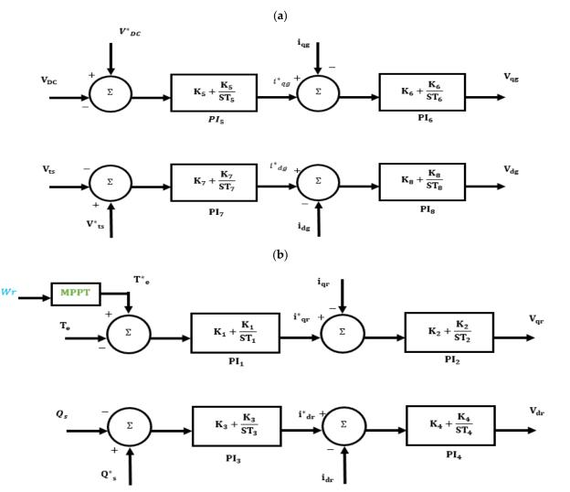
Figure 2. Controllers of the GSC (a) and RSC (b).
