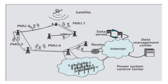
Figure 4. Hierarchical structure of a Wide Area Measurement System with PMUs.
