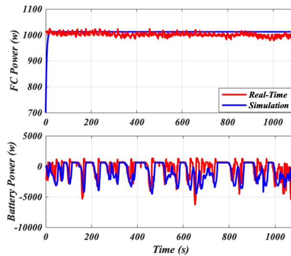
Figure 13. Real-time results of the PEMFC power and the battery power.
