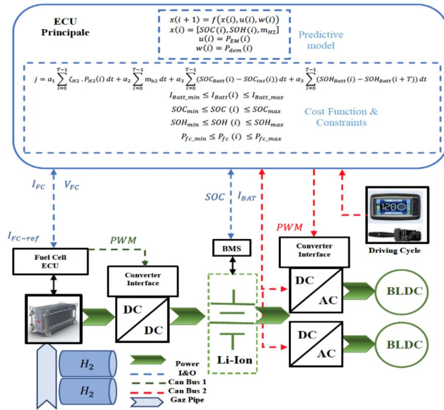
Figure 1. Synoptic diagram of the Moby Post vehicle.
