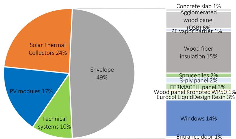
**Figure 7.** Life cycle assessment of the SolAce unit showing breakdown of different components’ contributions to embodied energy use as well as CO<sub>2</sub> emissions.
