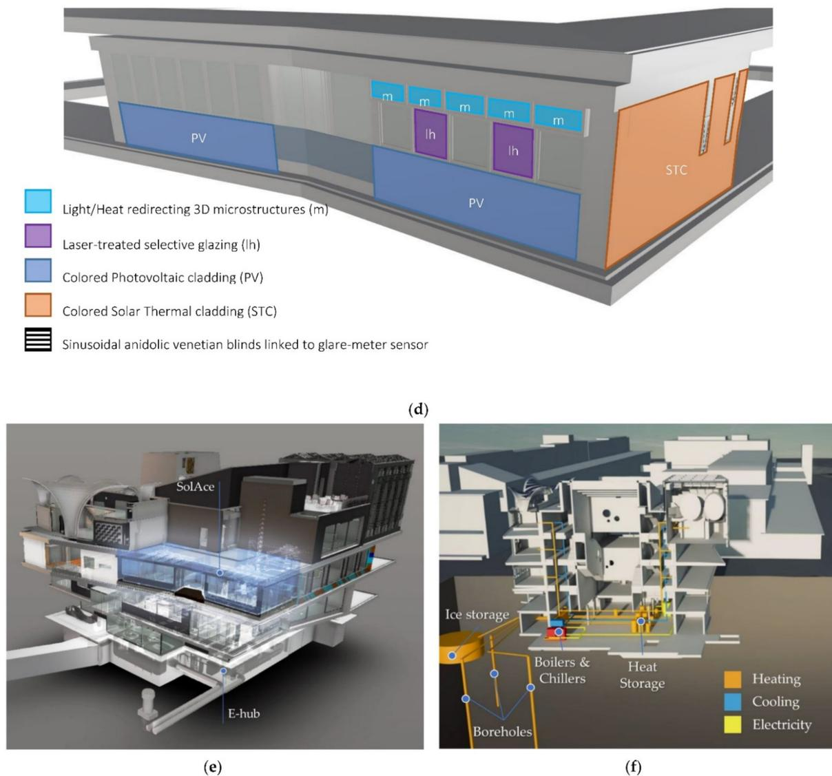
**Figure 2.** Plan (a), outdoor view (b), multifunctional façade representation (c), overview context map (d), and context model (e,f) of the NEST SolAce unit and the Energy-hub (plan—courtesy of Lutz Architectes, photo—Roman Keller©, context map—Google Earth©, context model of the NEST—Autodesk research©, and context model of the E-Hub—EMPA©).
