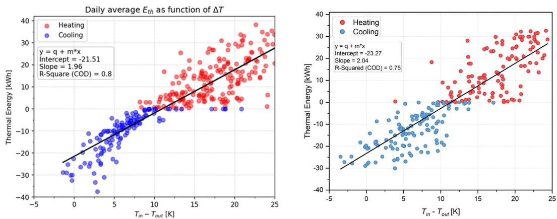
**Figure 10.** Daily heating and cooling demands as a function of average daily temperature difference for simulated (left) and monitored data (right).
