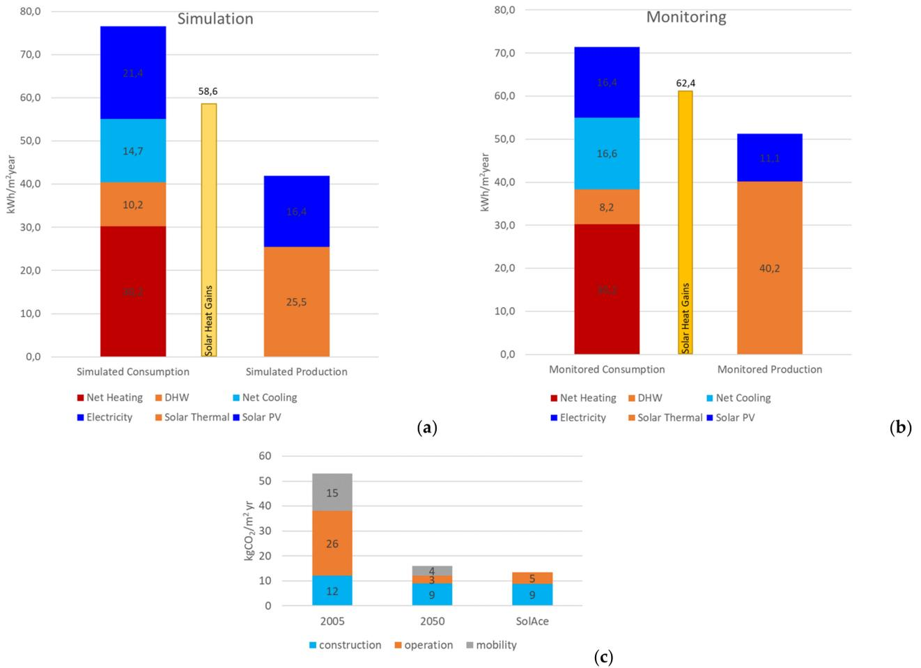
**Figure 6.** Bar chart of the annual end energy consumption vs the production and simulation scenario (a) and data-driven scenario (b). ‘Passive solar gains’ are annual and shown only for comparison; CO<sub>2</sub> emissions of the Swiss average buildings in 2005, 2050, and for the SolAce unit (c).
