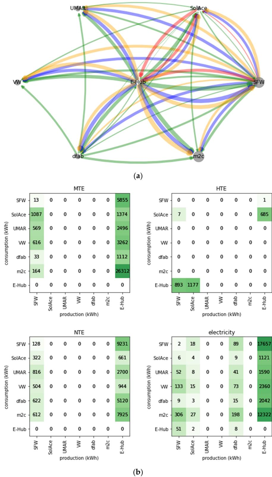
**Figure 9.** Energy exchange diagram between units at NEST (a) and relative association matrixes (b). In the diagram, flow thickness is proportional to the logarithm of the energy amount, while the node size is proportional to the annual total energy demand of the node.
