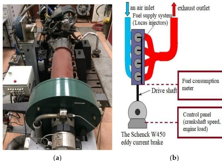
**Figure 1.** The research stand: XUD9A engine (a) and scheme of research stand (b).
