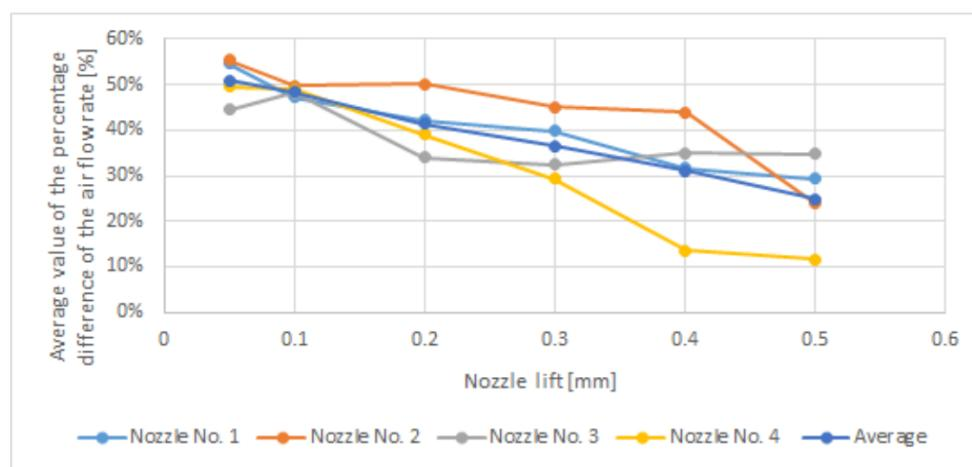
**Figure 4.** The mean value of the airflow rate for diesel fuel.
