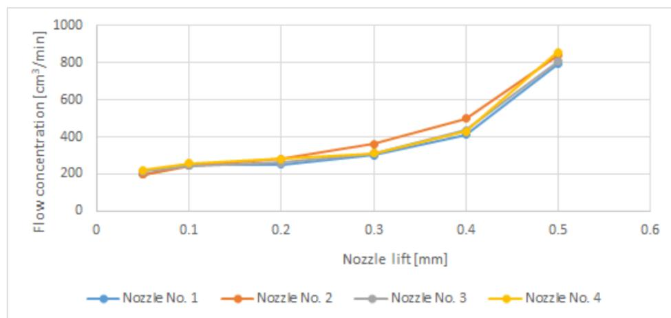
**Figure 2.** The flow before the test for diesel fuel.
