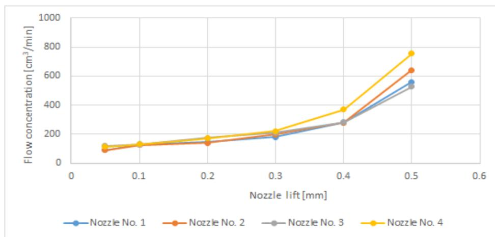
**Figure 3.** The flow after the test for diesel fuel.
