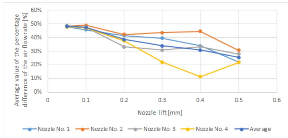
Figure 7. The mean value of the airflow rate for SD1.
