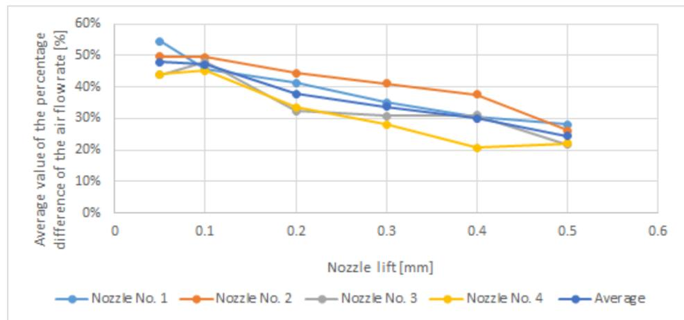
Figure 10. The mean value of the airflow rate for SD2.
