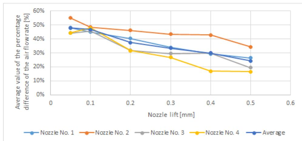
Figure 13. The mean value of the airflow rate for SD3.
