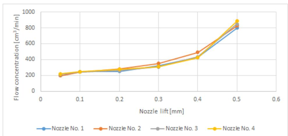
Figure 5. The flow before the test for SD1.
