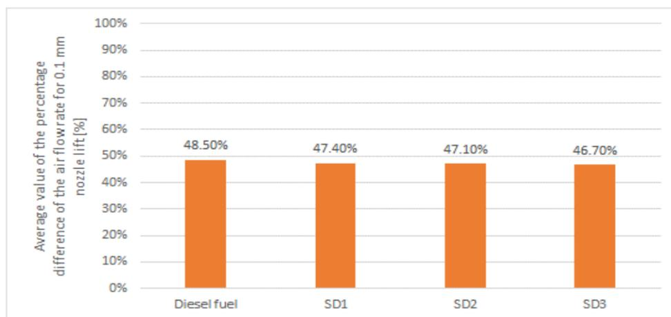
**Figure 15.** The mean value of the airflow rate difference (expressed as a percentage) for a 0.1 mm nozzle lift in the CEC test PF-023.
