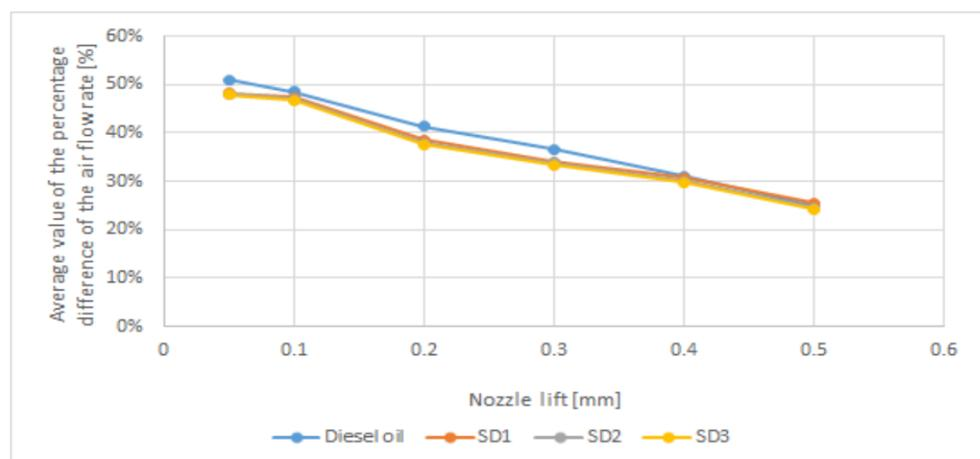
Figure 14. The mean value of the difference in the airflow rate through the injectors obtained from the CEC test PF-023.
